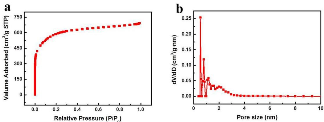
**Fig. S5** (a) Nitrogen adsorption-desorption isotherm and (b) pore-size distribution of NHVO.
