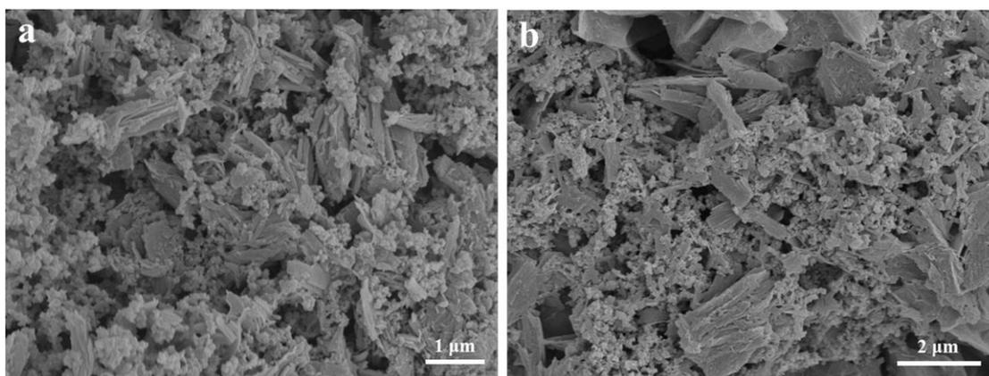
**Fig. S9** (a, b) SEM images of NHVO/rGO composite after 100 cycles in 500 mg/L NaCl solution at the cell voltage of 0.8 V.
