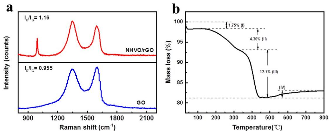
**Fig. S3** (a) Raman spectra of NHVO/rGO composite and pure GO; (b) TGA curve of NHVO/rGO composite.
