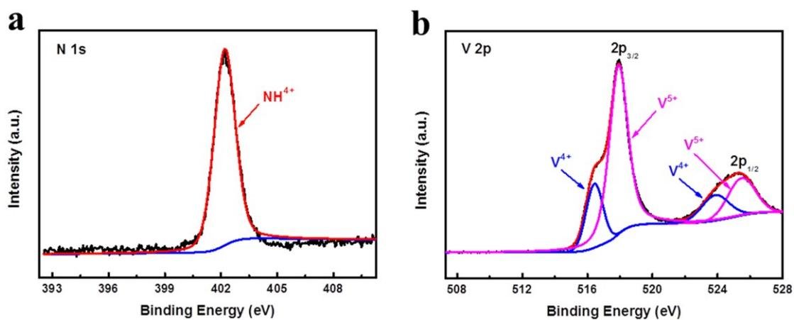
**Fig. S4** (a) N 1s and (b) V 2p XPS spectrum of NHVO.
