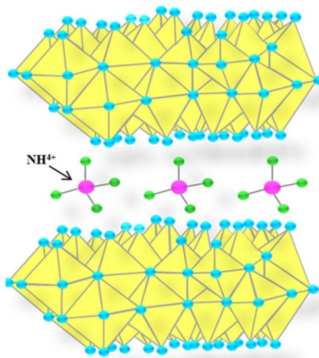
**Fig. S1** Crystal structure diagram of  $\text{NH}_4\text{V}_4\text{O}_{10}$ .
