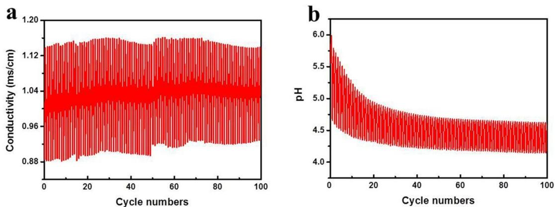
**Fig. S8** (a) the effluent conductivity variation and (b) effluent pH changes of NHVO/rGO cell during 100 cycles of charging and discharging process in 500 mg/L NaCl solution at the cell voltage of 0.8 V.
