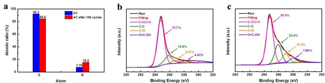
**Fig. S10** (a) atomic ratio of C and O on the surface of AC after 100 cycles; (b) C 1s XPS spectrum of AC before cycling; (c) C 1s XPS spectrum of AC after 100 cycles.
