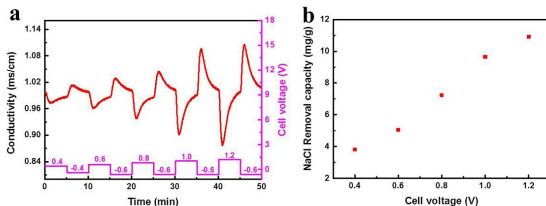
**Fig. S6** (a) conductivity change curves of effluent and (b) NaCl removal capacity of rGO//AC cell (rGO as the cathode and AC as the anode) in 500 mg/L NaCl solution at different cell voltages. (The mass of active material (containing AC and rGO) is 45.0 mg. The thickness of AC electrode, and rGO electrode is about 255.2  $\mu$ m and 326.1  $\mu$ m, respectively.)
