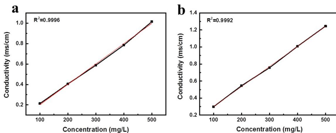
**Fig. S7** (a) relationship between conductivity and concentration of CaCl<sub>2</sub>; (b) relationship between conductivity and concentration of MgCl<sub>2</sub>
