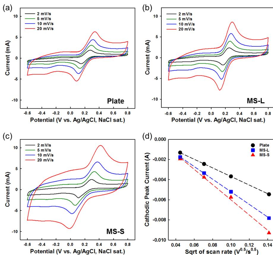
**Fig. S2** Cyclic voltammogram of (a) plate, (b) MS-L, and (c) MS-S in 0.01 M  $\text{K}_4\text{Fe}(\text{CN})_6$  and 100 mM KCl supporting electrolyte. (d) Cathodic peak currents were plotted with respect to the square root of the scan rate. The absolute gradients of the cathodic peak currents and scan rates are 0.0428, 0.0628 and 0.0758  $\text{A V}^{-0.5} \text{s}^{0.5}$ , respectively, for plate, MS-L and MS-S electrodes.
