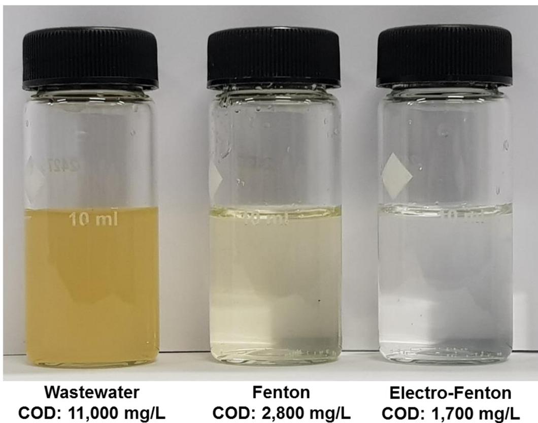
**Fig. S5** Color and COD changes of real wastewater treated with the Fenton or electro-Fenton processes.
