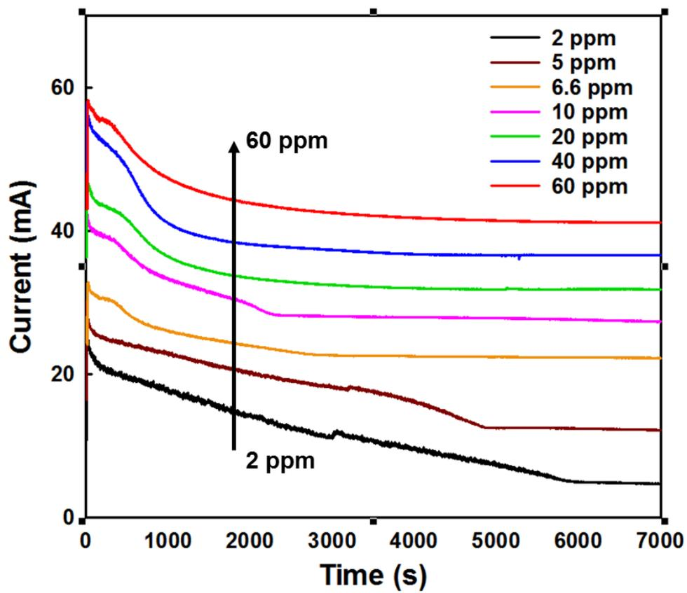
Fig. S3 Current profiles with respect to change in the Fe<sup>2+</sup> concentration
