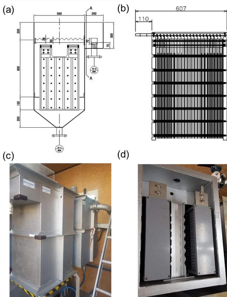
**Fig. S6** Schematics and photographs of (a, c) pilot-scale electro-Fenton and corresponding (b, d) electrode stacks.
