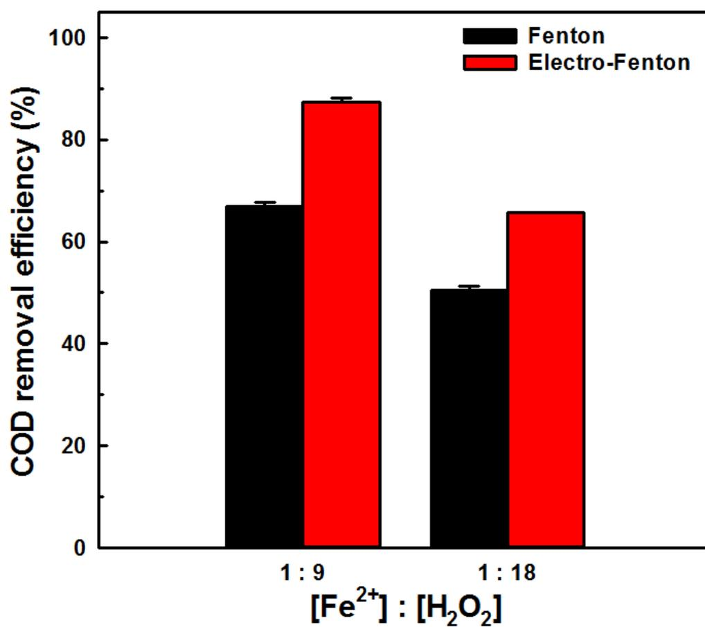
**Fig. S4** Change in COD removal efficiency of the Fenton and electro-Fenton processes with respect to injected concentration ratio of  $\text{Fe}^{2+}$  and  $\text{H}_2\text{O}_2$ .
