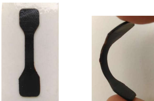
Figure S1. Pictures of dog bone-shaped samples of vitrimer 1.
