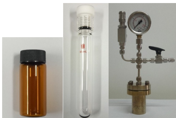
Figure S1 The three types of reactors employed in the work. The brown bottle (left), the thick-wall bottle (middle) and the autoclave (right).
