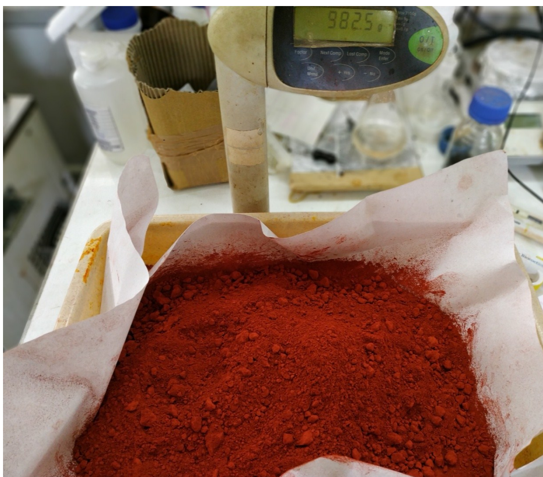
Figure- S2: 1 kg Sudan dye synthesized using the screw reactor
