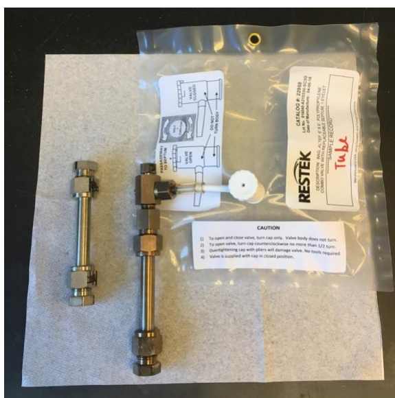
Figure S1. Photo of tube reactors used for depolymerization (left) and dehydration and decarboxylation reactions (right). The latter was attached to a gas sampling bag via a small piece of plastic tube.
