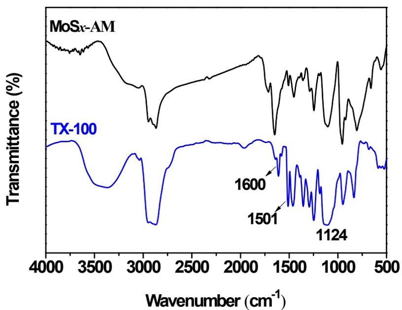
**Figure S2.** FTIR spectra of MoS<sub>x</sub>-AM and Triton X-100.
