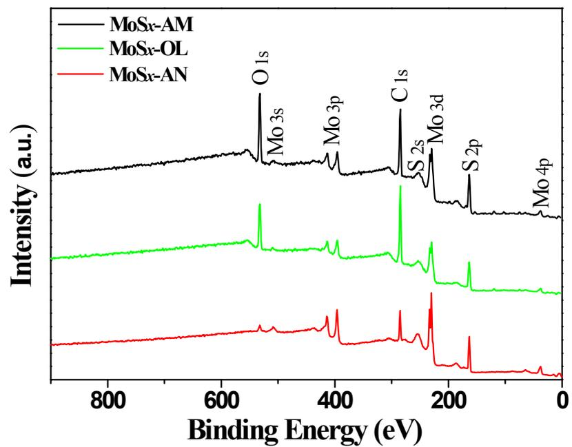
Figure S3. XPS survey spectra of MoS<sub>x</sub> nanocatalysts samples.
