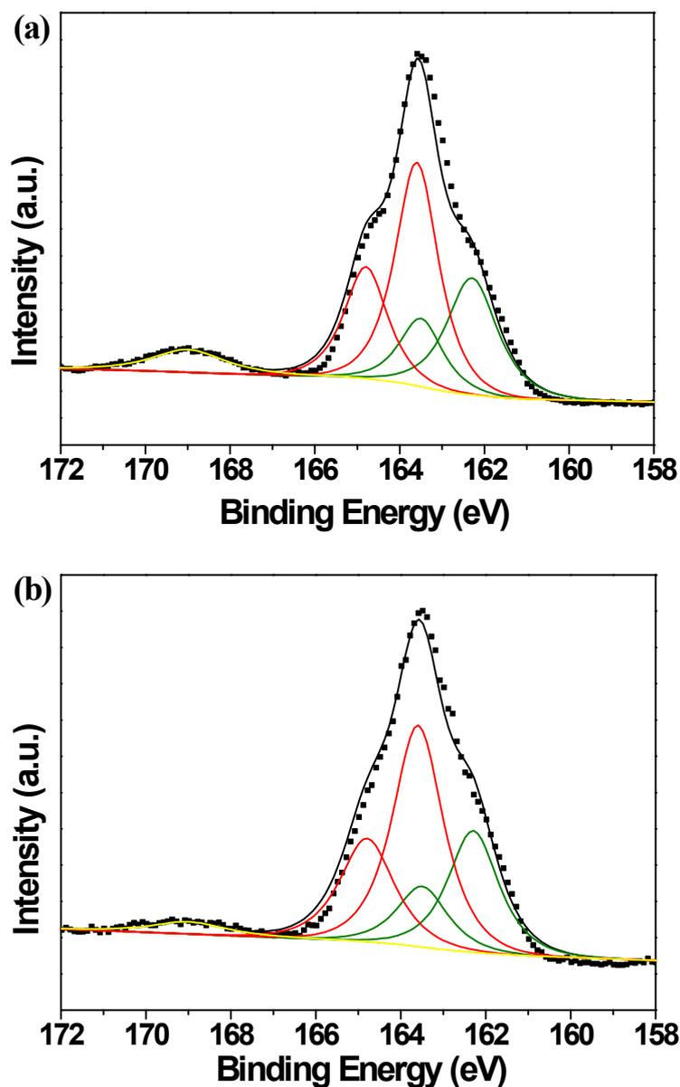
**Figure S5.** High-resolution S 2p spectra of (a) MoS<sub>x</sub>-AM and (b) MoS<sub>x</sub>-OL. (Dashed lines are raw data, black lines are fitted data, olive lines are S 2p<sub>3/2</sub> and S 2p<sub>1/2</sub> orbital curves of unsaturated S<sup>2-</sup> and terminal S<sub>2</sub><sup>2-</sup>, red lines are S 2p<sub>3/2</sub> and S 2p<sub>1/2</sub> orbital curves of apical S<sup>2-</sup> and bridging S<sub>2</sub><sup>2-</sup>, yellow lines are orbital curves of S<sup>6+</sup>.)
