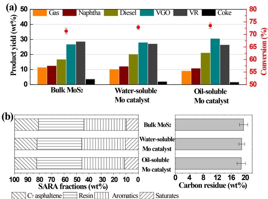
**Figure S6.** (a) Product distribution and conversion, and (b) SARA composition and Conradson carbon residue of VR products from SZVR slurry-phase hydrocracking with different Mo-based catalysts.
