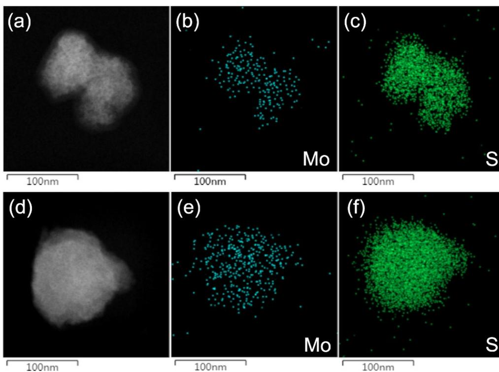
**Figure S1.** TEM image and the corresponding elemental mapping images of Mo, S of (a-c) MoS<sub>x</sub>-AM and (d-f) MoS<sub>x</sub>-OL.
