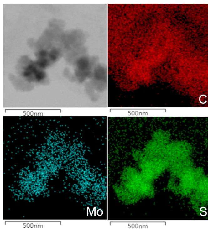
**Figure S9.** TEM image and the corresponding EDS elemental mapping images of C, Mo, S of the solid products from SZVR slurry-phase hydrocracking with MoS<sub>x</sub>-OL.
