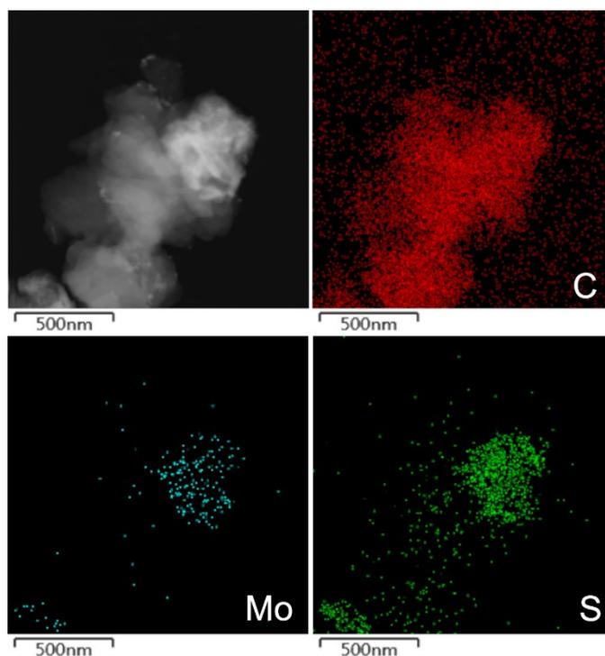
**Figure S10.** TEM image and the corresponding EDS elemental mapping images of C, Mo, S of the solid products from SZVR slurry-phase hydrocracking with MoS<sub>x</sub>-AN.
