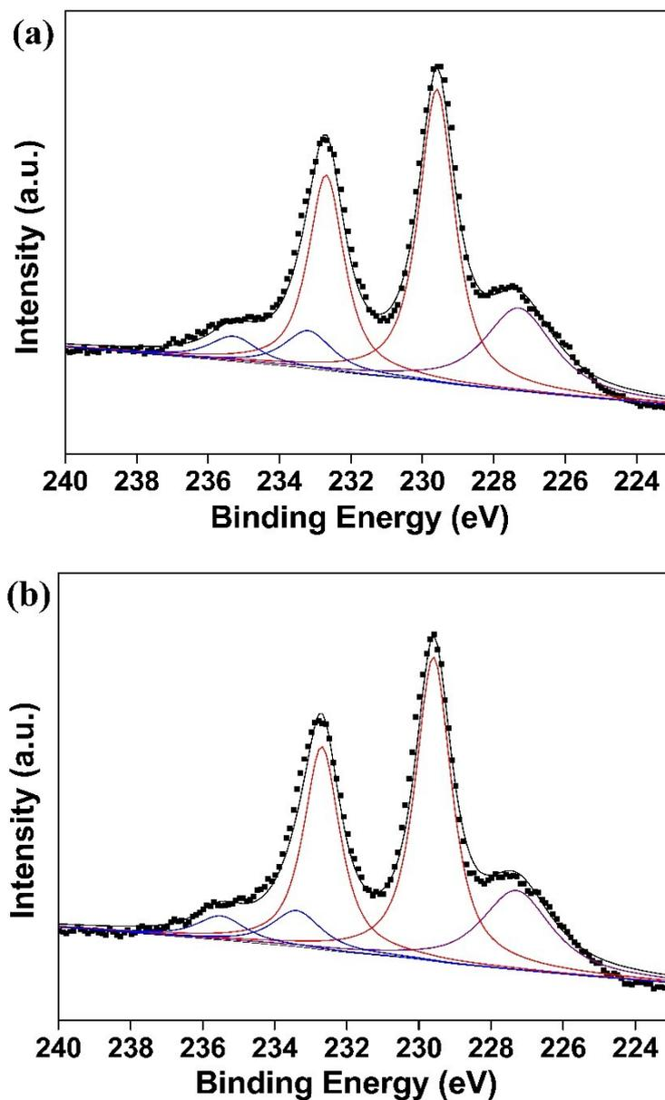
**Figure S4.** High-resolution Mo 3d spectra of (a) MoS<sub>x</sub>-AM and (b) MoS<sub>x</sub>-OL. (Dashed lines are raw data, black lines are fitted data, red lines are 3d<sub>5/2</sub> and 3d<sub>3/2</sub> orbital curves of Mo<sup>4+</sup>, blue lines are 3d<sub>5/2</sub> and 3d<sub>3/2</sub> orbital curves of Mo<sup>6+</sup>, purple lines are orbital curves of S 2s.)
