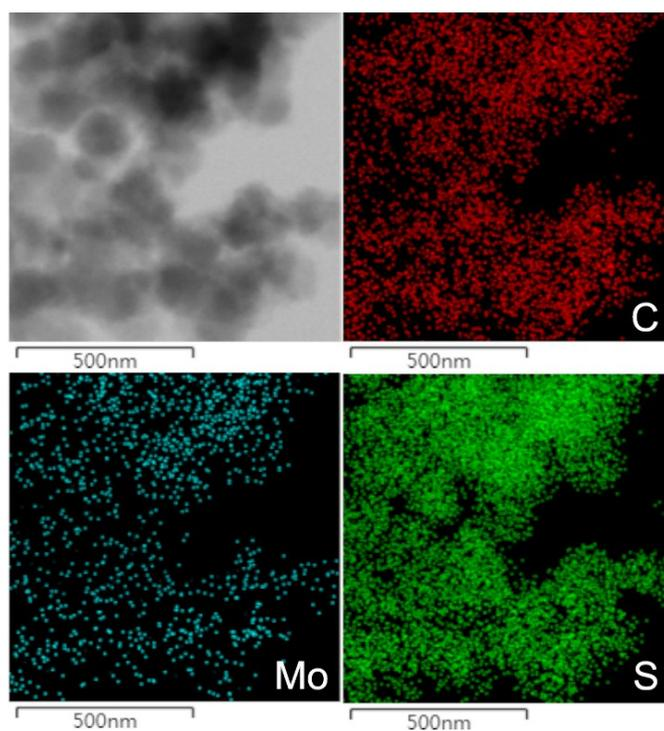
**Figure S8.** TEM image and the corresponding EDS elemental mapping images of C, Mo, S of the solid products from SZVR slurry-phase hydrocracking with MoS<sub>x</sub>-AM.
