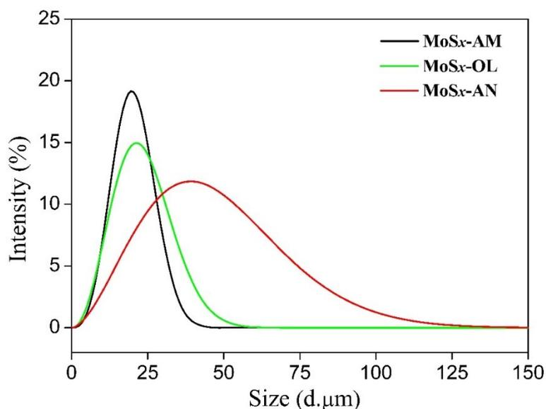
**Figure S7.** Size distribution of the coke products from SZVR slurry-phase hydrocracking with different MoS<sub>x</sub> nanocatalysts.
