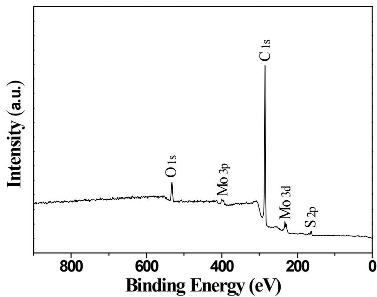
**Figure S11.** XPS survey spectra of the coke product from SZVR slurry-phase hydrocracking with MoS<sub>x</sub>-AM.
