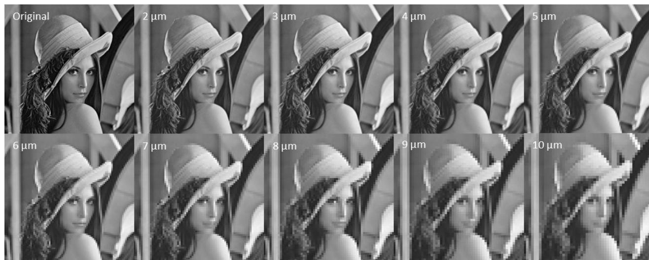
**Fig S1** Influence of the pixel size on the image quality as simulated by virtual LA-ICP-MS mapping of the Lenna image (the original has a pixel size of 1  $\mu\text{m}$ ).
