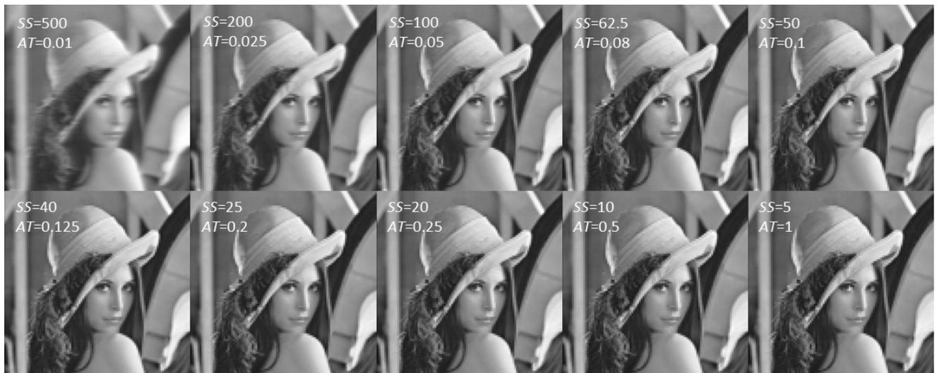
**Fig S4** Influence of scanning speed ( $SS$ ) / acquisition time ( $AT$ ), in combination with the system's response time  $FW0.01M$  of 0.1 s, on the image quality; both single pulse ( $n=1$ ) and multiple pulse ( $n=10$ ) analysis are simulated by virtual LA-ICP-MS mapping of the Lenna image according to steps 1, 3 and 4 of the simulation protocol in Fig. 1.
