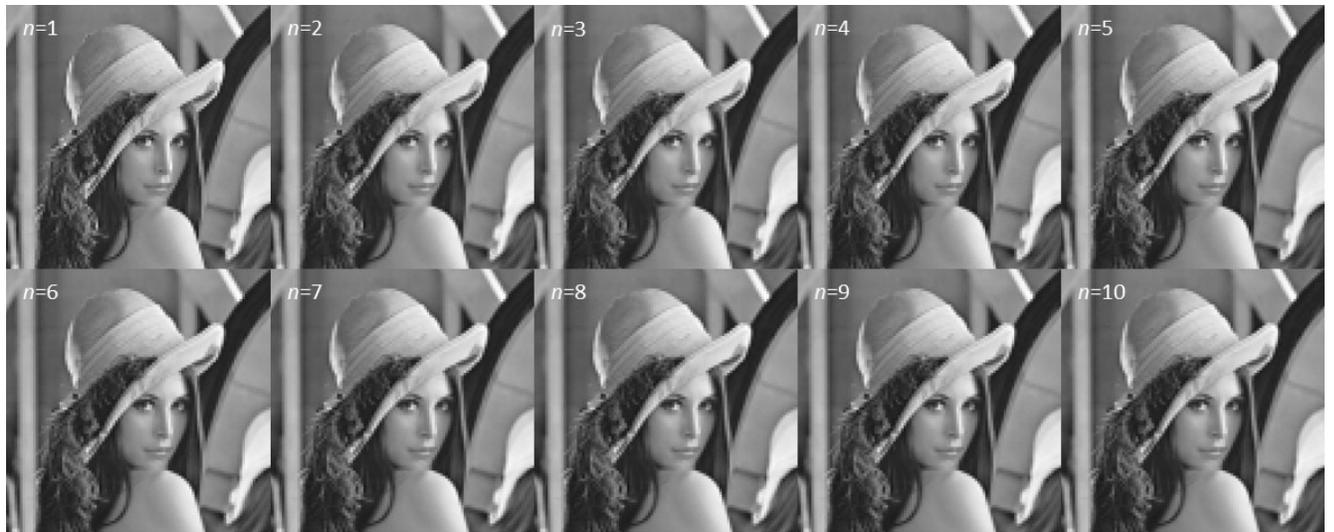
**Fig S3** Influence of laser sampling, i.e. the number of oversampled pixels ( $n$ ), on the image quality as simulated by virtual LA-ICP-MS mapping of the Lenna image via step 1 and 4 of the simulation protocol in Fig. 1.
