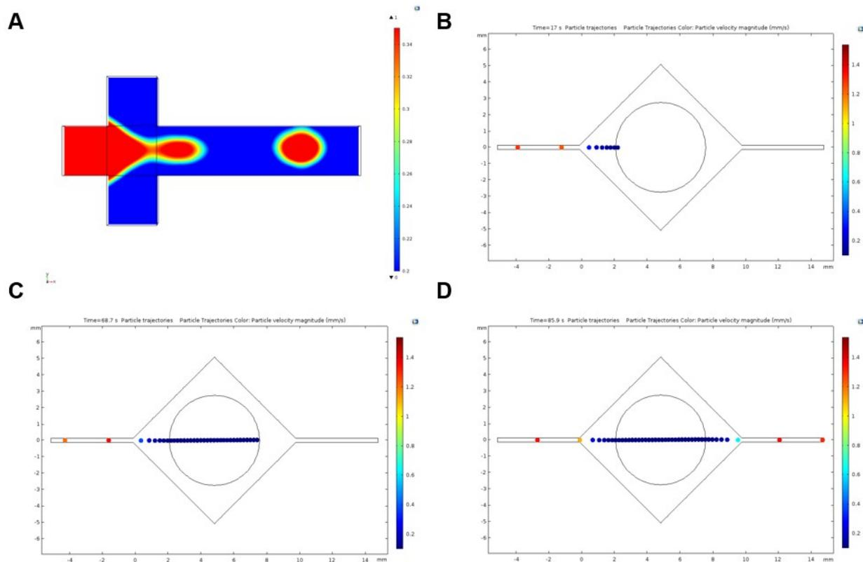
**Figure S2.** Computational simulation results of hydrogel droplets generation and crosslinking. (A) GelMA prepolymer droplet generation at the flow focusing cross junction (the color bar specifies the volume fraction of the dispersed phase). (B-D) Travel time estimation in the on-chip photocrosslinking chamber (diamond shape) with a laser beam spot (circular area). Droplets enter the crosslinking chamber (B), travel through the area of laser spot (C), and leave the crosslinking chamber (D).
