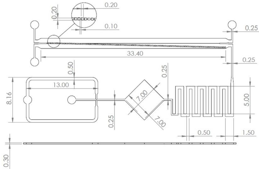
**Figure S1.** Detailed dimensional layout of the integrated microfluidic platform (unit: mm).
