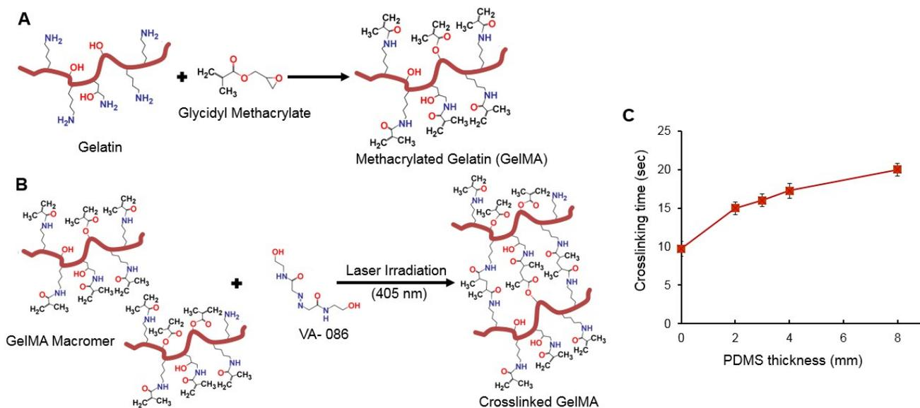
**Figure S4.** GelMA synthesis and photocrosslinking. (A) A schematic of the chemical reaction of gelatin and glycidyl methacrylate for conjugating methacryloyl groups. (B) A schematic of the GelMA photocrosslinking reaction under 405 nm blue laser irradiation in the presence of VA-086 photoinitiator. (C) Macroscale off-chip GelMA crosslinking time test under different thicknesses of PDMS pieces.
