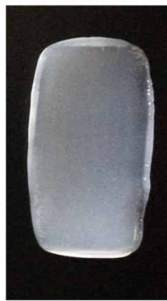
Fig. S3 PP slides molded by two different methods. PP slide with air bubbles molded by standard soft molding method (left); PP slide without air bubbles molded using thermally treated PDMS in our method (right).
