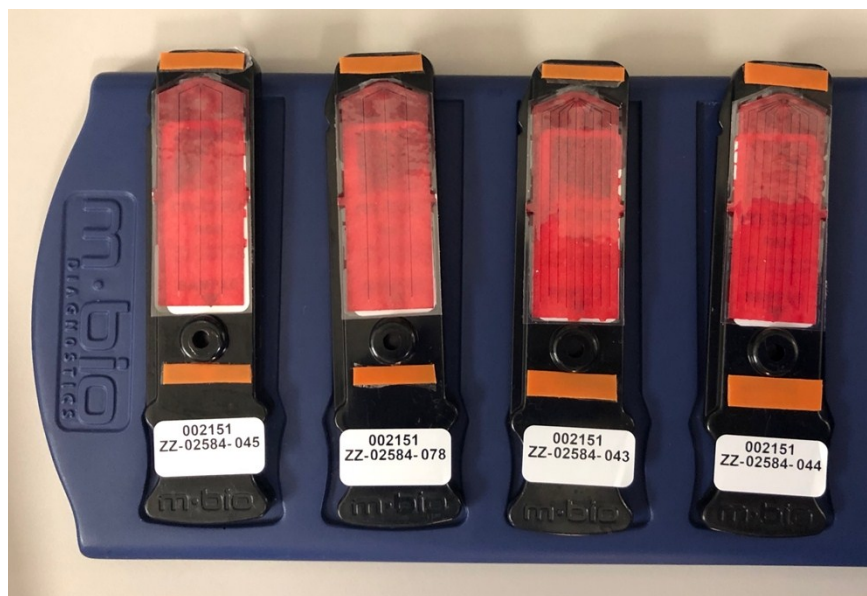
Figure S5: Demonstration of the grooved paper pumps attached to the commercially available microfluidic immunoassay cartridges (MBio Diagnostics, Inc., Boulder, CO, USA). The proposed pumps successfully transported (3-day old) human blood samples inside the cartridges.
