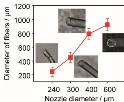
**Fig. S2** Nozzle effects on diameter of formed hollow microfibers. With keeping constant flow rate of the sodium alginate fluid, the diameter of microfibers increased with an increase of the diameter of nozzle. The s.d. from three measurements are shown as error bars.
