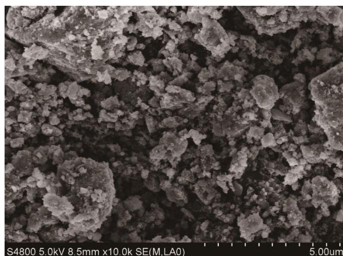
**Fig. S6** SEM image of magnetic particles of  $\text{Fe}_3\text{O}_4$ .
