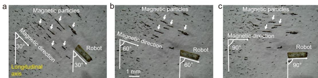
**Fig. S7** Controllable magnetic field for the motility of small-scale tubular robots. A simple device was assembled in which magnetic  $\text{Fe}_3\text{O}_4$  particles (average diameter: 200  $\mu\text{m}$ ) were utilized as reference objects which were capable of indicating the direction of magnetic field. A magnet was fixed over a control console that could be adjusted to shift along x, y and z axis respectively to alter the direction of magnetic field.
