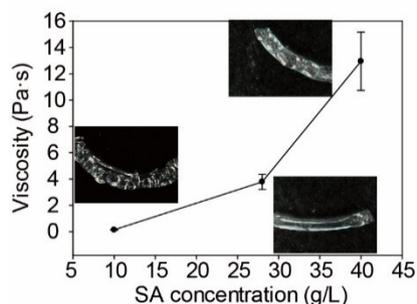
**Fig. S3** Viscosity effects on the morphologies of SA hydrogel hollow tubes. The viscosity of 0.5 Pa.s (SA concentration: 10 g/L) resulted in very soft microfibers with intermittent channel structures. Increasing viscosity to 13 Pa.s (SA concentration: 40 g/L) produced interconnected hollow microfibers, but the external surface of microfibers was not smooth. The viscosity at 4 Pa.s (SA concentration at 28 g/L) was optimal to form hollow microfibers.
