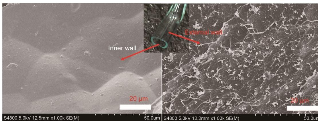
**Fig. S1** SEM images of sodium alginate hydrogel microfibers showing the surface morphologies of inner wall and external wall.
