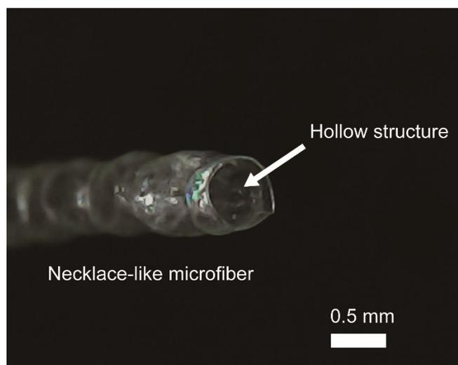
**Fig. S5** High-resolution image showing necklace-like geometry and hollow channel structure of sodium alginate hydrogel microfiber.
