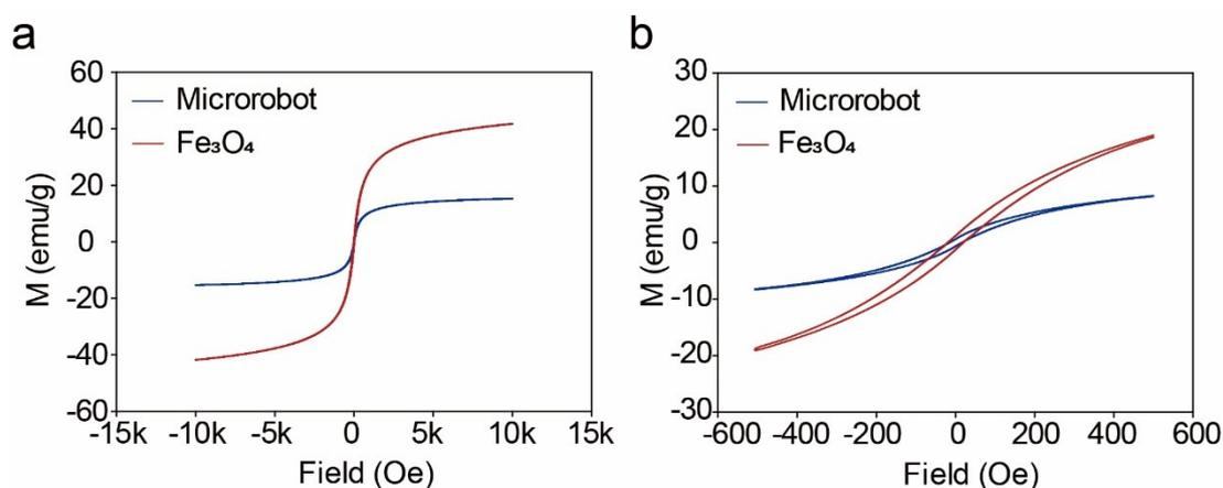
**Fig. S8 Magnetic properties.** (a) Magnetic property of  $\text{Fe}_3\text{O}_4$ -loaded hydrogel robot and  $\text{Fe}_3\text{O}_4$  particles were examined with a vibrating sample magnetometer (VSM, LakeShore7404) by cycling the applied field from -10 to +10 kOe (major hysteresis loop). (b) The minor hysteresis loop was obtained by cycling the applied field from -500 to +500 Oe. The test was at room temperature.
