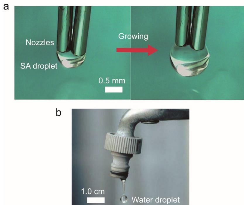
**Fig. S4** Demonstration on accumulation and growth of viscous liquid droplet. (a) Sodium alginate (SA) solution accumulated into a spherical droplet at the nozzle before entering into tris-HCl buffer solution of  $\text{CuSO}_4$  and  $\text{H}_2\text{O}_2$ . (b) A water droplet was formed when the flow rate of water was low enough. This phenomenon inspired us to design a two-nozzles microfluidic device for preparation of necklace-like microfibers.
