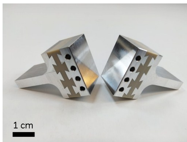
Figure S1. Heatable sample holders. The heating coil was introduced in the holes. The heatable plates were isolated from the rest of the sample holder and device by PEEK 1000 insulator layer (light brown). The sample was attached directly on heatable plate by high temperature epoxy.
