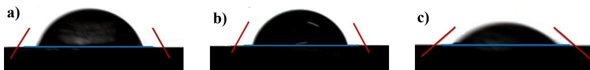
Figure S2 Contact angles of (a) the bulk MoS 2 , (b) MoS 2 /rGO and (c) SiQDs-MoS 2 /rGO-2.
