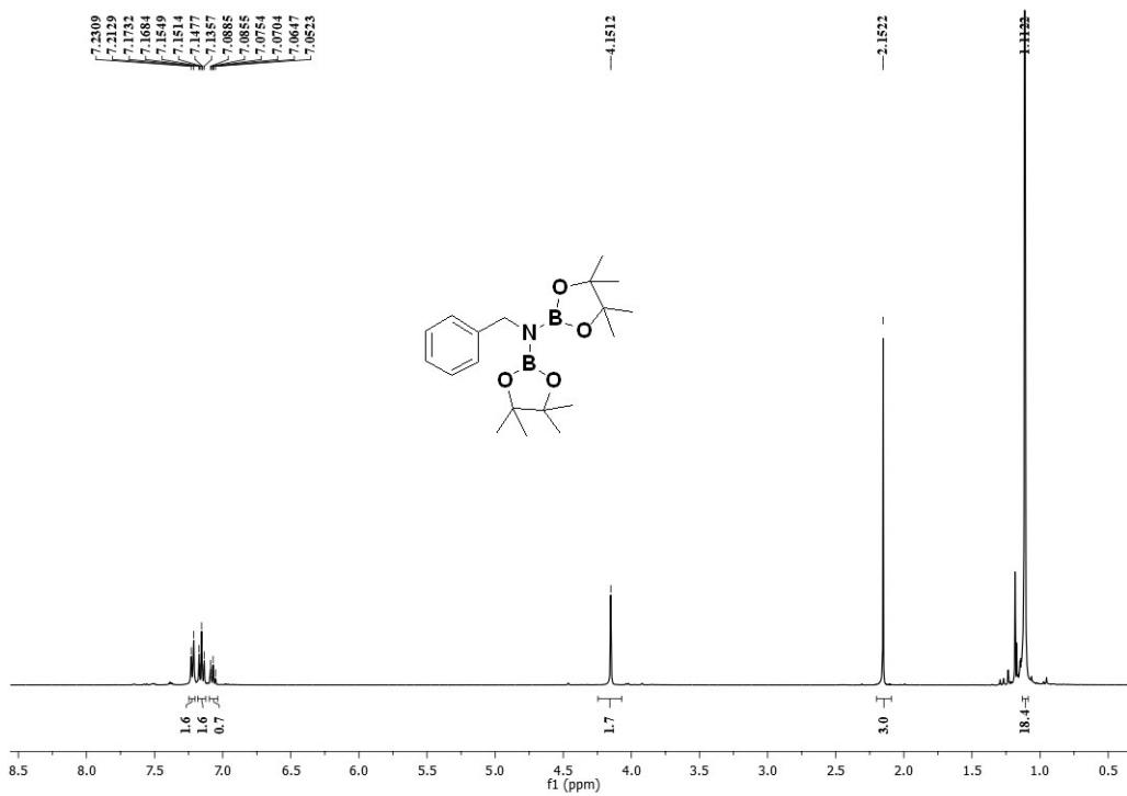
**Figure FS14.**  $^1\text{H}$  NMR spectra of complex **2d**.
