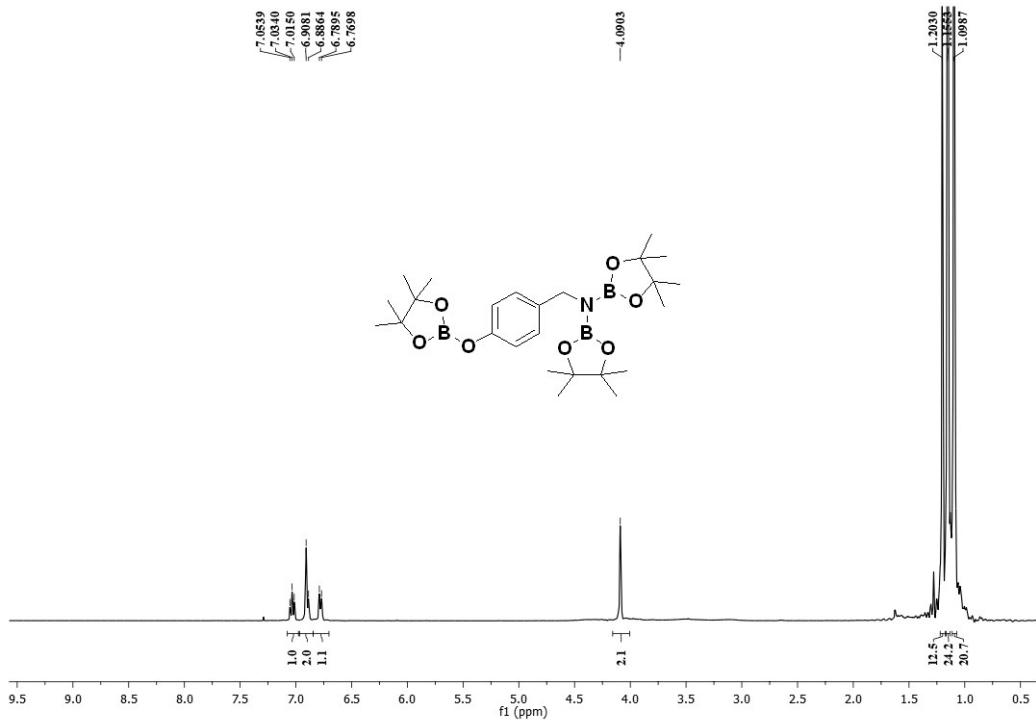
**Figure FS78.**  $^1\text{H}$  NMR spectra of complex 3e.
