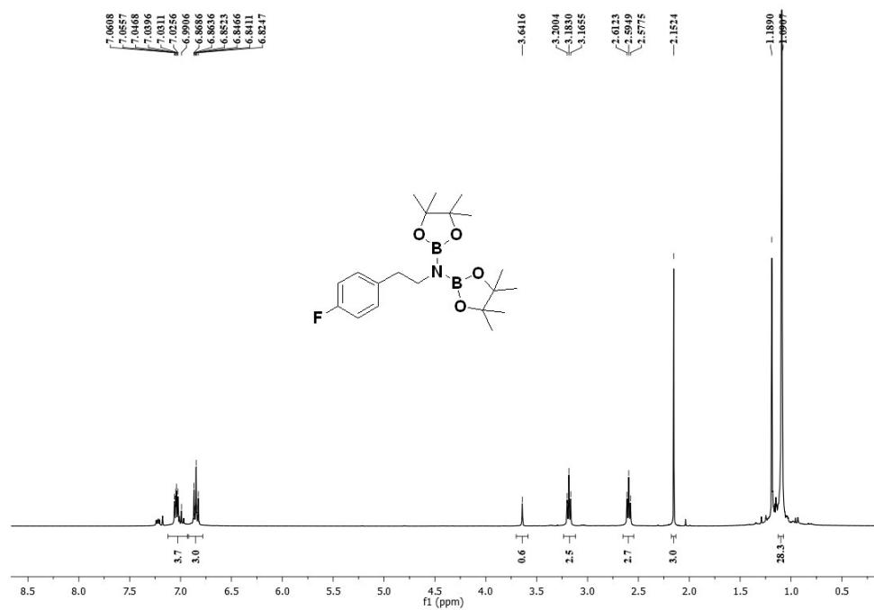
**Figure FS60.**  $^1\text{H}$  NMR spectra of complex **2s**.
