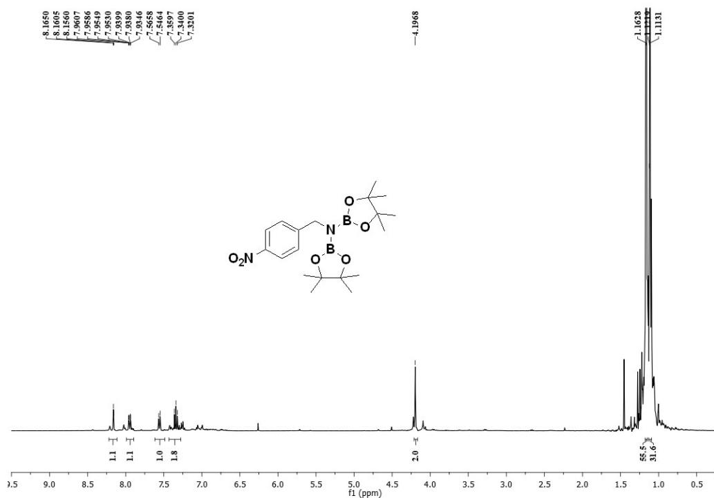
**Figure FS69.**  $^1\text{H}$  NMR spectra of complex **3a**.
