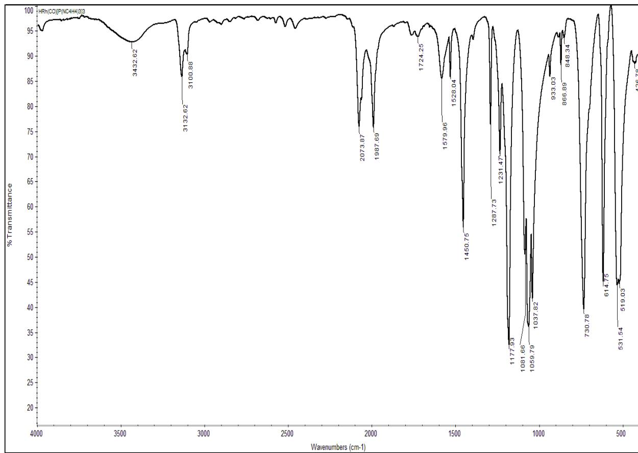
Fig. S1. IR- spectra (KBr) of  $\text{HRh}(\text{CO})\{\text{P}(\text{NC}_4\text{H}_4)_3\}_3$
