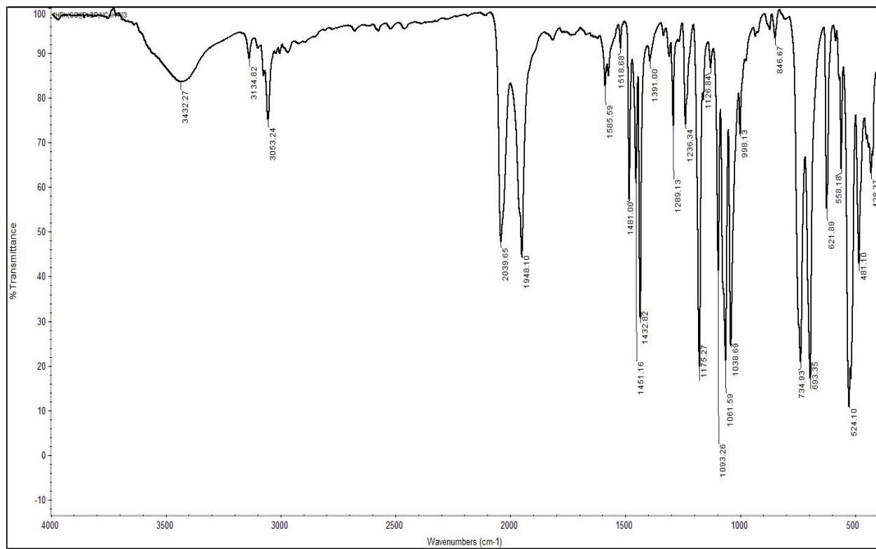
Fig. S3. IR- spectra (KBr) of  $\text{HRh}(\text{CO})\{\text{Ph}_2\text{P}(\text{NC}_4\text{H}_4)\}_3$
