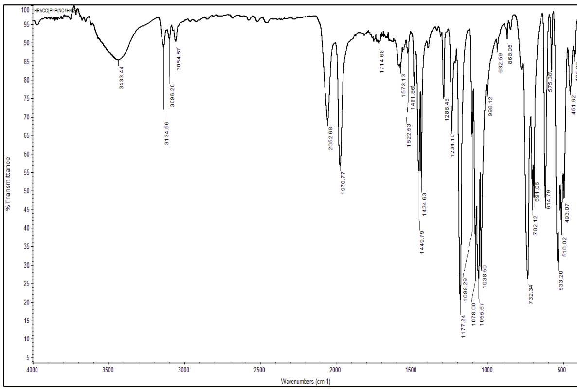
Fig. S2. IR- spectra (KBr) of  $\text{HRh}(\text{CO})\{\text{PhP}(\text{NC}_4\text{H}_4)_2\}_3$
