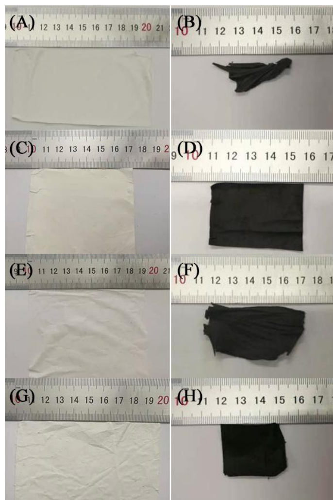
Figure S2. (A) PAN membranes, (B) C nanofiber membranes, (C) \text{TiO}_2 @PAN membranes, (D) \text{TiO}_2 @C nanofiber membranes, (E) GO@PAN membranes, (F) GO@C nanofiber membranes, (G) \text{TiO}_2 @GO@PAN membranes and (H) \text{TiO}_2 @GO@C nanofiber membranes.
