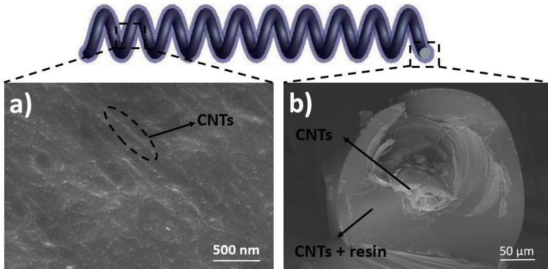
**Figure S2.** SEM images of the surface (a) and cross-section (b) for the CNT nanocomposite yarn artificial muscle. We can see the CNTs with orientation on the nanocomposite artificial muscle surface (a), and cross-section of the spring-like nanocomposite artificial muscle was divided into two parts (b), the results indicated that epoxy resin was infiltrated into the spiral CNT yarn.
