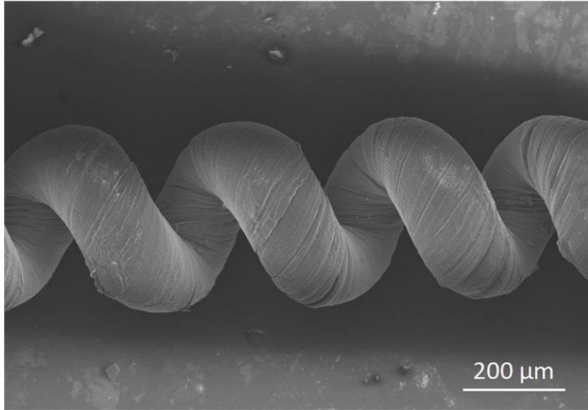
**Figure S1.** The pre-stretched spiral CNT fiber.
