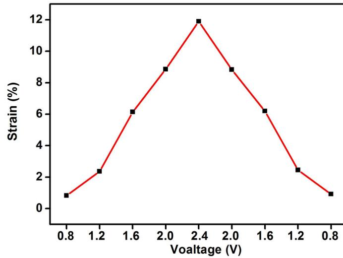
**Figure S5.** The strain variation of the CNT nanocomposite yarn artificial muscle when the applied voltages increased first and then decreased. We can see that the strain of the nanocomposite yarn artificial muscle can be changed with the applied voltages, which proves that the artificial muscle can achieved reversible and controllable deformation.
