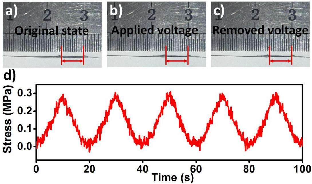
**Figure S3.** Morphological changes (a-c) and output stress under pulsed voltages vs. Time (d) for the pure CNT yarn. (a-c) There is no morphological changes for pure CNT yarn when the voltage was applied. (d) The pure CNT yarn also can output periodic stress under the pulsed voltage, but it was very small ( $< 0.3$  MPa), which indicated that the driving deformation of the CNT nanocomposite yarn artificial muscle is realized by the resilience force of the spring.
