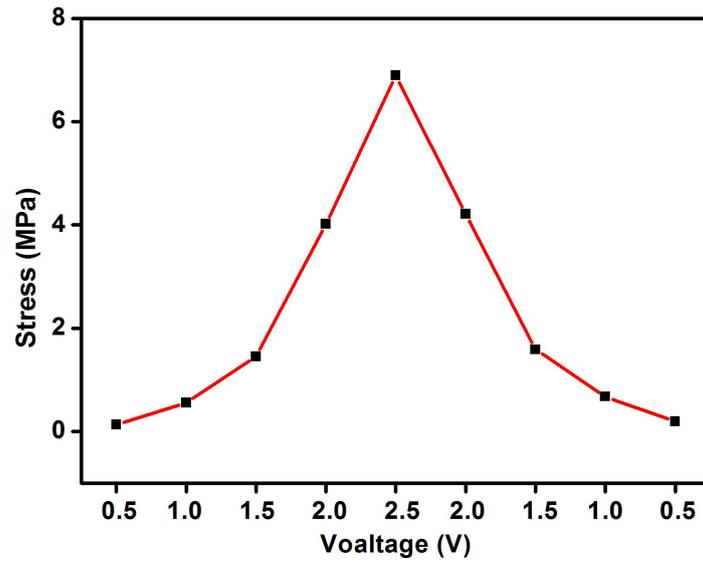
**Figure S6.** The output stress variation of the CNT nanocomposite yarn artificial muscle when the applied voltages increased first and then decreased.
