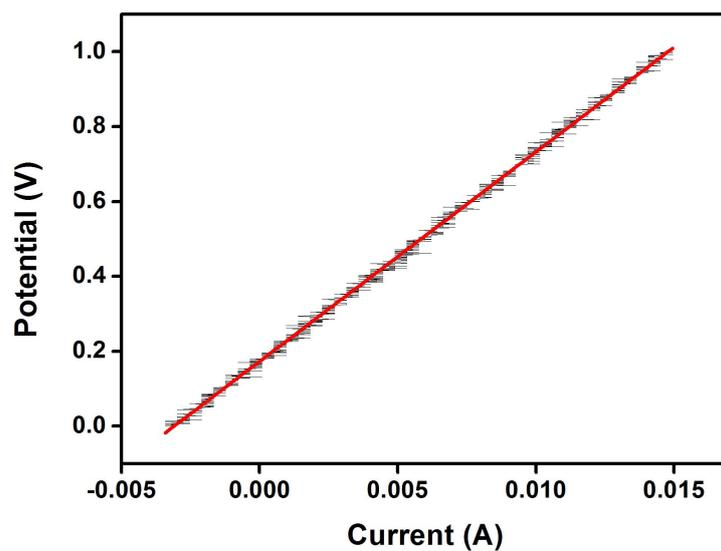
**Figure S7.** The Volt-Ampere(V-A) curve of the CNT nanocomposite yarn artificial muscle.
