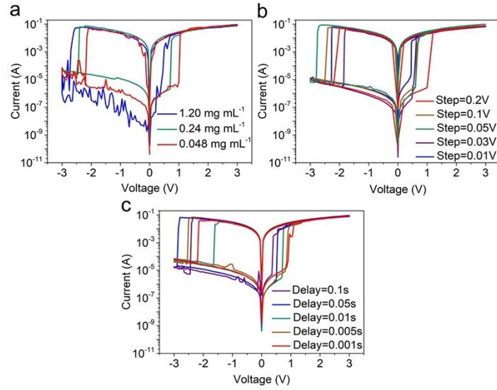
**Figure S10.** a) The  $I$ - $V$  curves of memories with different  $\text{Ti}_3\text{C}_2$  concentrations. b) The  $I$ - $V$  curves of RRAM with different voltage step. c) The  $I$ - $V$  curves of memories with different delay times.
