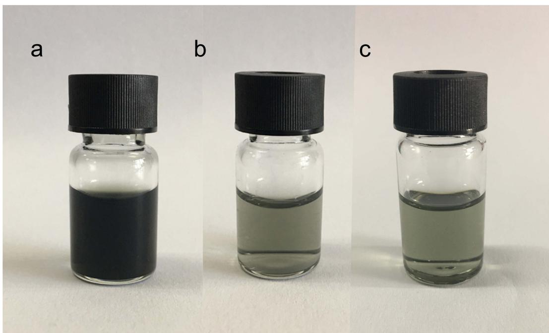
**Figure S1.** (a) Photograph of the MXene ( $\text{Ti}_3\text{C}_2$ ) colloid solution (A,  $2.5 \text{ mg mL}^{-1}$ ). (b) The mixture of  $\text{Ti}_3\text{C}_2$  ( $0.24 \text{ mg mL}^{-1}$ ) and PVPy ( $20 \text{ mg mL}^{-1}$ ). (c) The mixture of  $\text{Ti}_3\text{C}_2$  ( $0.24 \text{ mg mL}^{-1}$ ) and PVPy ( $20 \text{ mg mL}^{-1}$ ) after 30 days, indicating the excellent uniformity.
