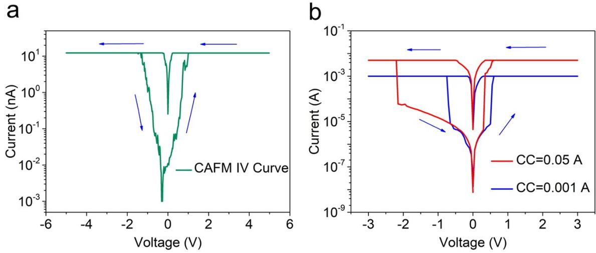
**Figure S7.** The  $I$ - $V$  curves collected by C-AFM using Ramp program (a) and probe station (b).
