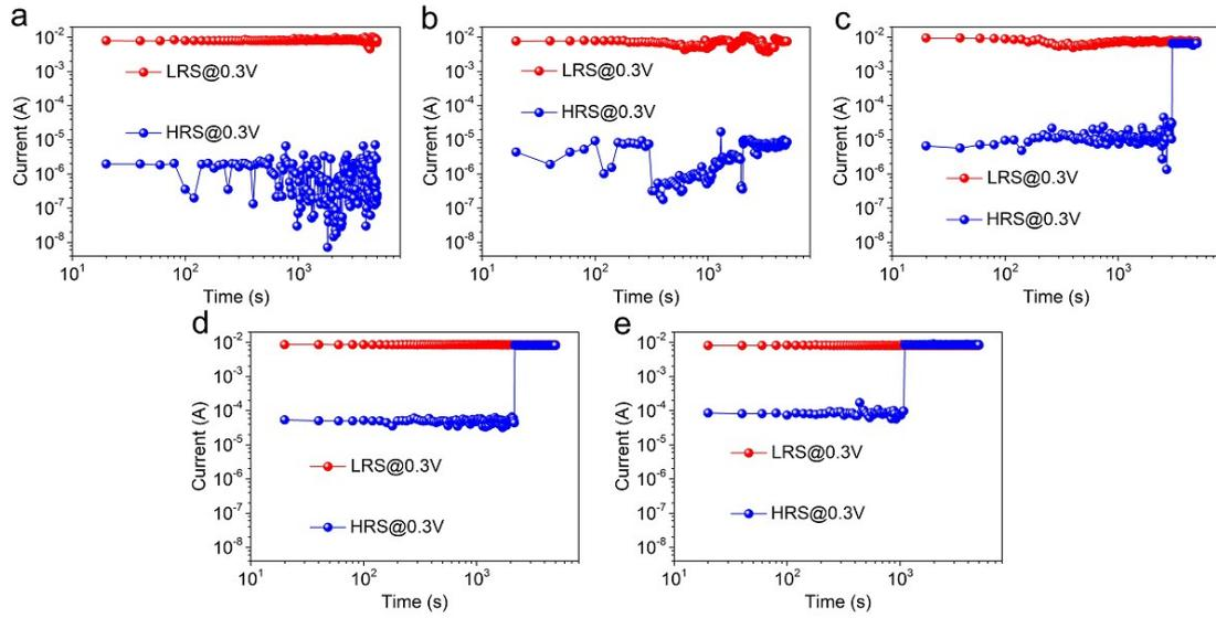
**Figure S5.** The retention characters of  $\text{Ti}_3\text{C}_2$  based RRAM under different temperatures (a: 30°C, b: 50°C, c: 70°C, d: 90°C, e: 110°C).
