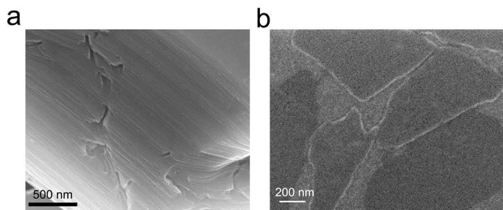
**Figure S3.** The SEM images of the MAX ( $\text{Ti}_3\text{AlC}_2$ ) after HF treatment (a) and dispersive MXene (b).
