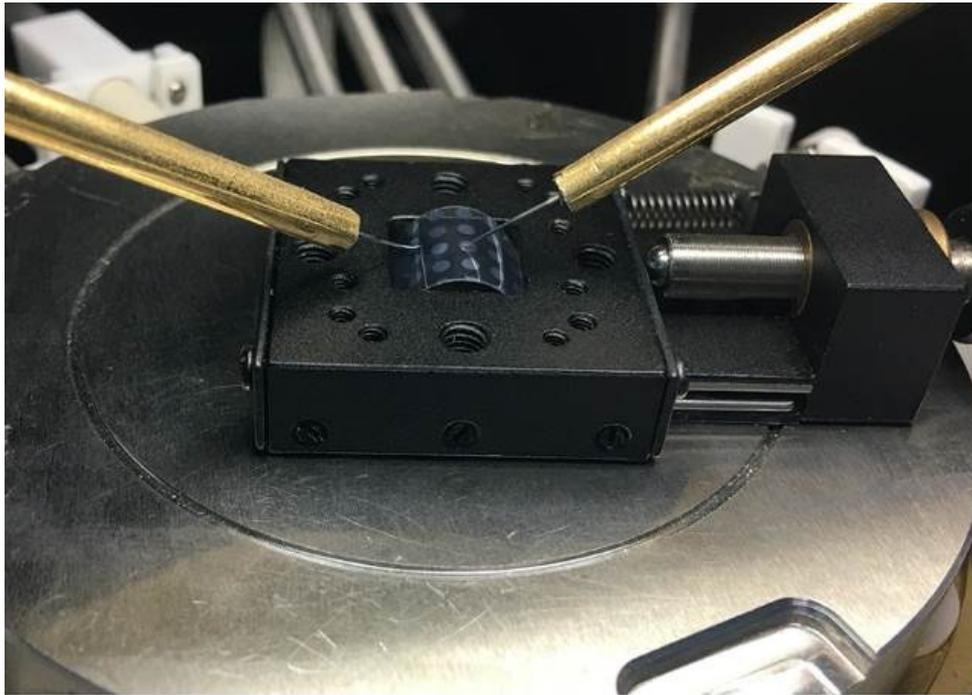
**Figure S13.** Illustration of test condition during the bending test (the measured devices were near the middle of the sample).
