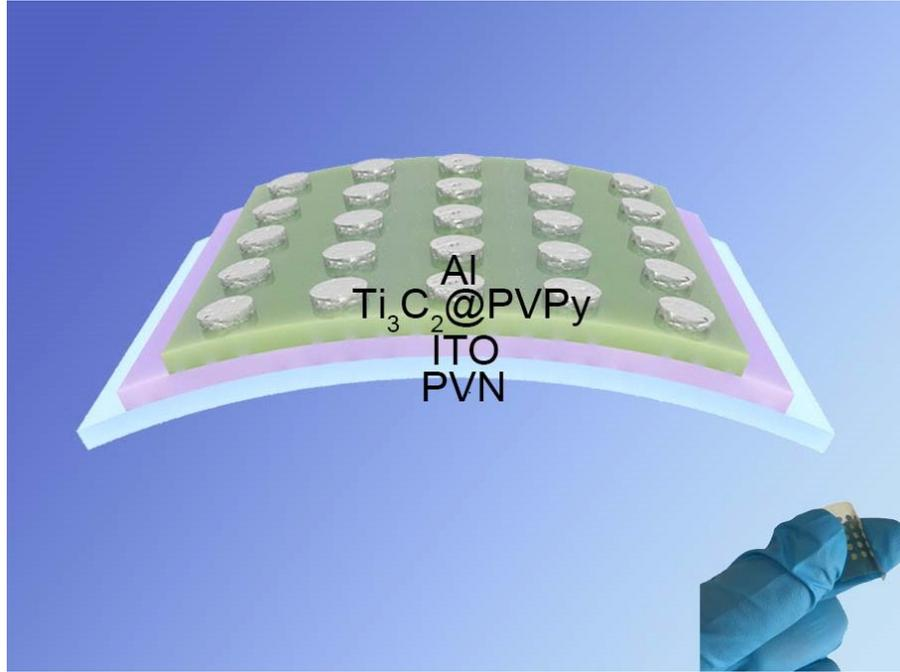
**Figure S12.** Schematic of the PEN/ITO/Ti<sub>3</sub>C<sub>2</sub>@PVPy/Al (inset: the optical image of Ti<sub>3</sub>C<sub>2</sub> memory devices fabricated on flexible substrate).
