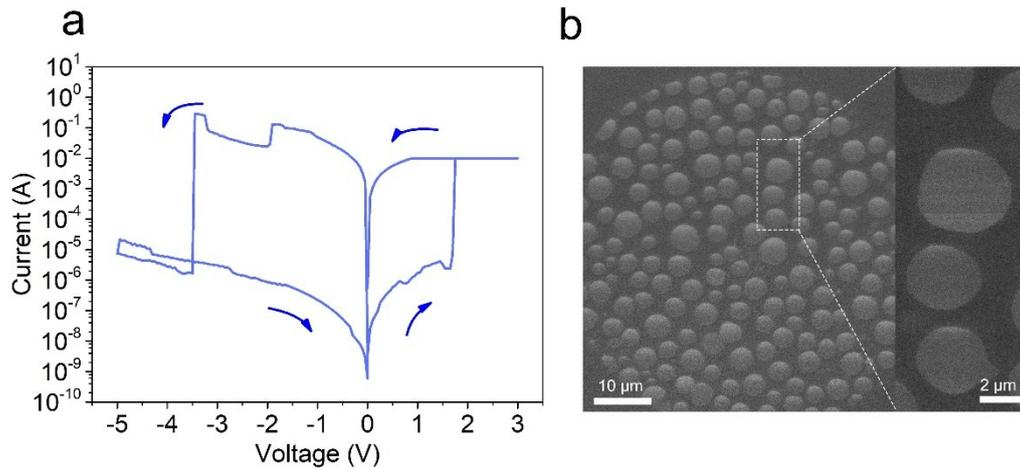
**Figure S9.** a) The  $I-V$  curve of small size device (diameter: 3-5 $\mu\text{m}$ ) collected using probe station. b) The pictures of small size device collected by SEM; The subminiature device was fabricated using micrograte supporting film (Zhongjingkeyi(Beijing) Films Technology Co., Ltd) as shadow mask; The diameter of probe tip for subminiature device is about 0.2  $\mu\text{m}$  (PL-T02, Zhanxin (Shenzhen) Technology Co., Ltd).
