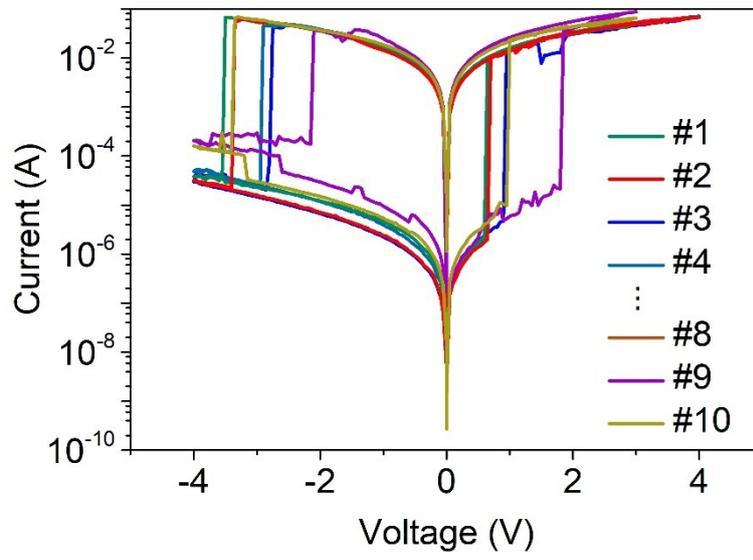
**Figure S8.** The  $I$ - $V$  curves of the small size cross-point  $\text{Ti}_3\text{C}_2$  based devices ( $100\ \mu\text{m}$ ).
