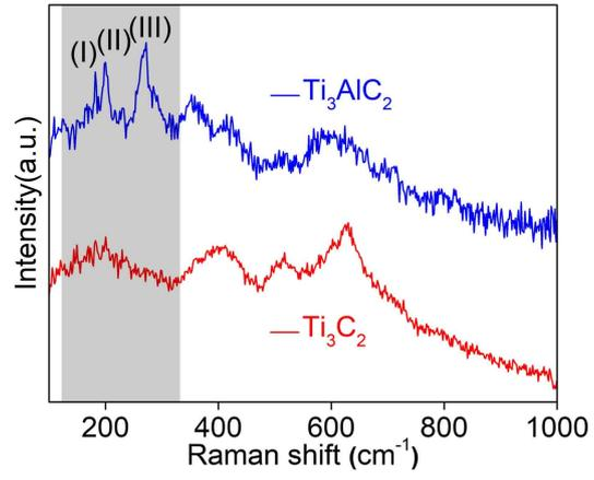
**Figure S2.** Raman spectra of the Ti<sub>3</sub>AlC<sub>2</sub> MAX (powder) and Ti<sub>3</sub>C<sub>2</sub> MXene film.
