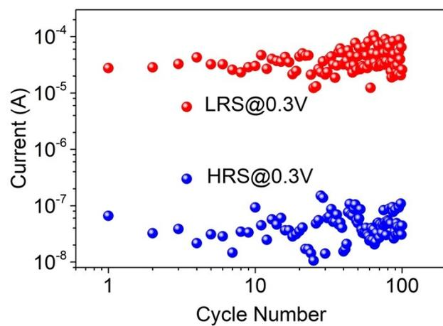
**Figure S14.** The reliability of the  $\text{Ti}_3\text{C}_2$ -based flexible memories.
