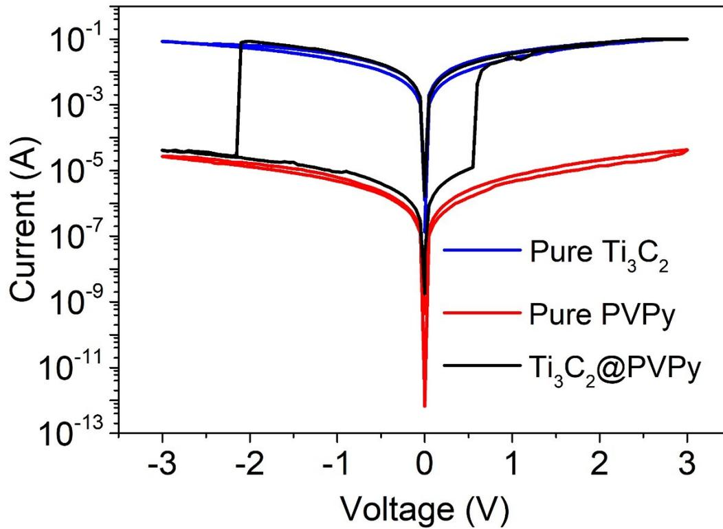
**Figure S4.** The *I-V* curves of pure  $\text{Ti}_3\text{C}_2$ , pure PVPy and  $\text{Ti}_3\text{C}_2@\text{PVPy}$  mixtures (PVPy:  $20 \text{ mg mL}^{-1}$ ,  $\text{Ti}_3\text{C}_2$ :  $0.24 \text{ mg mL}^{-1}$ ) based RRAM devices.
