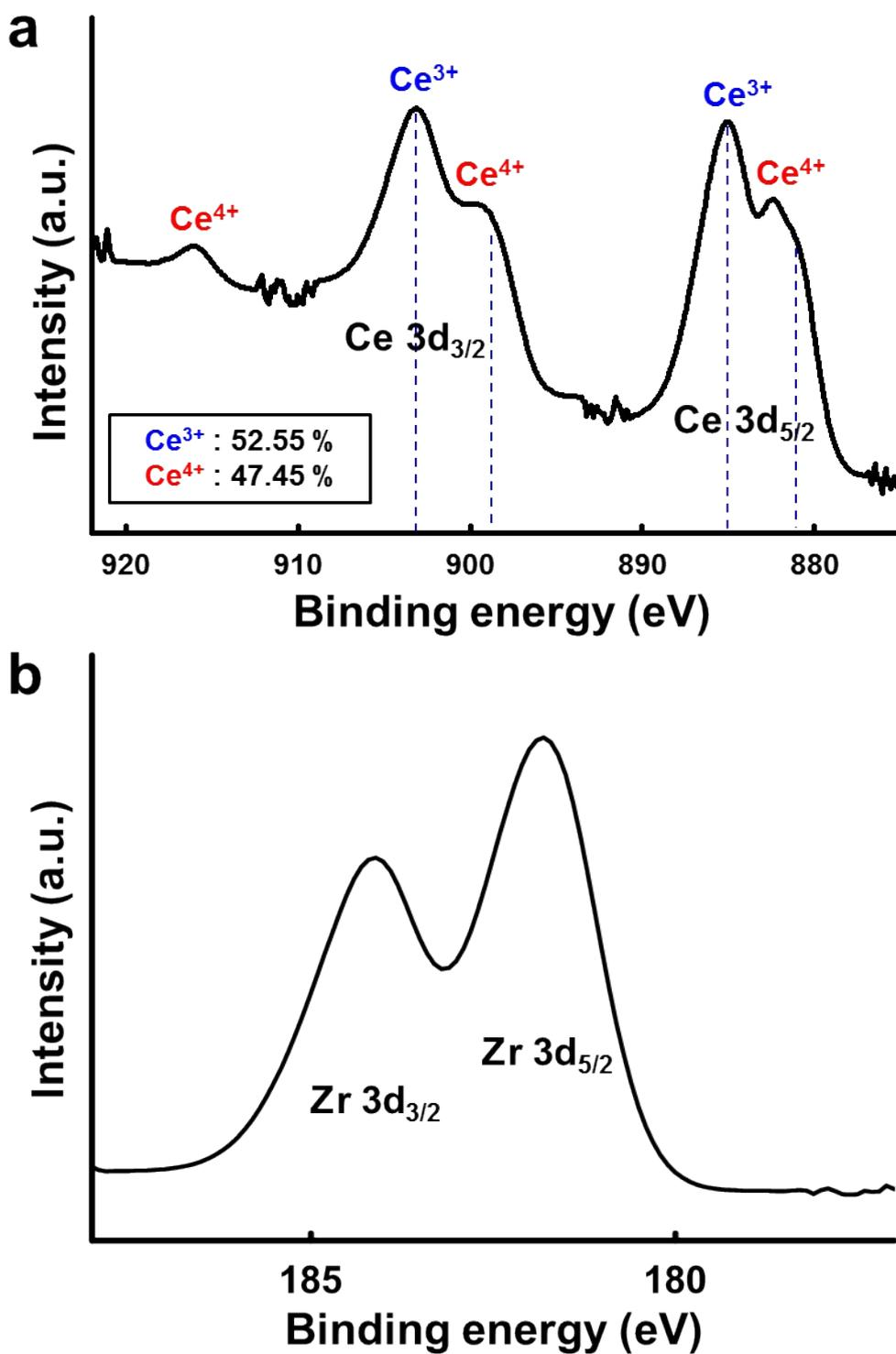
Figure S3. XPS analysis of (a) Ce (Ce<sup>3+</sup>: 52.55% and Ce<sup>4+</sup>: 47.45%) and (b) Zr ions in 7CZ NPs.
