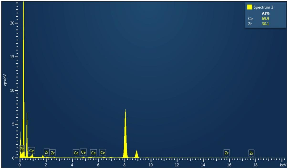
**Figure S4.** EDS spectra, confirming atomic compositions of 7CZ NPs (69.9 at% Ce and 30.1 at% of Zr).
