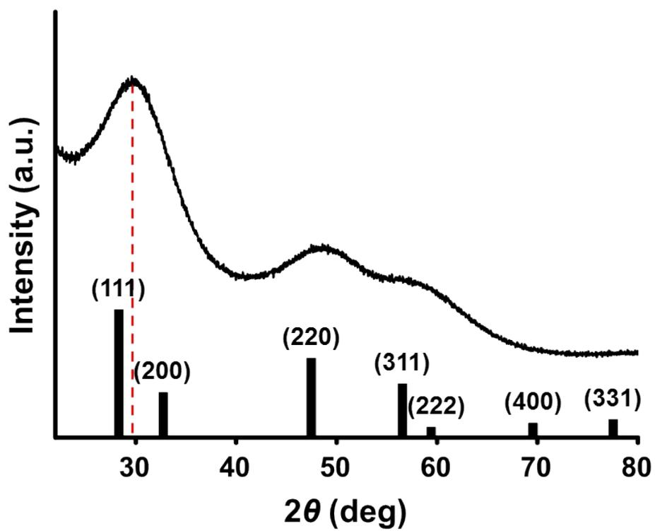
**Figure S2.** XRD pattern of 7CZ NPs. The black bars indicate the reference peaks of ceria. The red dashed line represents that fluorite peak (111) of 7CZ NPs is shifted.
