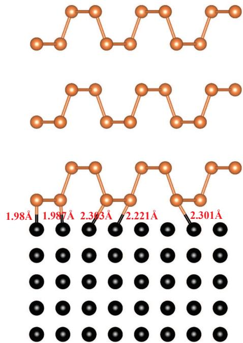
**Figure S1** Bond lengths between the trilayer BP and Ni electrode interface.
