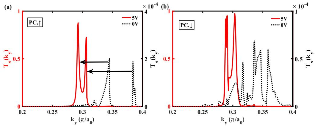
**Figure S3** The transmission coefficients  $T_\sigma(k_y)$  versus transverse momentum  $k_y$  when  $V_g = 0, 5$  V. (a) Spin up component in PC. (b) Spin down component in PC.
