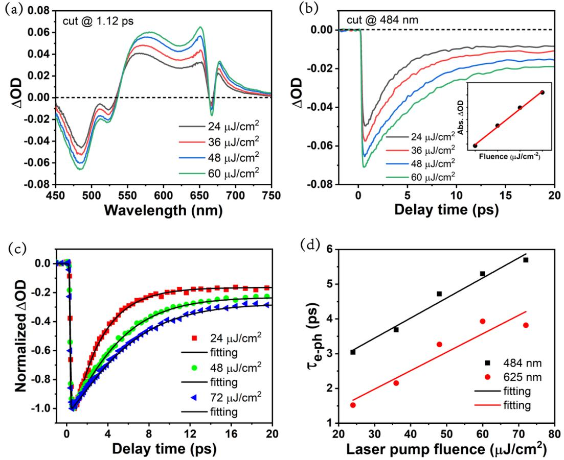
Figure S8. (a) Fluence-dependent transient  $\Delta OD$  spectra around  $20^\circ$  azimuthal angle at the delay time of 1.12 ps. (b) Fluence-dependent  $\Delta OD$  kinetics at the wavelength of 484 nm. Inset: Absolute  $\Delta OD$  versus the pump fluence. (c) Fluence-dependent normalized  $\Delta OD$  kinetics for three specific fluences of 24, 48, 72  $\mu J/cm^2$ . (d) A plot of the electron-phonon relaxation times against the pump fluence.
