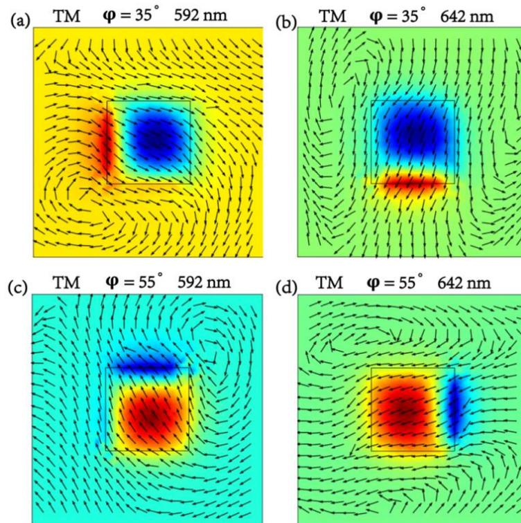
Figure S11. Electric field pattern of  $E_z$  and magnetic field vector distribution of  $H_x$ ,  $H_y$  under TM polarization. The azimuthal angles are  $35^\circ$  and  $55^\circ$  in (a, b) and (c, d), respectively. Note that: All intensities are normalized by the same scale bar.
