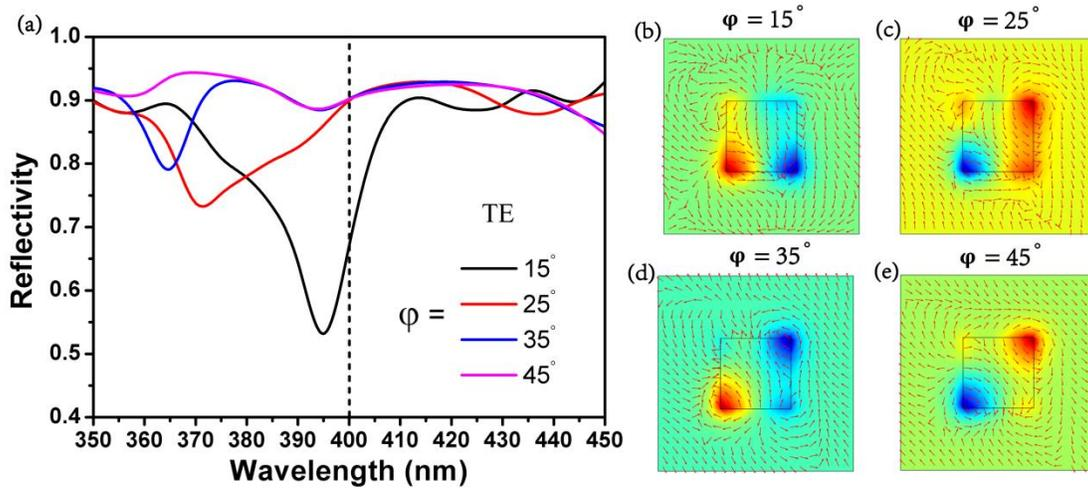
Figure S4. (a) The simulated reflectance spectra with azimuthal angles of  $15^\circ \sim 45^\circ$  in the wavelength range of 350 ~ 450 nm under TE polarization, and (b-e) corresponding electromagnetic field profile of a single nanohole cell at the wavelength of 400 nm.
