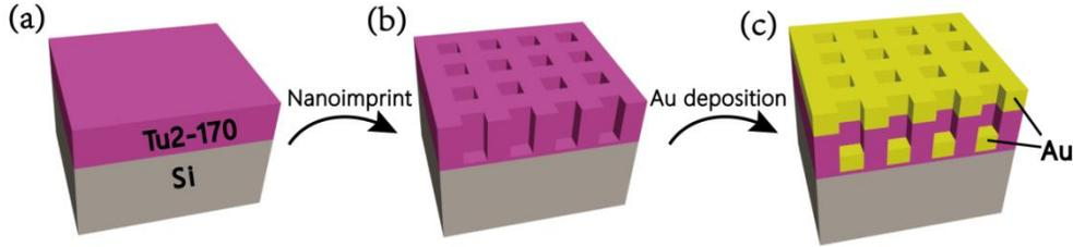
Figure S1. Sample fabrication processes
