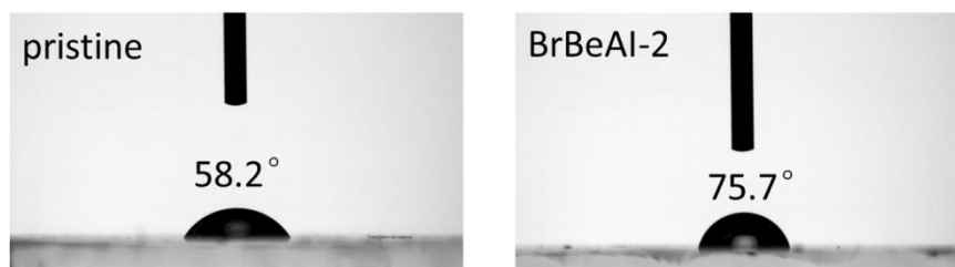
Fig. S9. The water contact angle characterization for pristine perovskite and BrBeAl-2 thin films.
