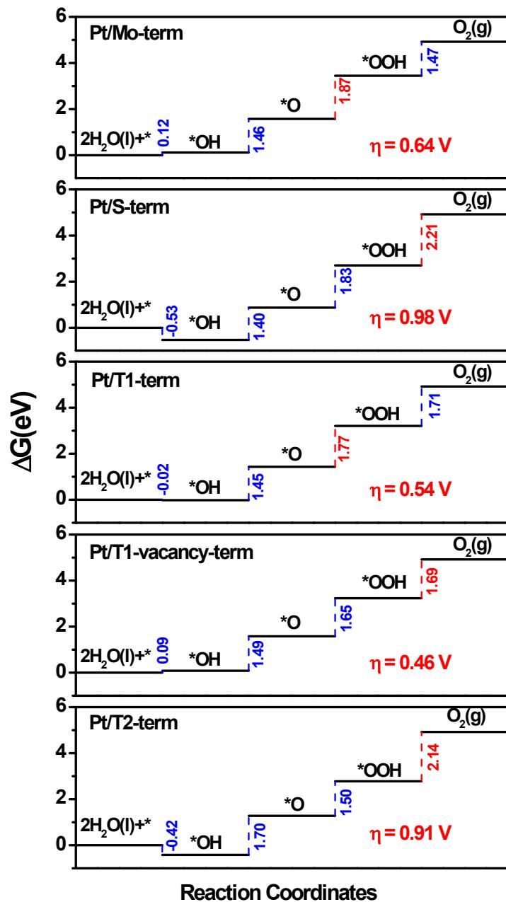
**Figure S19** Free energy diagram for Pt doped MoS<sub>2</sub> terminations for OER, where the elementary reaction with  $\Delta G$  in red shows the potential-determining step.
