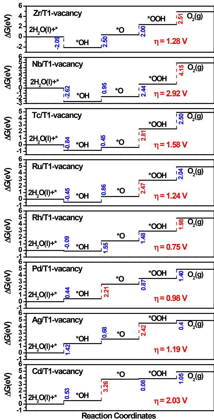
**Figure S7** Free energy diagram for 4d single TM atom doped T1-vacancy term for OER, where the elementary reaction with  $\Delta G$  in red shows the potential-determining step.
