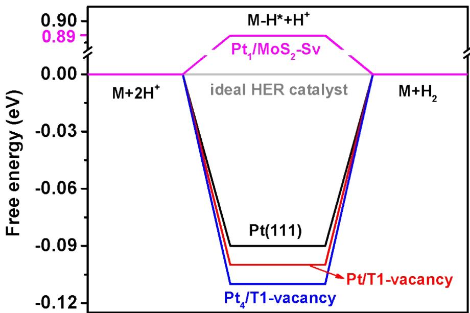
**Figure S12** Free energy diagram for HER on ideal electrocatalyst, Pt(111), Pt/T1-vacancy, Pt<sub>4</sub>/T1-vacancy and Pt<sub>1</sub>/MoS<sub>2</sub>-Sv at zero electrode.
