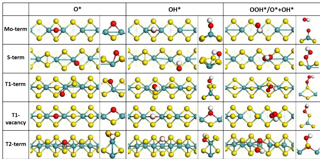
**Figure S4** The  $O^*$ ,  $OH^*$  and  $OOH^*$  adsorption configurations on different  $MoS_2$  edges.
