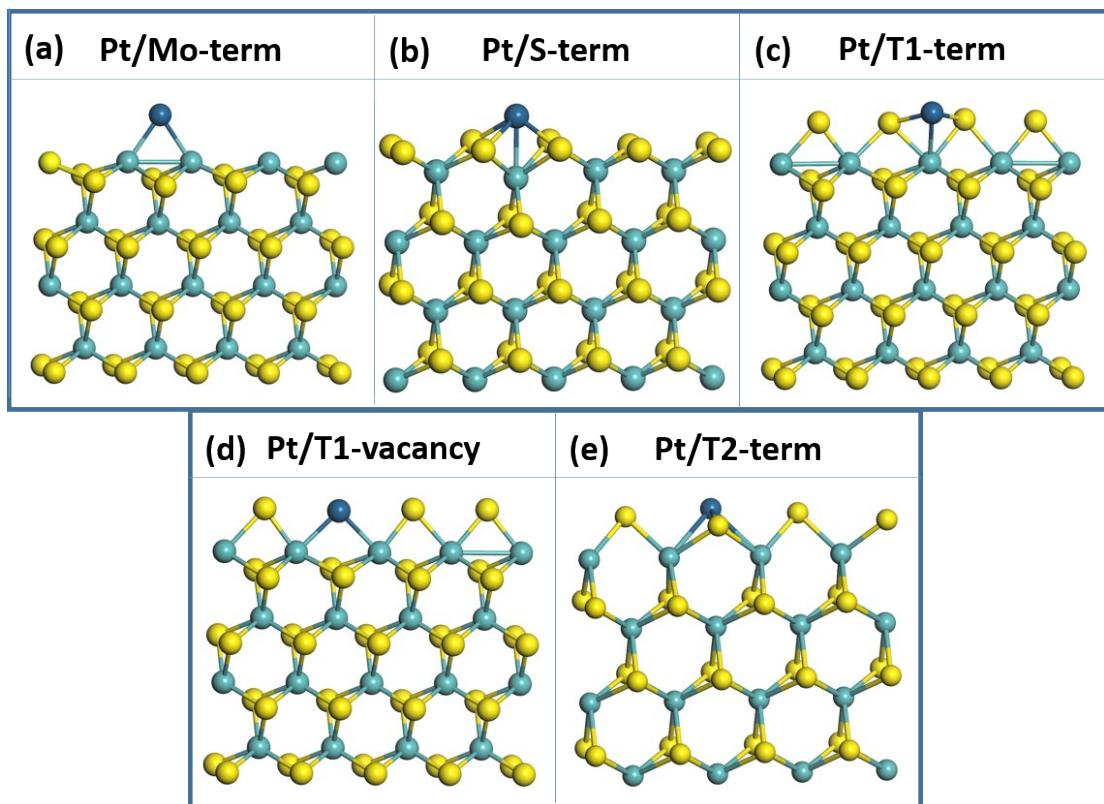
**Figure S9** The crystal structure of (a) Pt/Mo-term, (b) Pt/S-term, (c)Pt/T1-term, (d)Pt/T1-vacancy and (e)Pt/T2-term.
