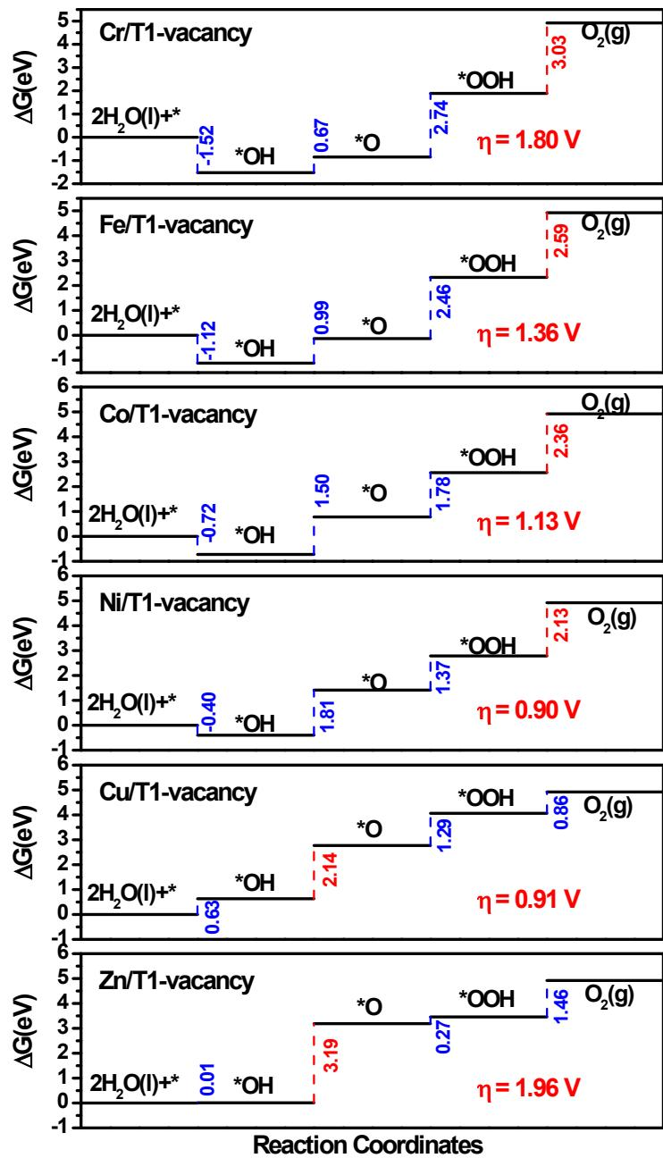
**Figure S6** Free energy diagram for 3d single TM atom doped T1-vacancy term for OER, where the elementary reaction with  $\Delta G$  in red shows the potential-determining step.
