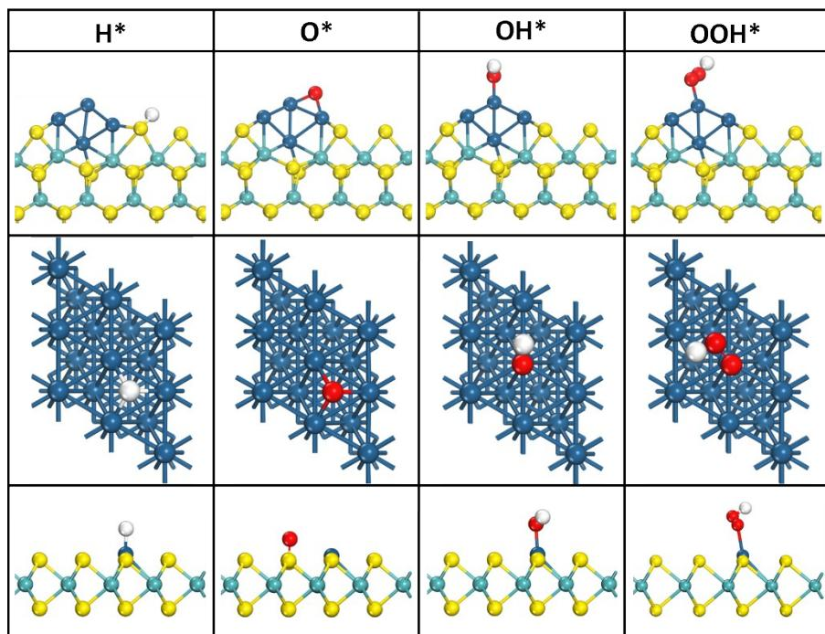
**Figure S13** The favorable  $H^*$ ,  $O^*$ ,  $OH^*$  and  $OOH^*$  adsorption configurations on  $Pt_4/1T$ -vacancy term,  $Pt$  (111) surface and  $Pt_1/MoS_2$ -Sv surface.
