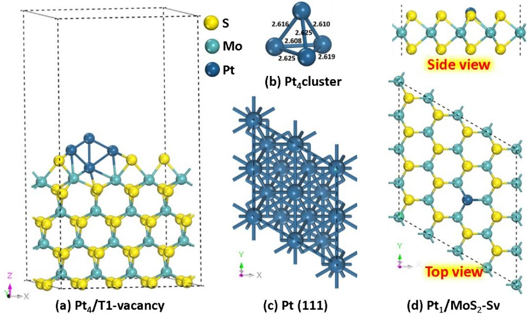
**Figure S11** (a) The most stable crystal structure of Pt<sub>4</sub>/1T-vacancy with Pt<sub>4</sub> cluster doped on 1T-vacancy. (b) The energetically favorable Pt<sub>4</sub> cluster. The numbers show the bond length of Pt<sub>4</sub> cluster. (c) the top view of Pt (111) slab. (d) the side and top view of Pt<sub>1</sub>/MoS<sub>2</sub>-Sv.
