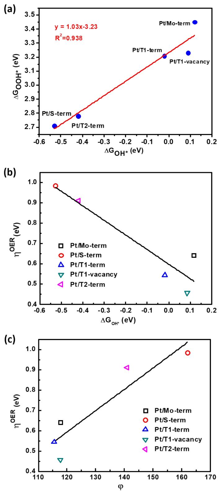
**Figure S20** The linear relationship between (a)  $\Delta G_{\text{OH}^*}$  and  $\Delta G_{\text{OOH}^*}$ , (b)  $\Delta G_{\text{OH}^*}$  and the Overpotential ( $\eta^{\text{OER}}$ ), and (c)  $\eta^{\text{OER}}$  and structure descriptor ( $\phi$ ) in different Pt/MoS<sub>2</sub> systems.
