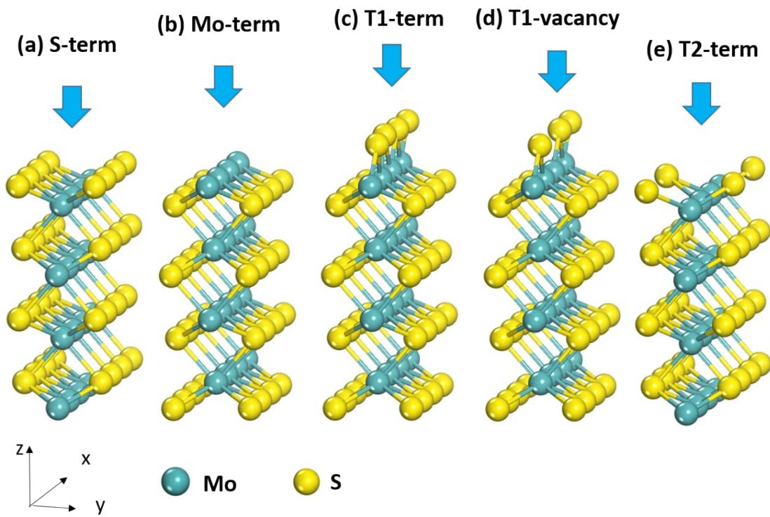
**Figure S1** The crystal structure of hexagonal MoS<sub>2</sub> edges with (a) S termination, (b) Mo termination, (c) T1 termination: 50% sulfur addition at the initial Mo termination, (d) T1 vacancy termination: 37.5% surface sulfur coverage and (e) T2 termination: 50% sulfur removal at the S termination.
