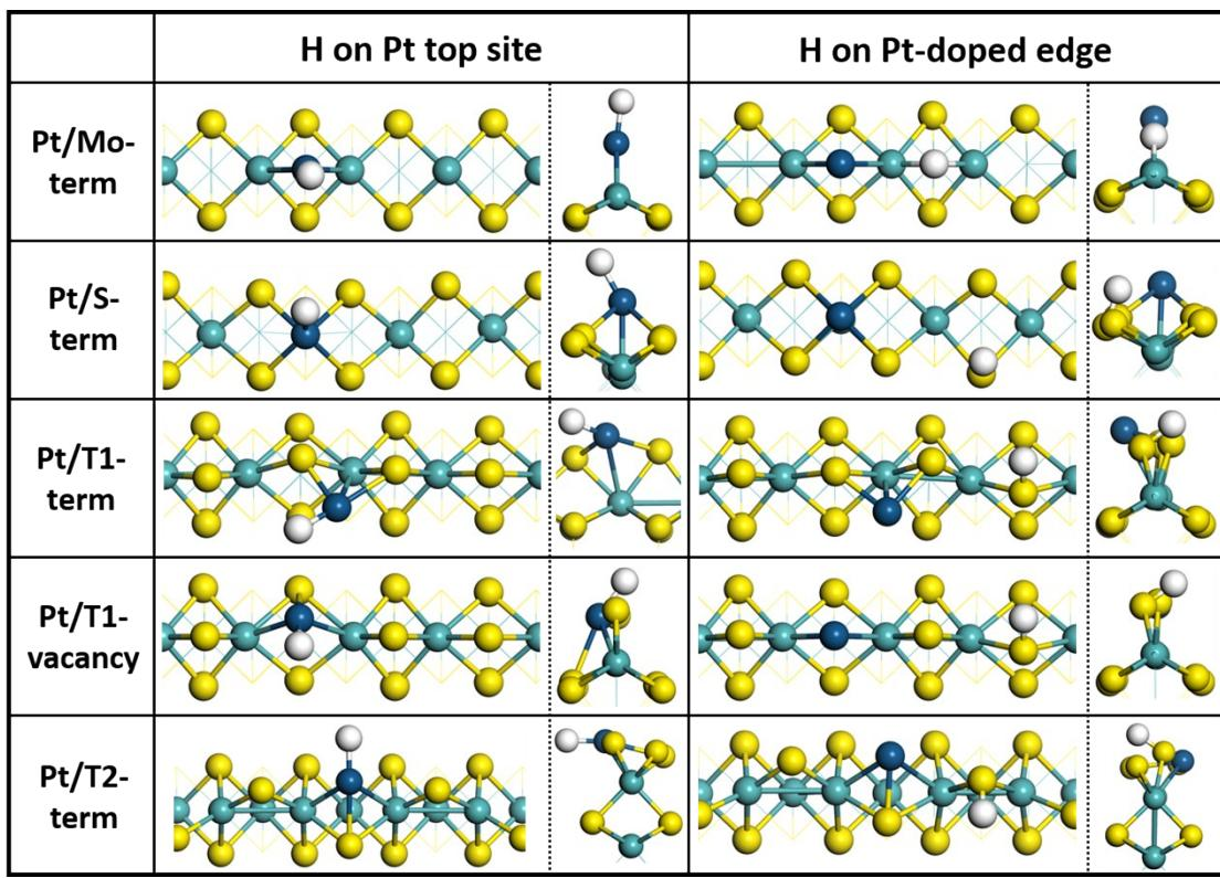
**Figure S16** The favorable  $\text{H}^*$  adsorption configurations on Pt/MoS<sub>2</sub> edges with H adsorbed on Pt and edge. The figure on the left side of the dashed line is top view, and the figure on the right side of the dashed line is side view.
