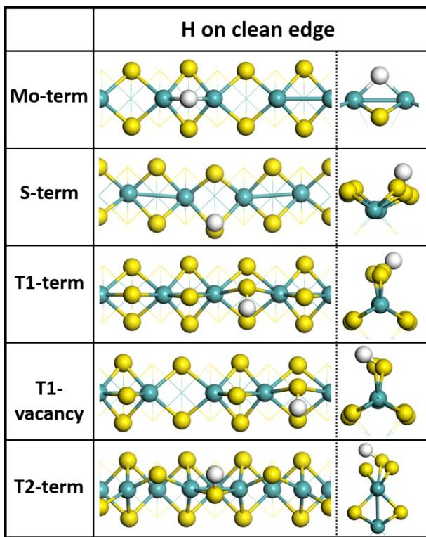
**Figure S3** The favorable H\* adsorption configurations on clean MoS<sub>2</sub> edges. The figure on the left side of the dashed line is top view, and the figure on the right side of the dashed line is side view.
