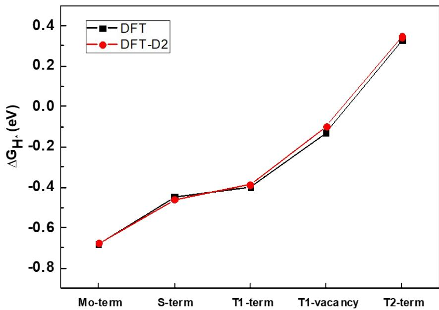
**Figure S2** The comparison of calculated  $\Delta G_{H^*}$  of different MoS<sub>2</sub> edges by using DFT method with and without D2 correction.
