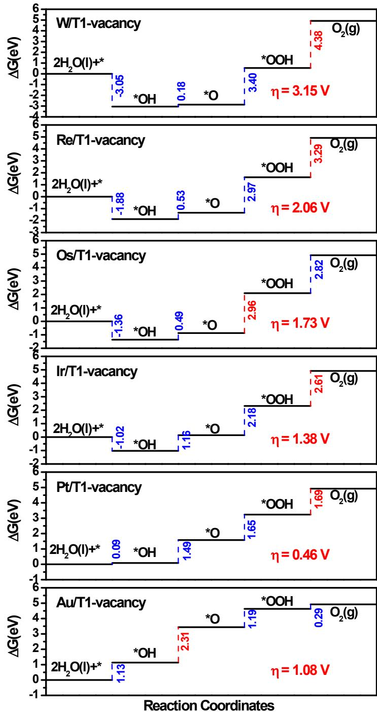
**Figure S8** Free energy diagram for 5d single TM atom doped T1-vacancy term for OER, where the elementary reaction with  $\Delta G$  in red shows the potential-determining step.
