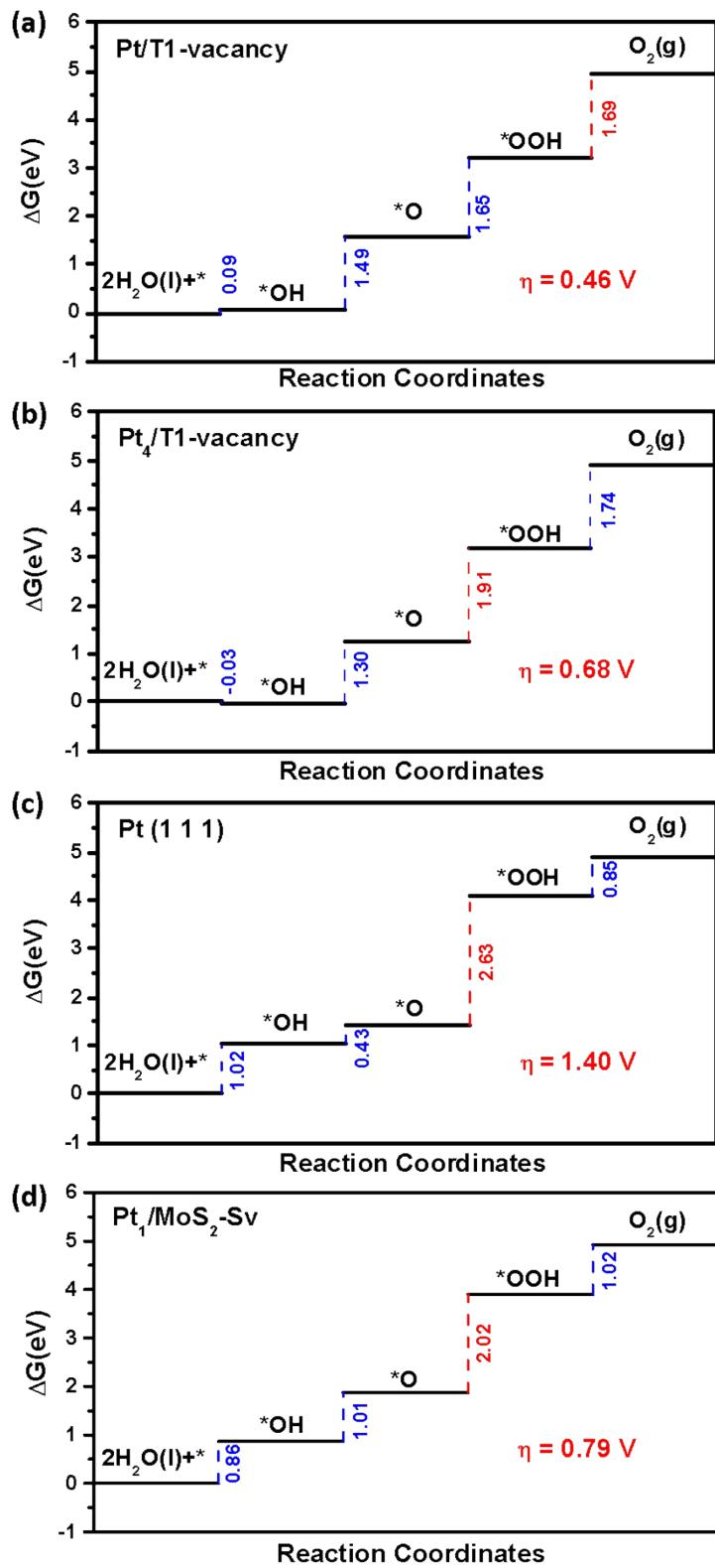
**Figure S14** Free energy diagram for OER on (a) Pt/T1-vacancy, (b)  $\text{Pt}_4/\text{T1-vacancy}$ , (c)  $\text{Pt}(111)$  surface and (d)  $\text{Pt}_1/\text{MoS}_2\text{-Sv}$ , where the elementary reaction with  $\Delta G$  in red shows the potential-determining step.
