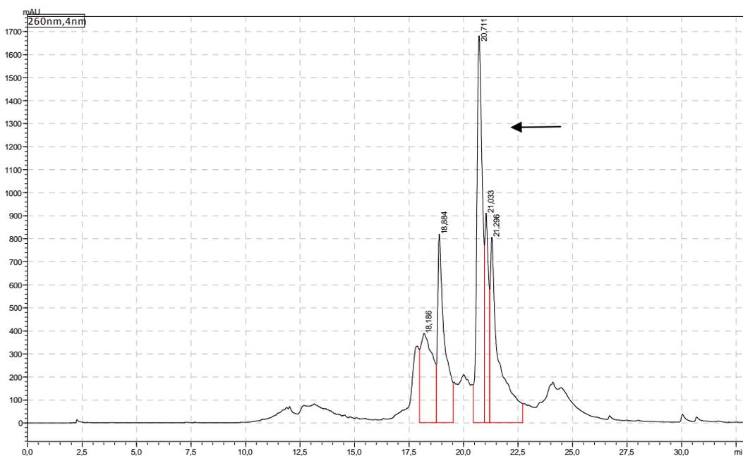
**Figure S2B.** RP HPLC profile of crude "trityl on" triped **5** (the peak of the collected material indicated by arrow). RP-HPLC conditions were as follow: the buffer A (0.1M  $\text{CH}_3\text{COONH}_4$ ) and buffer B (100%  $\text{CH}_3\text{CN}$ ). The buffer B gradient was as follows: 0→2 min 0%; 2→25 min 0-45%; 25→28 min 45-60%; 28→30 min 60-0%; 30→33 min 0%.
