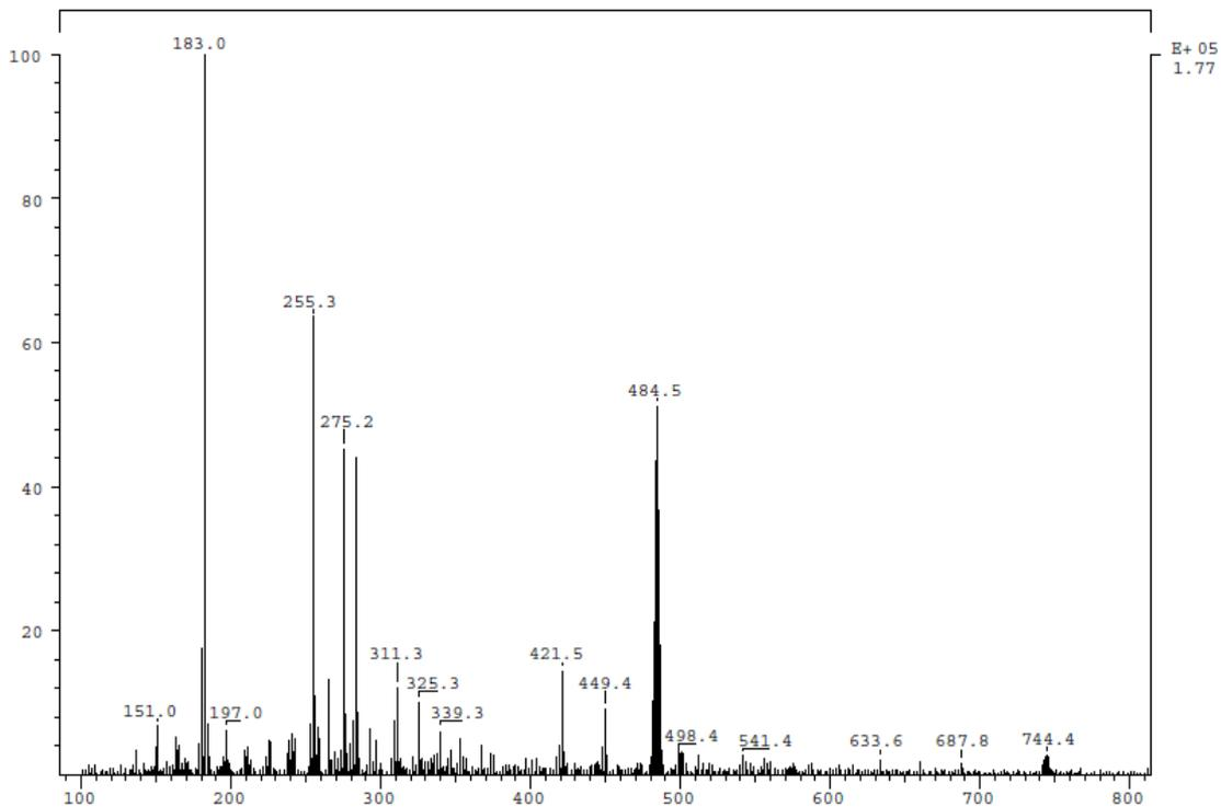
**Figure S13.** MS (FAB): spectrum of 9,12-di(3-O-tritylprop-1-yl)-1,2-dicarba-closo-dodecaborane (**5a**).
