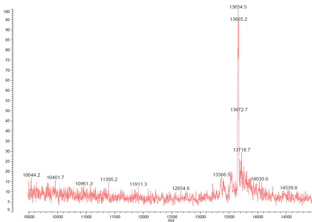
**Figure S3B.** MALDI - TOF mass spectrometry analysis of triped **4**. M.W. calc: 13652.35;  $m/z$ : 13654.5.
