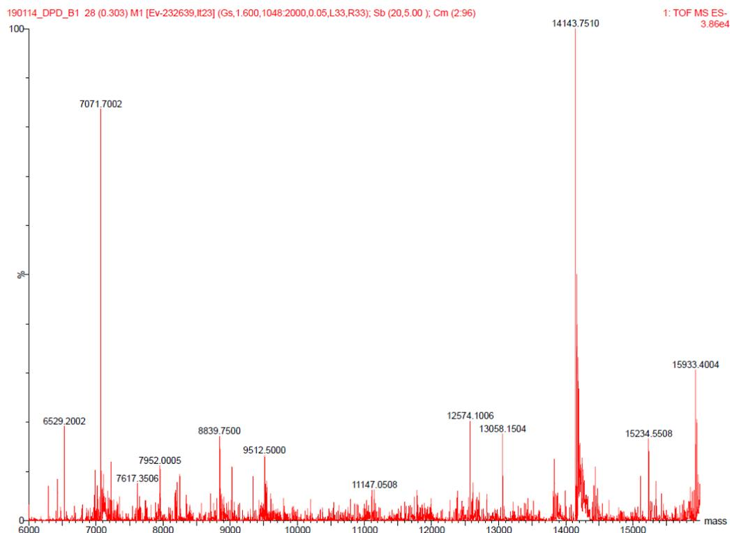
**Figure S3C.** ESI-Q-TOF mass spectrometry analysis of triped **5**. M.W. calc: 14143.31;  $m/z$ : 14143.7510.
