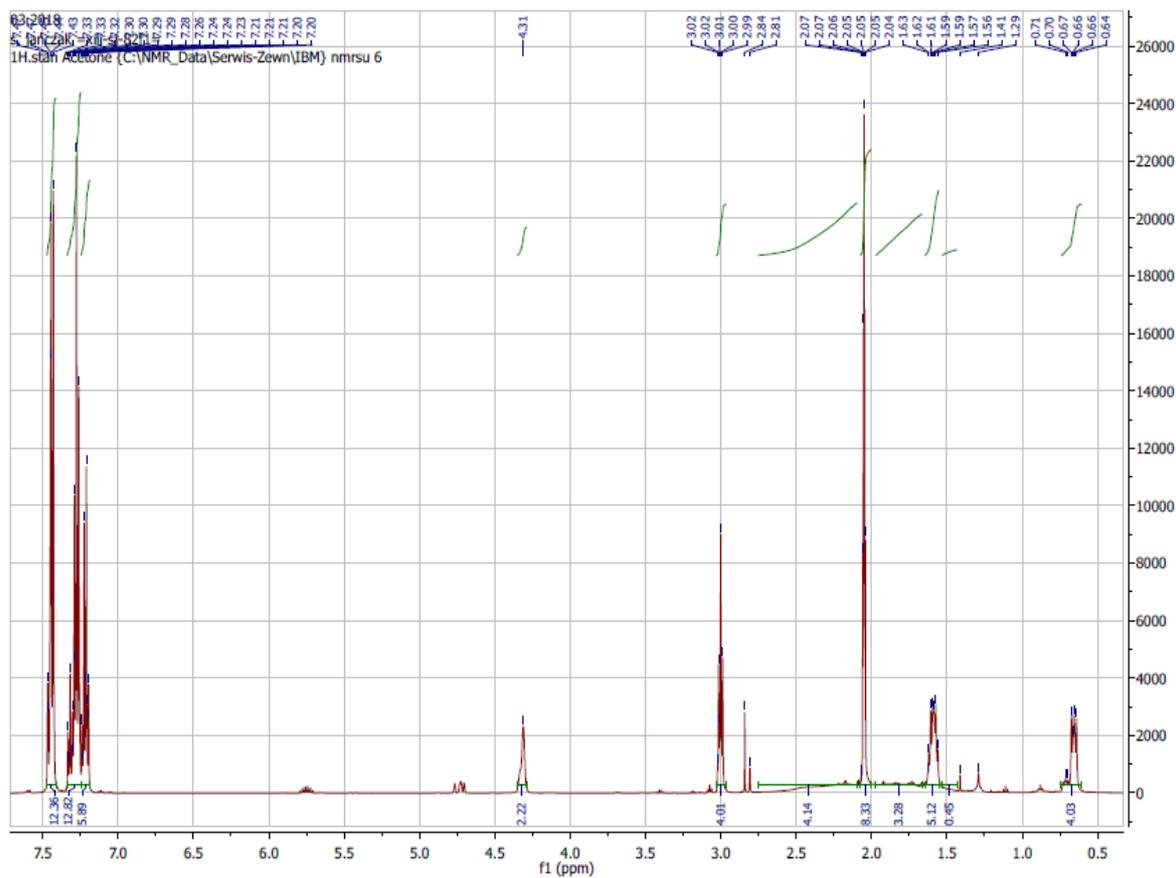
**Figure S12.**  $^1\text{H}$  NMR (acetone- $d_6$ , 600 MHz, 25°C, TMS) spectrum of 9,12-di(3-O-tritylprop-1-yl)-1,2-dicarba-*closo*-dodecaborane (**5a**).
