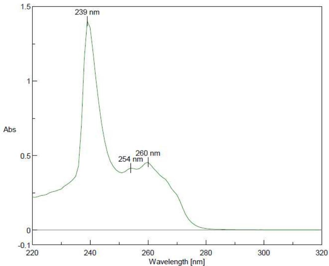
Figure S6. UV-Vis spectrum of 3-bromo-1-trityloxypropane (2a).
