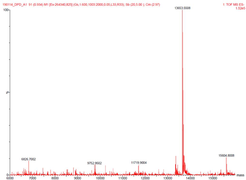
**Figure S3A.** ESI-Q-TOF mass spectrometry analysis of triped **4**. M.W. calc: 13652.35;  $m/z$ : 13653.5508.
