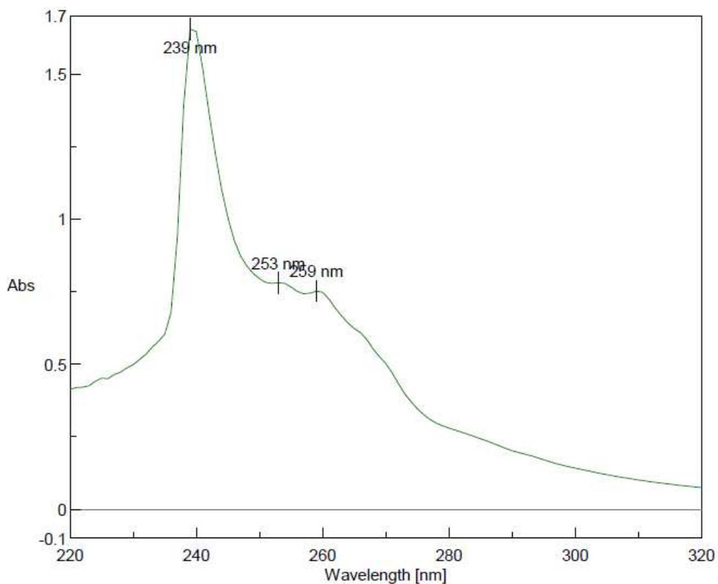
**Figure S10.** UV-Vis spectrum of 9,12-di(3-O-tritylprop-1-yl)-1,2-dicarba-*c*loso-dodecaborane (5a).
