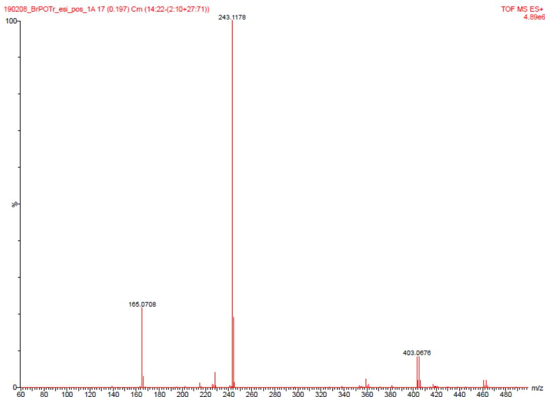
**Figure S9.** HRMS: spectrum of 3-bromo-1-trityloxypropane (**2a**).
