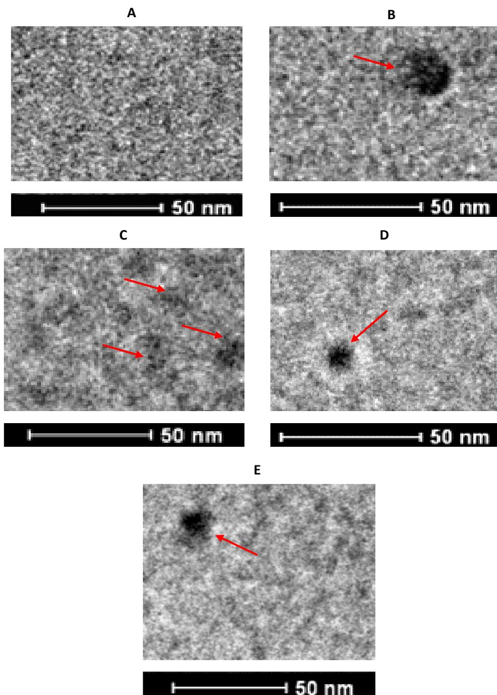
**Figure S5.** The cryo-TEM images: A) buffer (20 mM Tris-HCl pH 8, 10 mM MgCl<sub>2</sub>, 50 mM NaCl), B) boron clusters (C<sub>2</sub>B<sub>10</sub>H<sub>12</sub>) aggregate, C) duplex **2/3**, D) aggregates of single stranded tripeds **4** and E) **5**, (16 times enlarged images from Figures S4A-E, respectively, scale bar: 50 nm). Red arrows show the individual structures.
