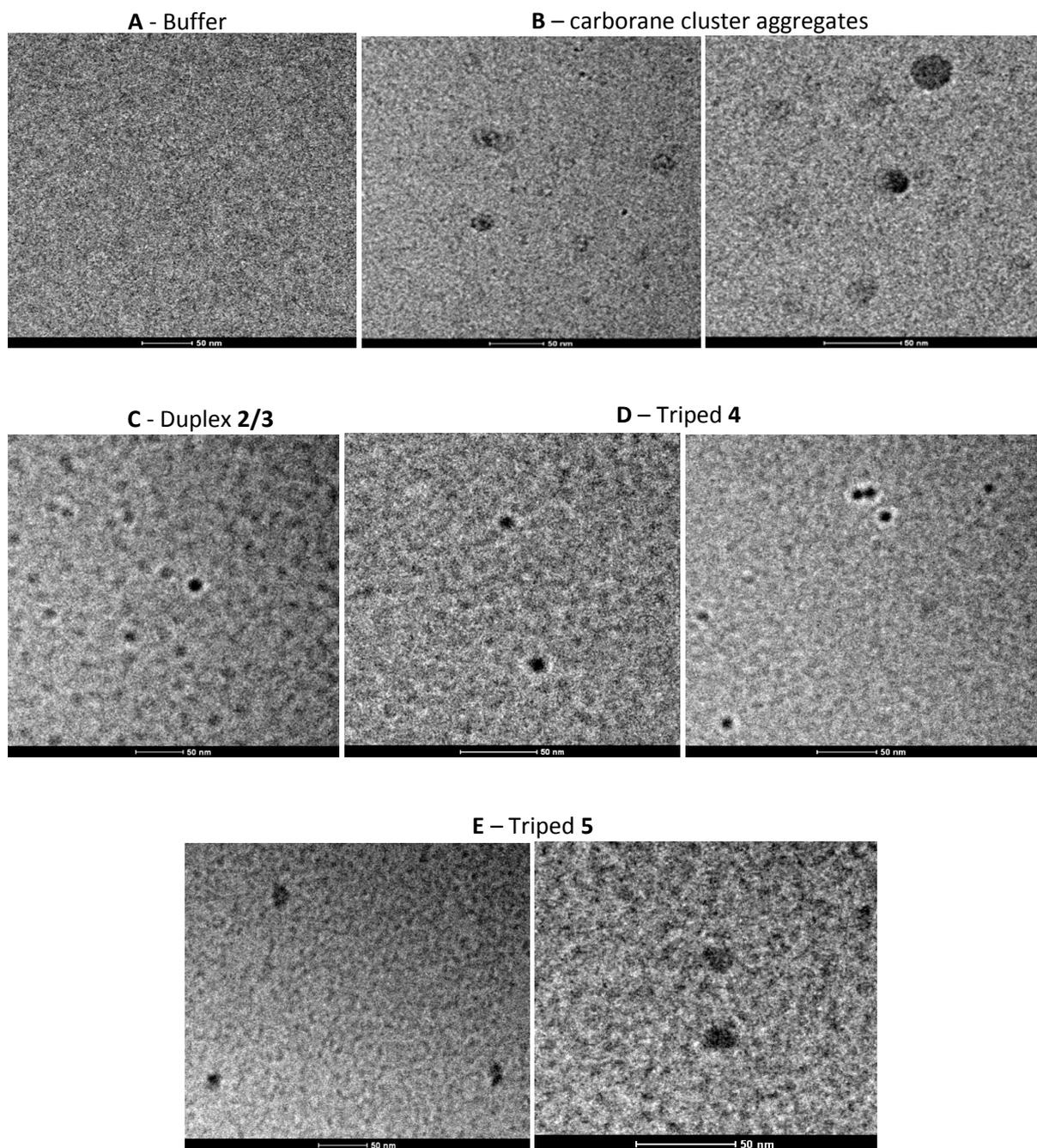
**Figure S4.** The cryo-TEM images: A) buffer (20 mM Tris-HCl pH 8, 10 mM MgCl<sub>2</sub>, 50 mM NaCl), B) 1,2-dicarbha-*closo*-dodecaborane cluster (C<sub>2</sub>B<sub>10</sub>H<sub>12</sub>) aggregate, C) duplex **2/3**, D) single stranded triped **4** and E) single stranded triped **5**. Images are shown on a scale 50 nm.
