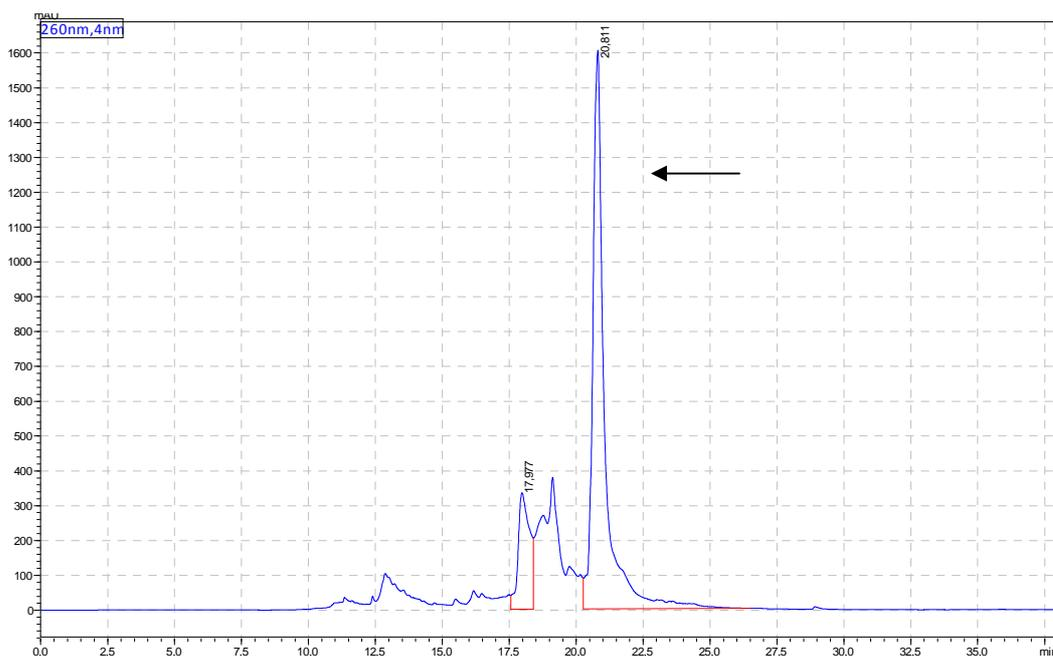
**Figure S2A.** RP HPLC profile of crude "trityl on" triped **4** (the peak of the collected material indicated by arrow). RP-HPLC conditions were as follow: the buffer A (0.1 M  $\text{CH}_3\text{COONH}_4$ ) and buffer B (100%  $\text{CH}_3\text{CN}$ ). The buffer B gradient: 0→2 min 0%; 2→21 min 0-40%; 21→24 min 40-45%; 24→28 min 45-0%; 28→32 min 0%.
