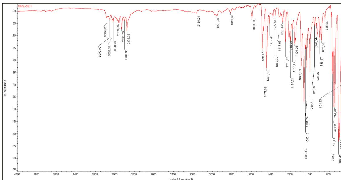
Figure S7. ATR IR (cm<sup>-1</sup>): spectrum of 3-bromo-1-trityloxypropane (2a).
