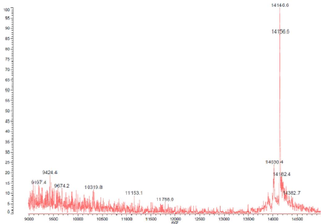
**Figure S3D.** MALDI-TOF mass spectrometry analysis of triped **5**. M.W. calc: 14143.31;  $m/z$ :14146.6.
