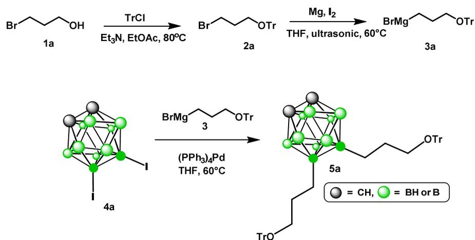
**Scheme S1.** Synthesis of 9,12-bis(3-O-tritylprop-1-yl)-1,2-dicarba-*closo*-dodecaborane (**5a**)
