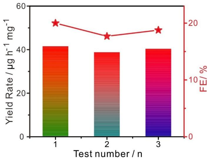
**Figure S7.**  $\text{NH}_3$  yields and FE of different test numbers at -0.3 V in 0.1 M HCl after 1 h of electrolysis.
