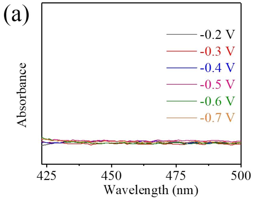
**Figure S14** UV-Vis adsorption spectra of the 0.1 M HCl electrolytes after 1 h electrolysis in N<sub>2</sub> saturated solution at various potentials.
