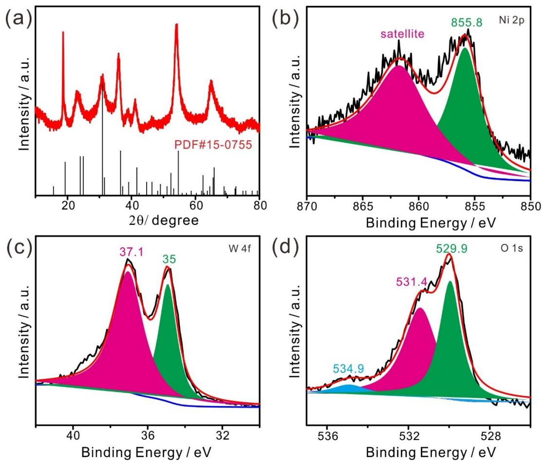
**Figure S8.** (a) XRD pattern of  $\text{NiWO}_4$  after long-term stability measurement in 0.1 M HCl. High-resolution XPS spectra of Ni 2p (b), W 4f (c) and O 1s (d) after durability test.
