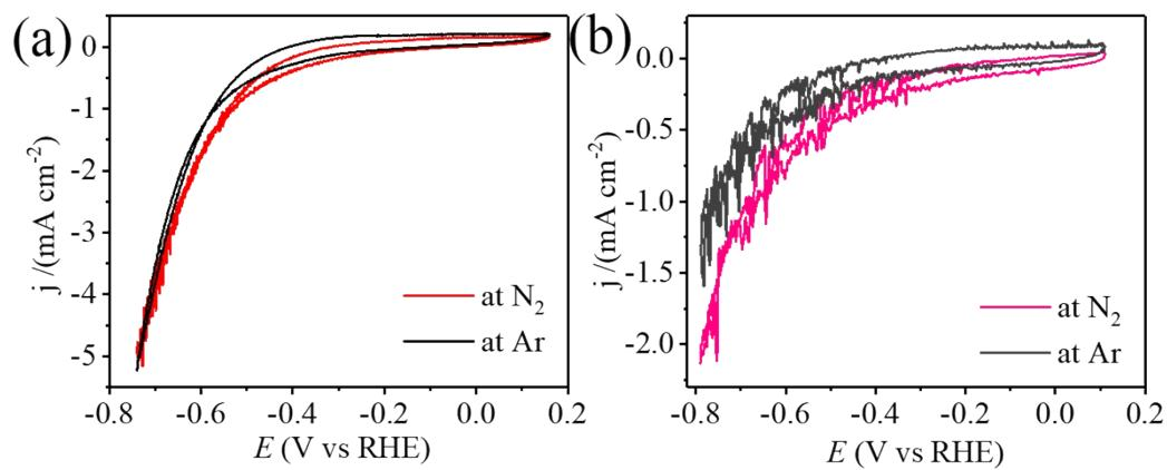
**Figure S11** CV of  $\text{NiWO}_4$  at  $\text{N}_2$  or Ar in 0.1 M HCl (a) and 0.1 M  $\text{Na}_2\text{SO}_4$  (b).
