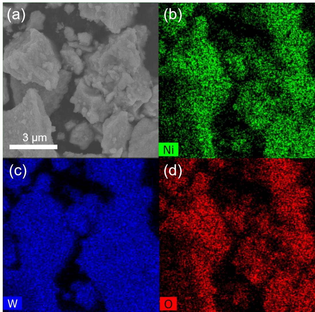
**Figure S1.** SEM image of NiWO<sub>4</sub> (a) and corresponding EDX mappings of Ni (b), W (c) and O (d).
