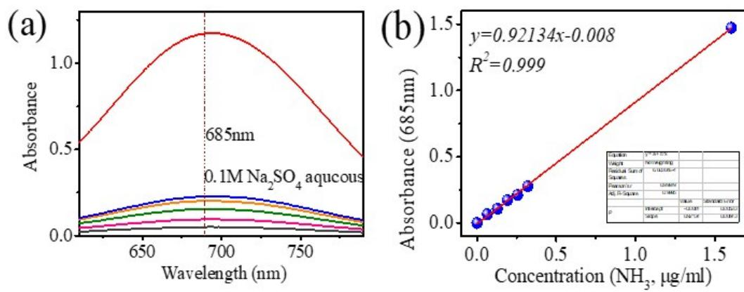
**Figure S6.** (a) UV-Vis absorption spectra of various  $\text{NH}_3$  concentrations after incubated for 1h at room temperature. (b) Calibration curve used for estimation of  $\text{NH}_3$ .
