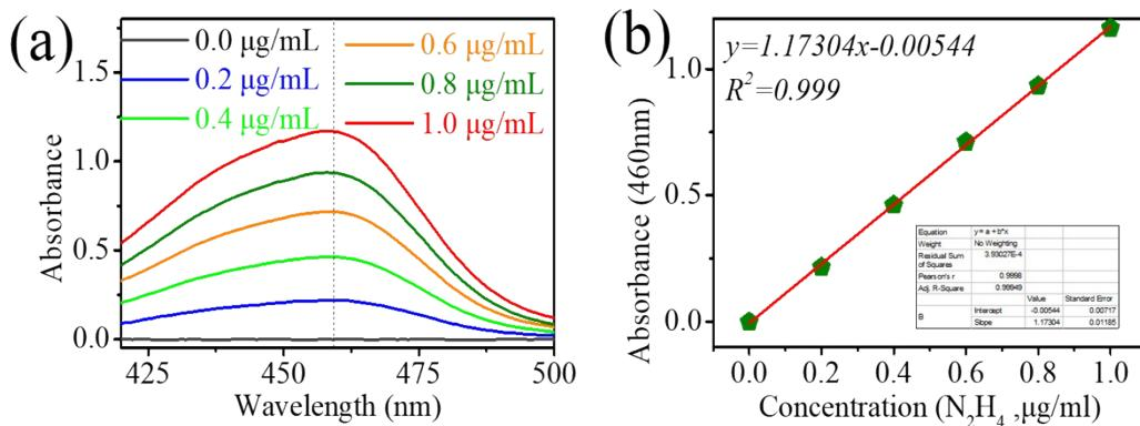
**Figure S3.** (a) UV-Vis absorption spectra of various  $\text{N}_2\text{H}_4$  concentrations after incubated for 10 min at room temperature. (b) Calibration curve used for calculation of  $\text{N}_2\text{H}_4$  concentrations.
