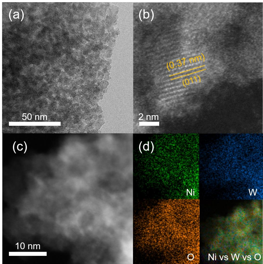
**Figure S10** TEM image of  $\text{NiWO}_4$  after stability measurement in 0.1 M HCl (a), (b), (c)and corresponding EDS mappings of Ni, W and O.
