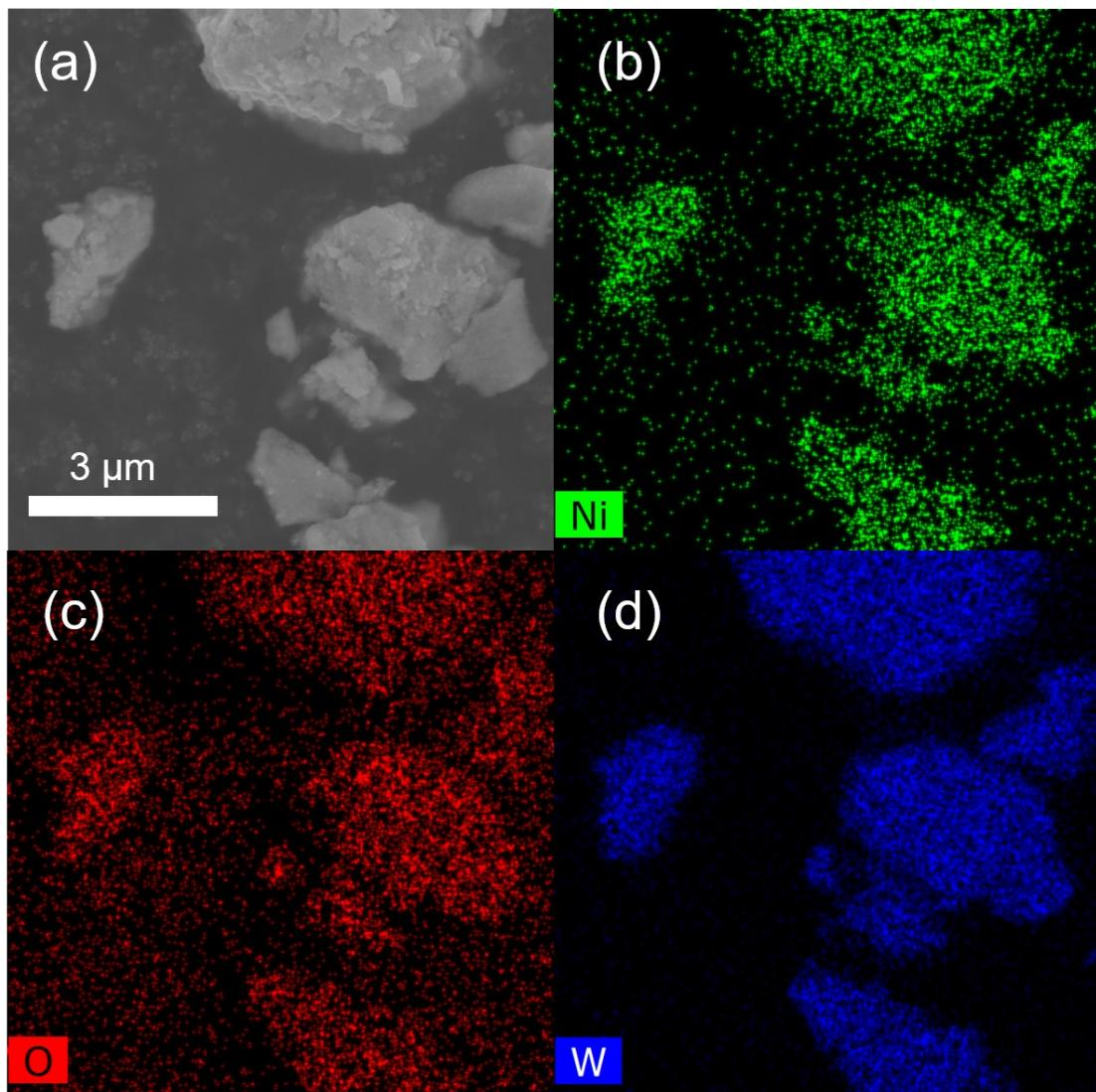
**Figure S9.** SEM image of NiWO<sub>4</sub> after stability measurement in 0.1 M HCl (a) and corresponding EDS mappings of Ni (b), W (c) and O (d).
