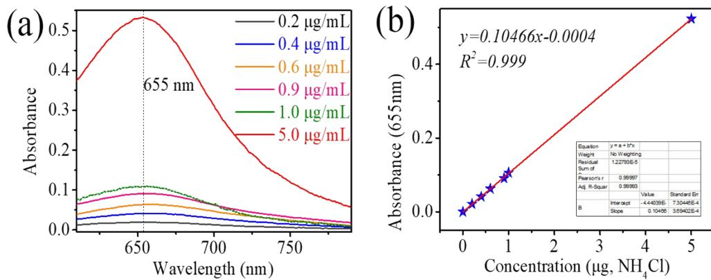
**Figure S2.** (a) UV-Vis absorption spectra of indophenol assays with  $\text{NH}_4^+$  after incubated for 2 h at room temperature. (b) Calibration curve used for estimation of  $\text{NH}_4\text{Cl}$ .
