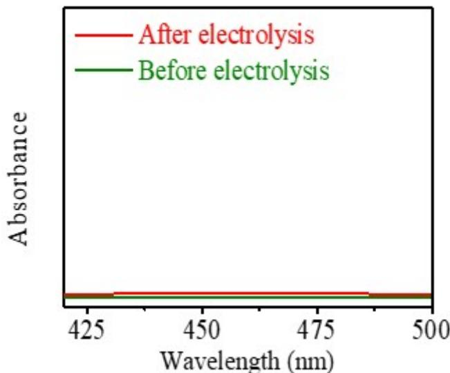
**Figure S4.** UV-Vis absorption spectra of the 0.1 M HCl electrolyte (after charging at  $-0.3$  V vs. RHE for 1 h) after incubated for 10 min at room temperature.
