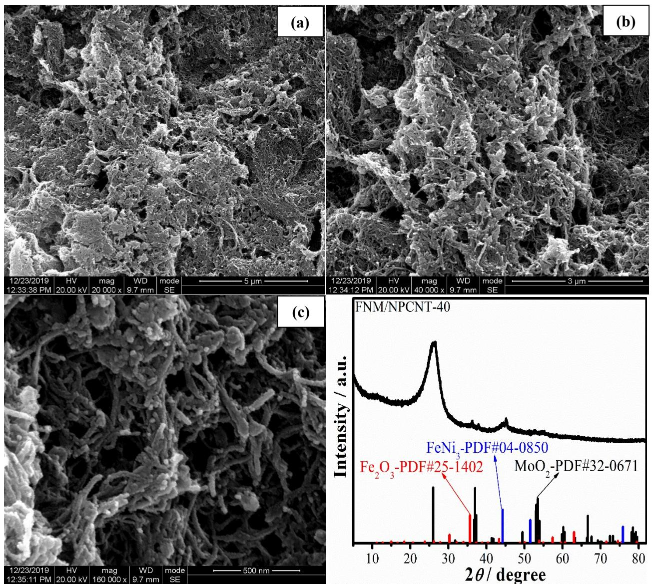
**Fig. S4** SEM (a, b, c) and XRD (d) of FNM/NPCNT-40 hybrid after 2000 CV treatment in KOH medium.
