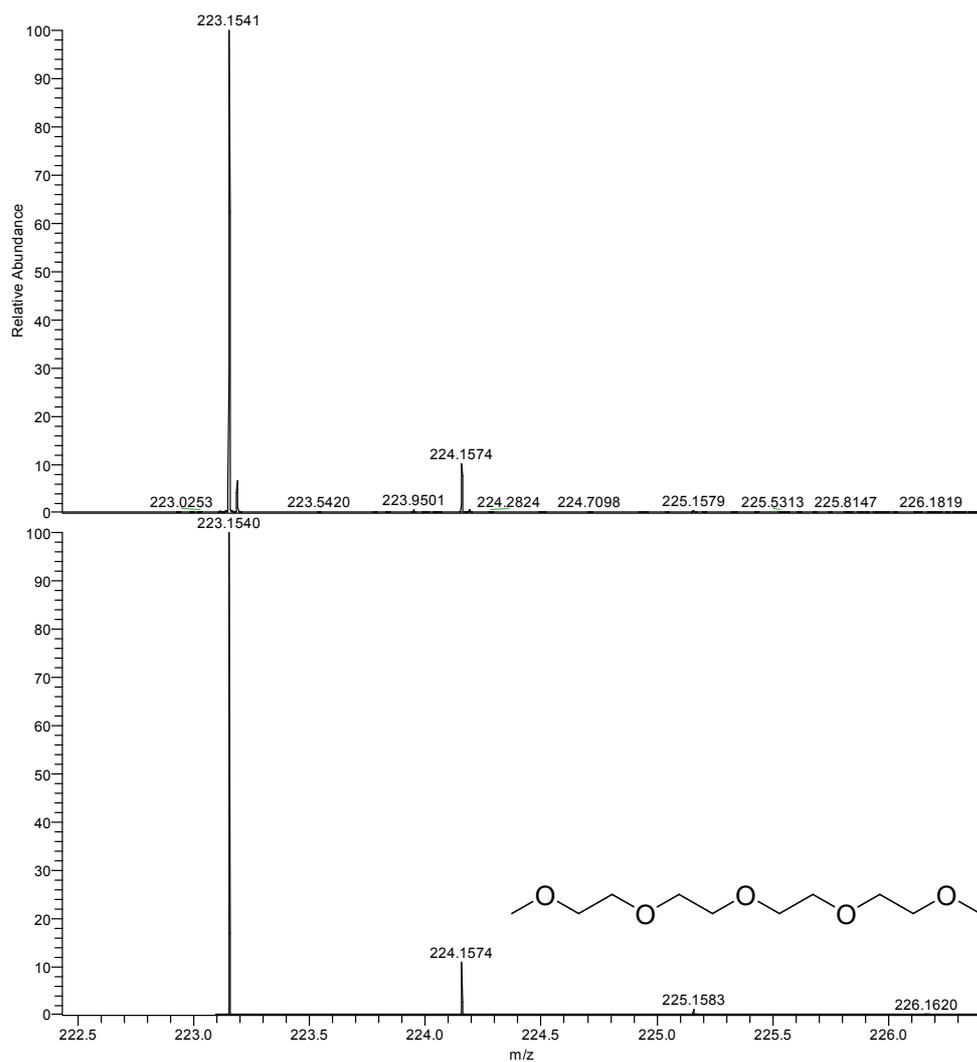
**Figure S21.** A zoomed in version of the high resolution mass spectrum shown in Figure S18 above of the reaction mixture from the reaction between 1-fluoro-2,4-dinitrobenzene **6**, triethylamine and  $[\text{Li}(\text{G4})][\text{N}(\text{SO}_2\text{CF}_3)_2]$  **2**. The predominate signal shown at  $m/z$  223.1540 corresponds to an elemental composition of  $\text{C}_{10}\text{H}_{23}\text{O}_5$  corresponding to the protonated form of the tetraglyme.
