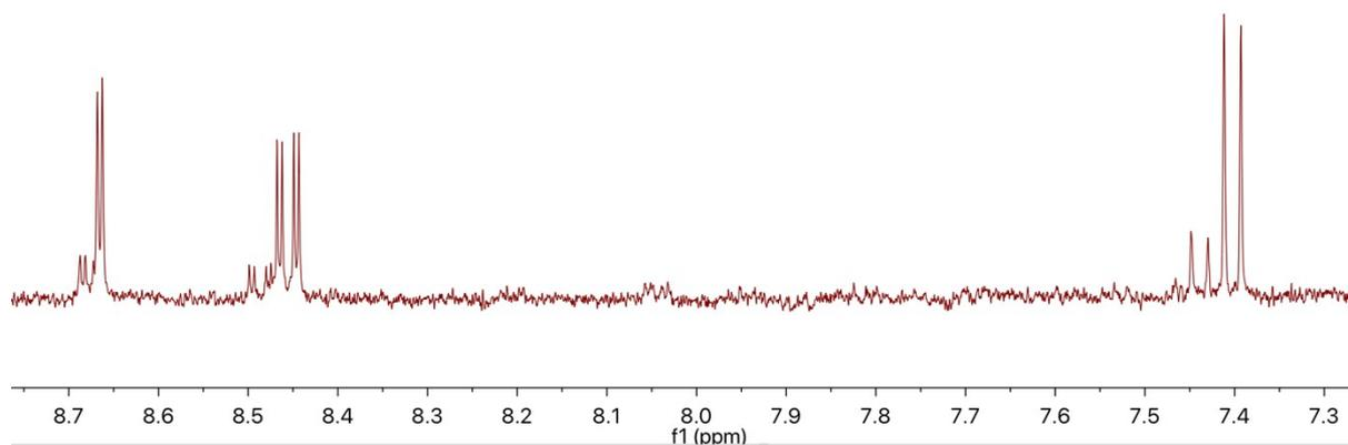
**Figure S22.** A section of the <sup>1</sup>H NMR spectrum of a reaction mixture typical of a kinetic run in [Li(G4)][N(SO<sub>2</sub>CF<sub>3</sub>)<sub>2</sub>] **2** ( $\chi_{IL}$  *ca.* 0.8) after heating at 55 °C for 16 h except that the fluoride scavenger methoxytrimethylsilane had been added. The smaller signals downfield from each signal representing the expected product, 2,4-dinitrophenetole **8**, are those of 1-methoxy-2,4-dinitrobenzene.
