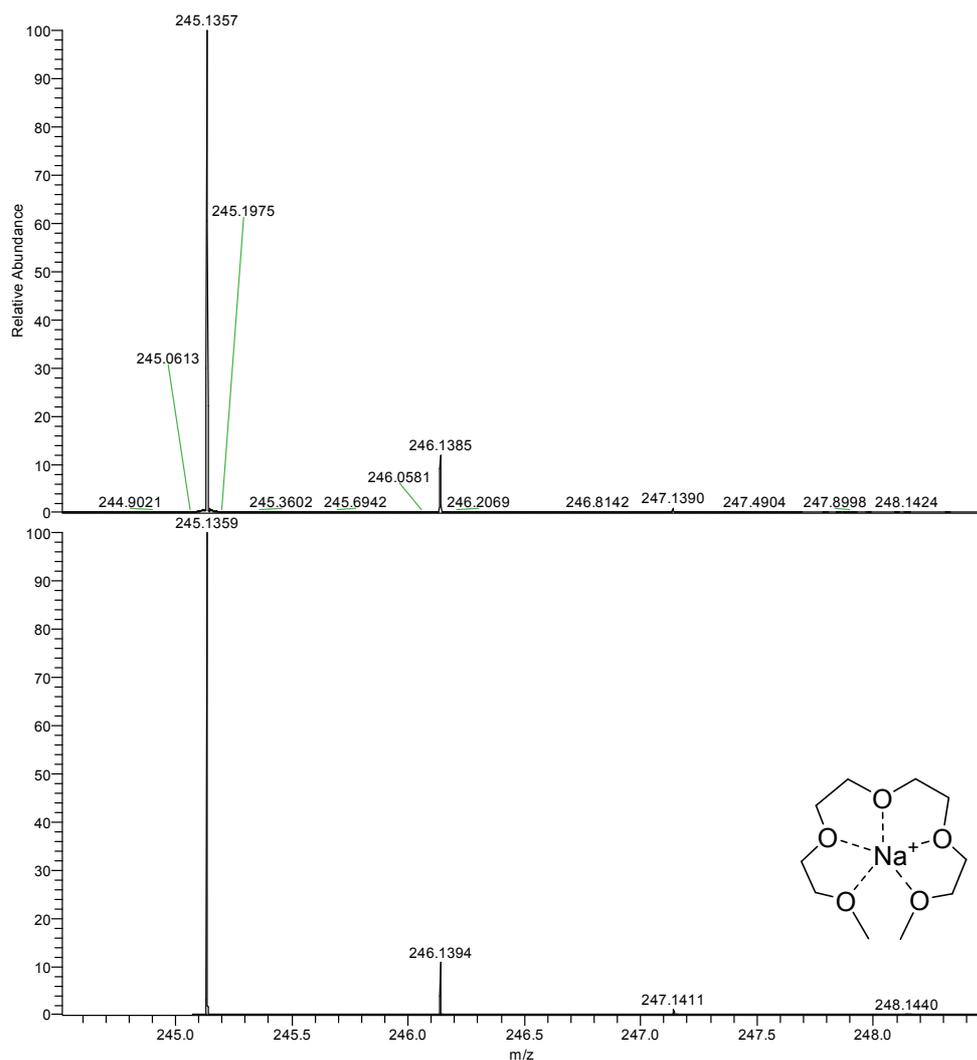
**Figure S15.** A zoomed in version of the high resolution mass spectrum shown in Figure S14 above of the reaction mixture from the reaction between 1-fluoro-2,4-dinitrobenzene **6**, triethylamine and tetraglyme. The predominate signal shown at  $m/z$  245.1359 corresponds to an elemental composition of  $C_{10}H_{22}O_5Na$ ; the sodiated form of the tetraglyme starting material.
