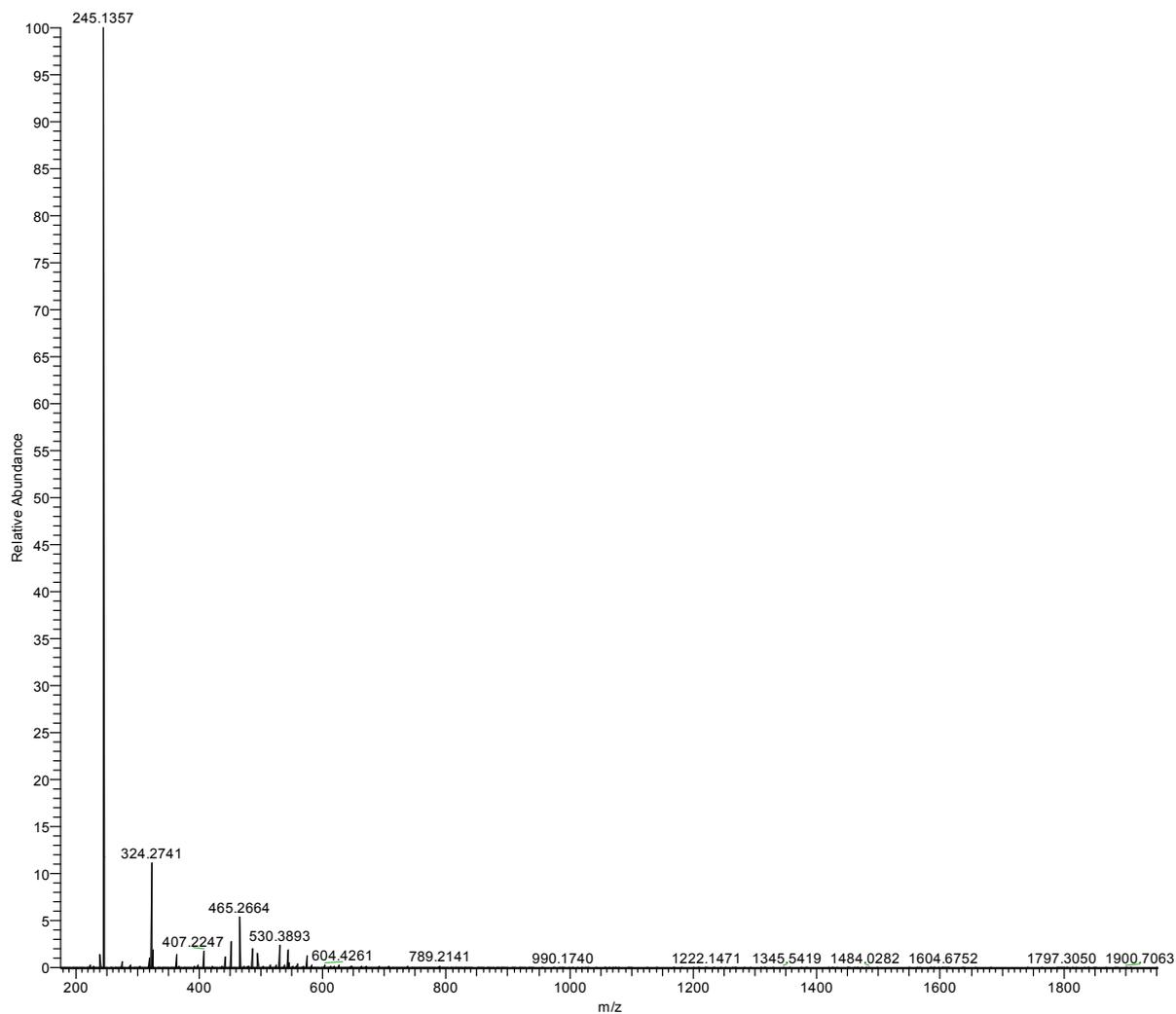
**Figure S14.** The high resolution mass spectrum of the reaction mixture from the reaction between 1-fluoro-2,4-dinitrobenzene **6**, triethylamine and tetraglyme.
