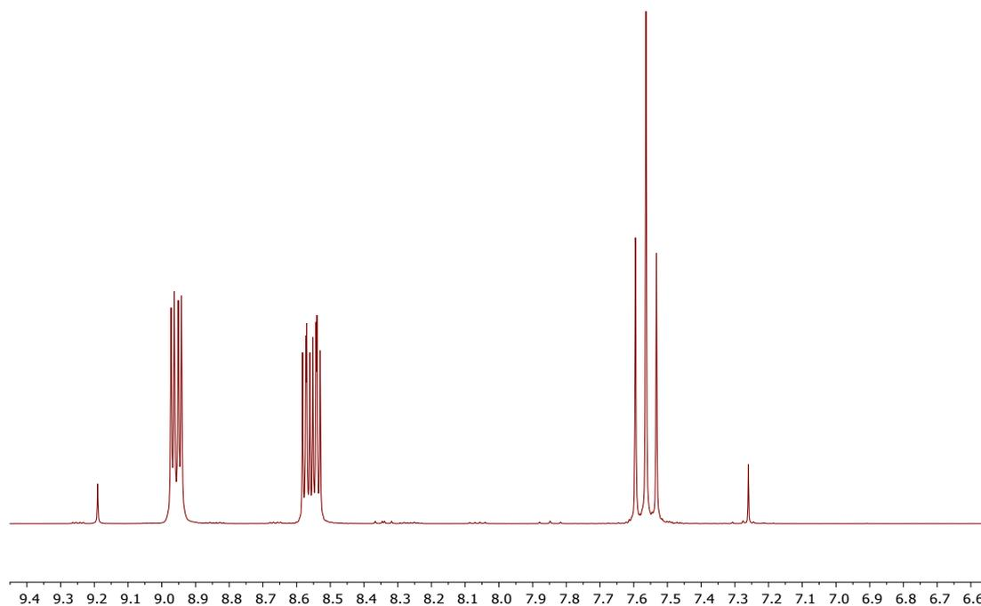
**Figure S4** A <sup>1</sup>H NMR spectrum of 1-fluoro-2,4-dinitrobenzene **6** in CDCl<sub>3</sub>.
