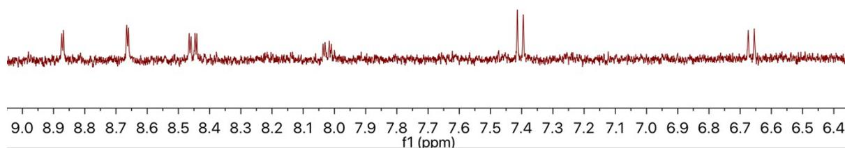
**Figure S23.** A section of the <sup>1</sup>H NMR spectrum of a reaction mixture of [Li(G4)][N(SO<sub>2</sub>CF<sub>3</sub>)<sub>2</sub>] **2**, tetrabutylammonium fluoride, 1-fluoro-2,4-dinitrobenzene **6**, ethanol and triethylamine after heating at 55 °C for 24 h.
