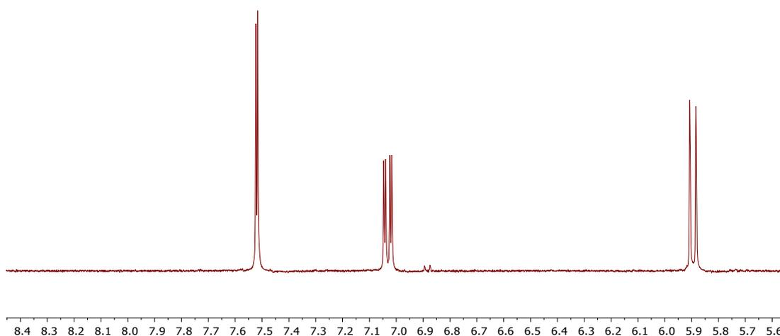
**Figure S7 A** <sup>1</sup>H NMR spectrum of 2,4-dinitrophenol in CD<sub>3</sub>CN.
