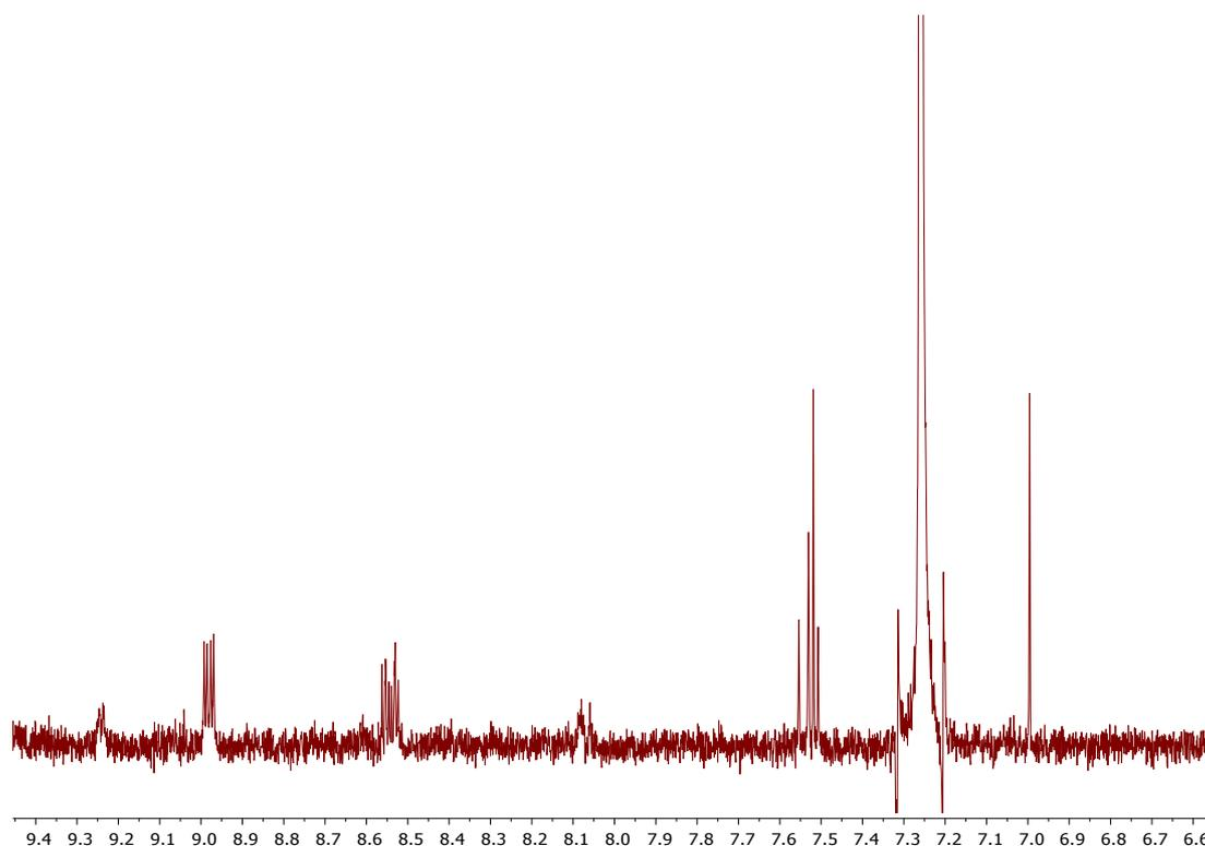
**Figure S13.** A <sup>1</sup>H NMR spectrum of a reaction mixture containing 1-fluoro-2,4-dinitrobenzene **6**, triethylamine and tetraglyme in acetonitrile after stirring at room temperature overnight, followed by heating at 55 °C for 4 h. Residual solvent signal at 7.26 ppm due to CDCl<sub>3</sub>.
