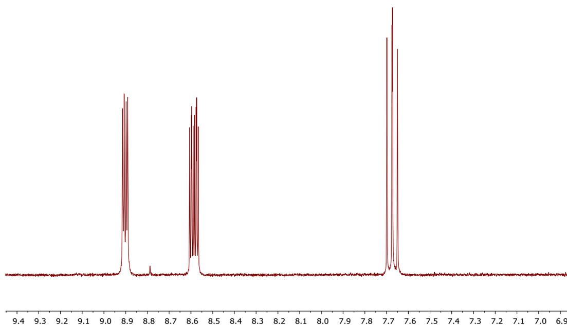
**Figure S16.** A section of the <sup>1</sup>H NMR spectrum of a reaction mixture containing 1-fluoro-2,4-dinitrobenzene **6** and [Li(G4)][N(SO<sub>2</sub>CF<sub>3</sub>)<sub>2</sub>] **2** after stirring at room temperature overnight, followed by heating at 55 °C for 4 h.
