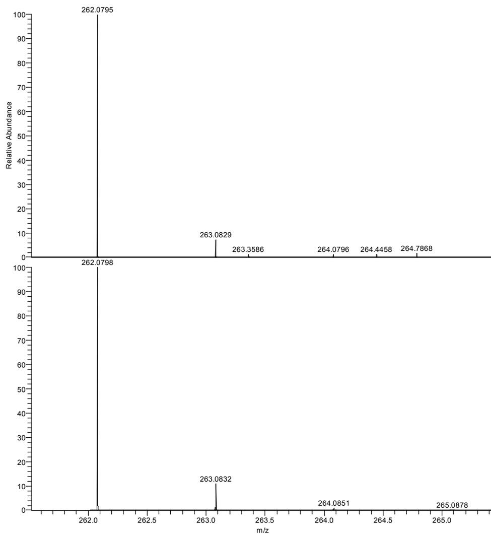
**Figure S12.** A zoomed in version of the high resolution mass spectrum presented above in Figure S11 of the reaction mixture from the reaction between 1-fluoro-2,4-dinitrobenzene **6** and triethylamine in acetonitrile. The predominate signal at  $m/z$  262.0795 corresponds to an elemental composition of  $C_{10}H_{13}N_3O_4Na$ ; the sodiated form of *N,N*-diethyl-2,4-dinitroaniline.
