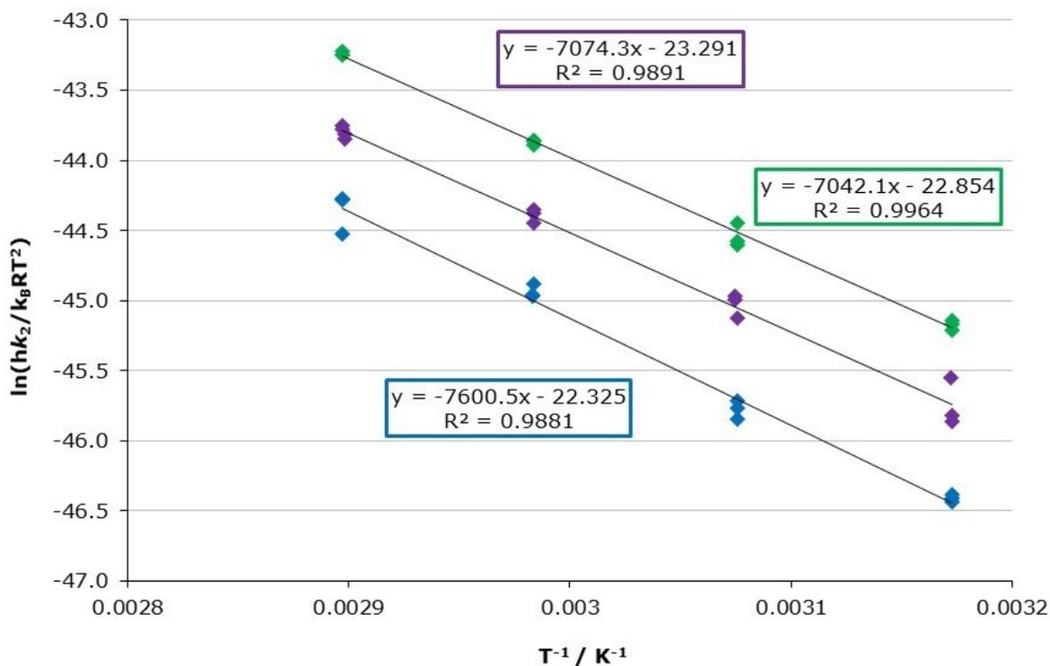
**Figure S1** Eyring plots for the reaction between pyridine **4** and benzyl bromide **5** in [Li(G3)][N(SO<sub>2</sub>CF<sub>3</sub>)<sub>2</sub>] **1** ( $\chi_1 \approx 0.83$ , purple), [Li(G4)][N(SO<sub>2</sub>CF<sub>3</sub>)<sub>2</sub>] **2** ( $\chi_2 \approx 0.82$ , green) and Li[N(SO<sub>2</sub>CF<sub>3</sub>)<sub>2</sub>] ( $\chi_{\text{salt}} \approx 0.20$ , blue).
