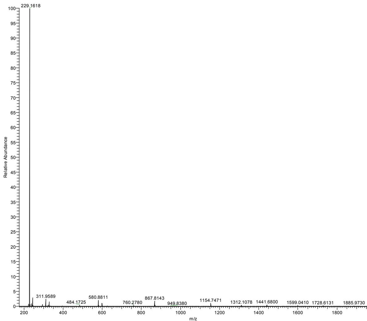
**Figure S18.** The high resolution mass spectrum of the reaction mixture from the reaction between 1-fluoro-2,4-dinitrobenzene **6**, triethylamine and  $[\text{Li}(\text{G4})][\text{N}(\text{SO}_2\text{CF}_3)_2]$  **2**.
