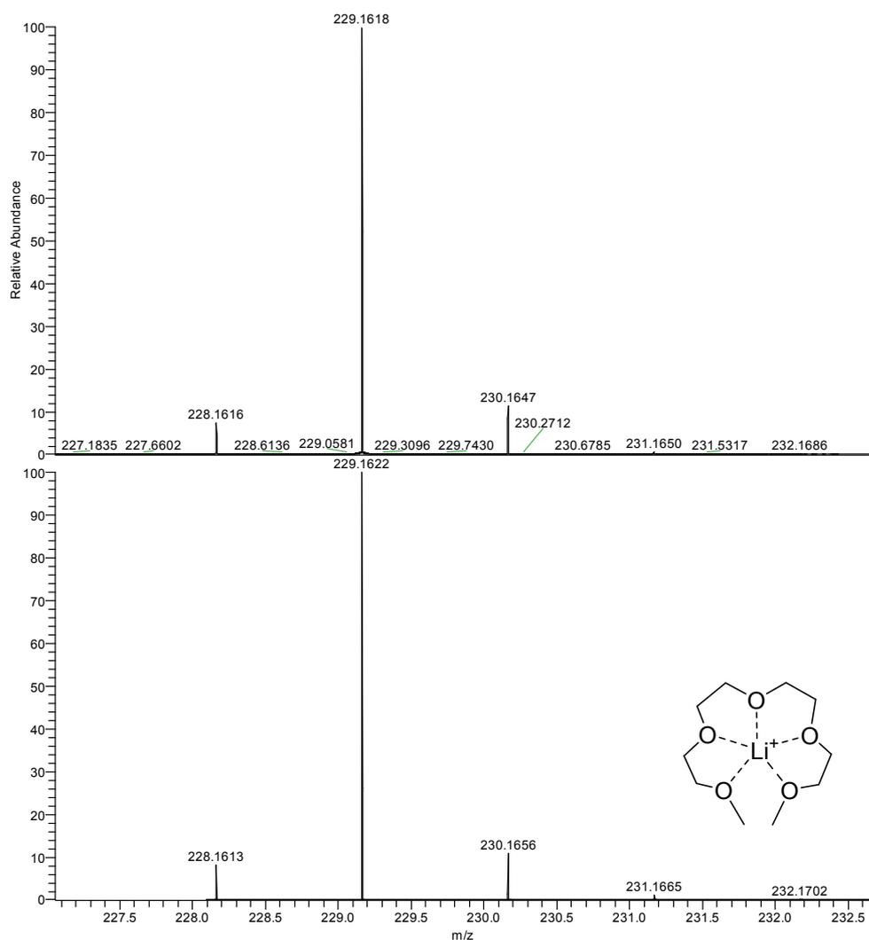
**Figure S19.** A zoomed in version of the high resolution mass spectrum shown in Figure S18 above of the reaction mixture from the reaction between 1-fluoro-2,4-dinitrobenzene **6**, triethylamine and [Li(G4)][N(SO<sub>2</sub>CF<sub>3</sub>)<sub>2</sub>] **2**. The predominate signal shown at  $m/z$  229.1622 corresponds to an elemental composition of C<sub>10</sub>H<sub>22</sub>Li<sub>1</sub>O<sub>5</sub>; the cation of the solvate ionic liquid **2**, [Li(G4)]<sup>+</sup>.
