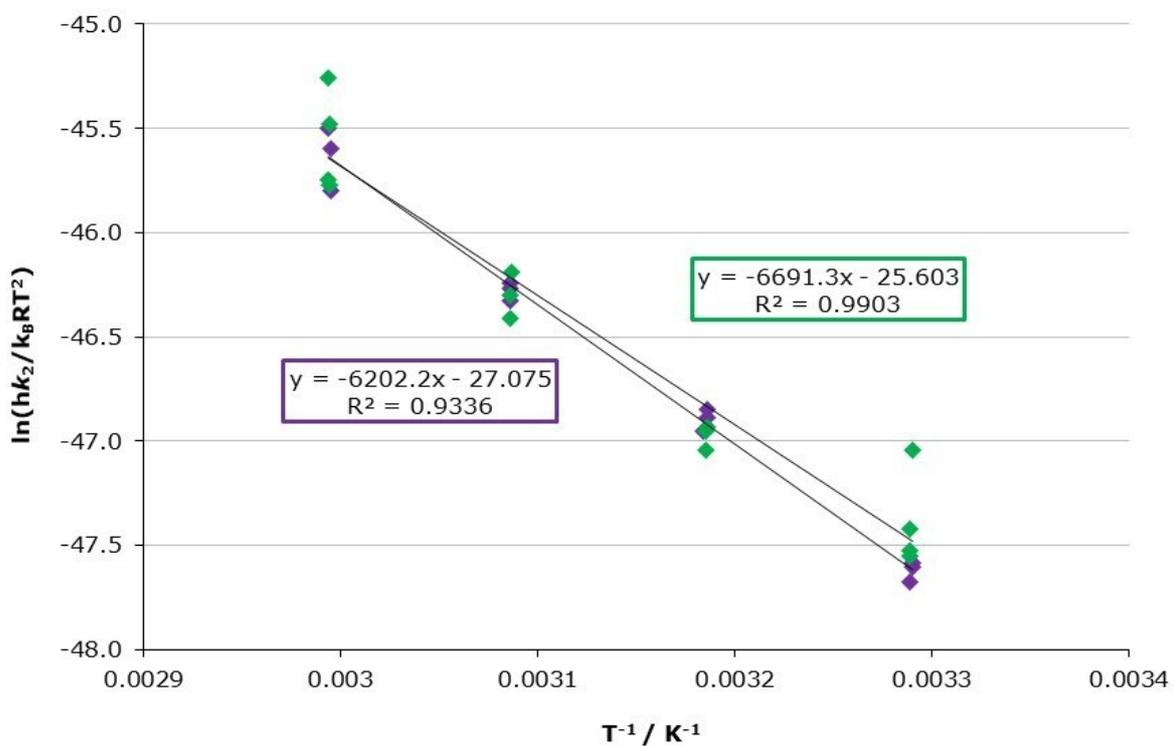
**Figure S3** Eyring plots for the reaction between ethanol and 1-fluoro-2,4-dinitrobenzene **6** in  $[\text{Li}(\text{G}3)][\text{N}(\text{SO}_2\text{CF}_3)_2]$  **1** ( $\chi_1 \approx 0.83$ , purple) and  $[\text{Li}(\text{G}4)][\text{N}(\text{SO}_2\text{CF}_3)_2]$  **2** ( $\chi_2 \approx 0.82$ , green).
