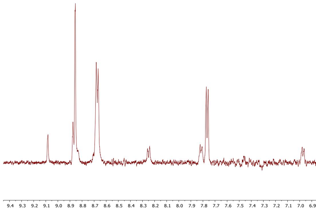
**Figure S6.** A <sup>1</sup>H NMR spectrum of a completed reaction mixture for the reaction between ethanol and 1-fluoro-2,4-dinitrobenzene **6** in [Li(G4)][N(SO<sub>2</sub>CF<sub>3</sub>)<sub>2</sub>] **2** ( $\chi_2 \approx 0.8$ ) diluted with ~ 0.5 mL of ethanol.
