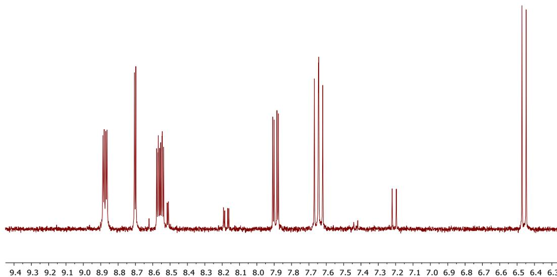
**Figure S10.** A  $^1\text{H}$  NMR spectrum of a reaction mixture containing 1-fluoro-2,4-dinitrobenzene **6** and triethylamine in acetonitrile after stirring at room temperature for a further 48 h.
