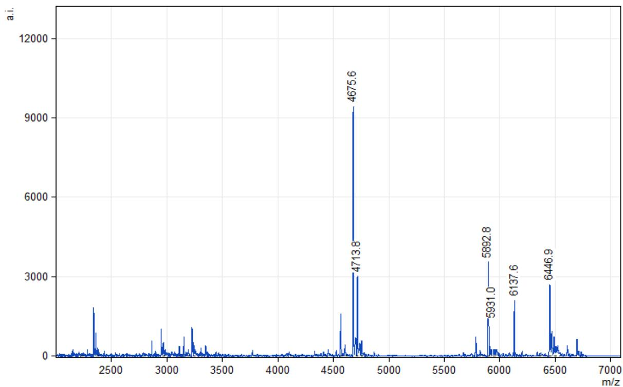
**Figure S14:** MALDI-TOF MS spectrum of **ON19\_1<sup>CM</sup>H** after thiol-ene reaction of **DNA19\_1<sup>V</sup>H** and **CM-SH**, calculated for  $[M+H]^+$ : 6134.9 Da; found: 6137.6. Peak at 5931.0 Da represents the starting vinyl modified DNA, 4675.6 Da is the signal of unreacted primer.
