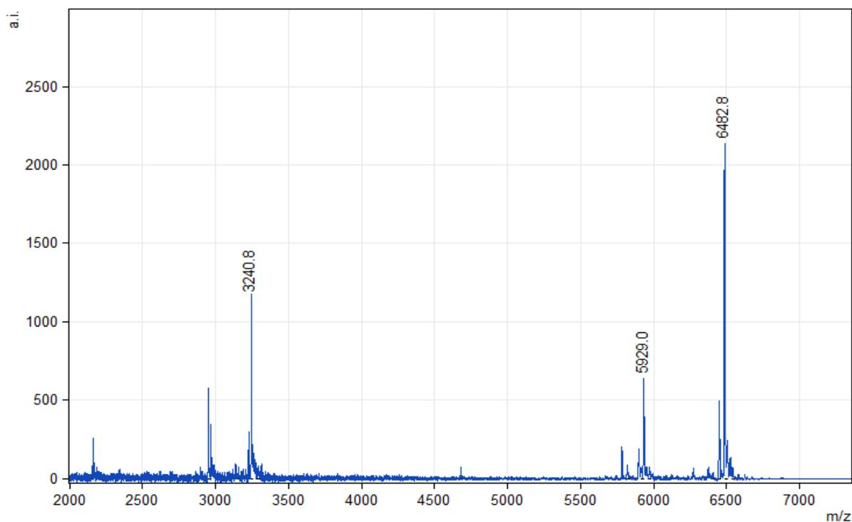
**Figure S11:** MALDI-TOF MS spectrum of **ON19\_1<sup>V</sup>H** after PEX with Temp19-bio and **d<sup>V</sup>ITP**, calculated for  $[M+H]^+$ : 5926.9 Da; found: 5929.0.
