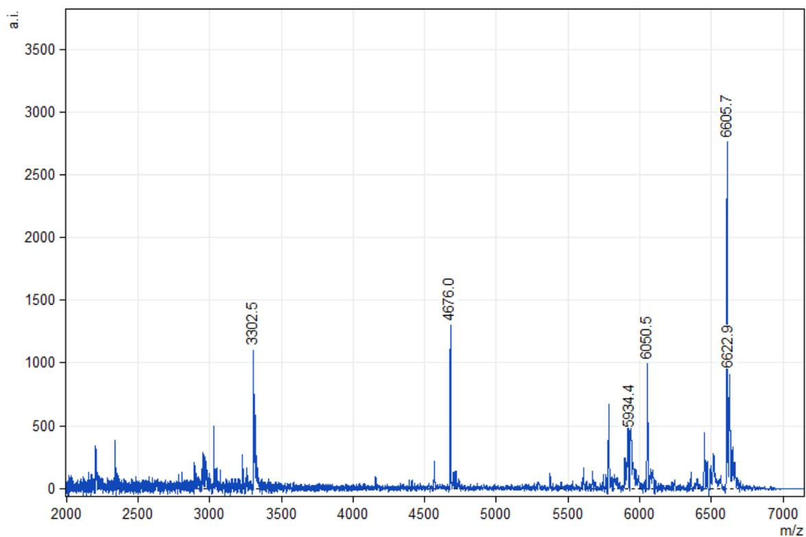
**Figure S16:** MALDI-TOF MS spectrum of **ON19\_1<sup>Cys</sup>H** after thiol-ene reaction of **DNA19\_1<sup>V</sup>H** and **L-cysteine**, calculated for  $[M+H]^+$ : 6049.0 Da; found: 6050.5. Peak at 5934.4 Da represents the starting vinyl modified DNA.
