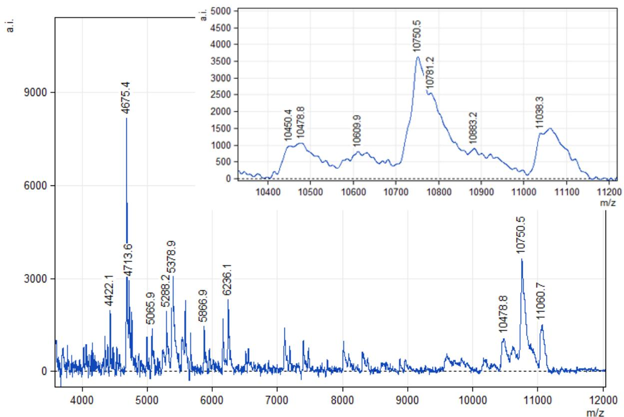
**Figure S15:** MALDI-TOF MS spectrum of **ON31\_4<sup>CM</sup>H** after thiol-ene reaction of **DNA31\_4<sup>V</sup>H** and **CM-SH**. Starting vinyl modified DNA was extended by one or two or three additional As at the 3' end due to non-templated extension. Products of thiol-ene reaction:  $[M+2As+2CM+K]^+$ : 10756.4, found 10750.5 – product of reaction of two vinyl groups,  $[M+3As+2CM+Na]^+$ : 11037.6, found 11038.3, etc.
