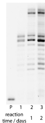
**Figure S7.** Denaturing PAGE showing results of the optimization of the reaction between peptides containing cysteine and vinyl modified DNA (**DNA26\_1<sup>VH</sup>**). Lanes: P: primer; 1: starting **DNA26\_1<sup>VH</sup>**; 2-3: products of reaction of vinyl modified DNA and corresponding **pept\_1-SH** with increased reaction time.
