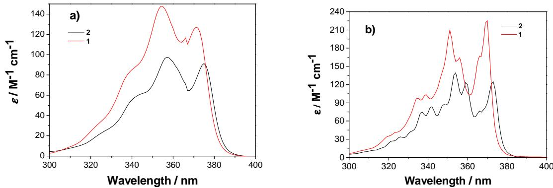
Figure S1. Absorption spectra of **1** and **2** in different solvents: a)  $\text{CH}_3\text{OH}$  and b) cyclohexane.
