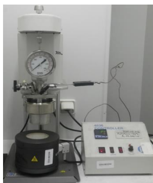
Fig. S5 Hastelloy autoclave Parr System 50 mL, equipped with a Bourdon pressure gauge, a rupture disk, inlet and outlet valves and an electronic device regulated and controlled both the stirring and the heating of the autoclave.
