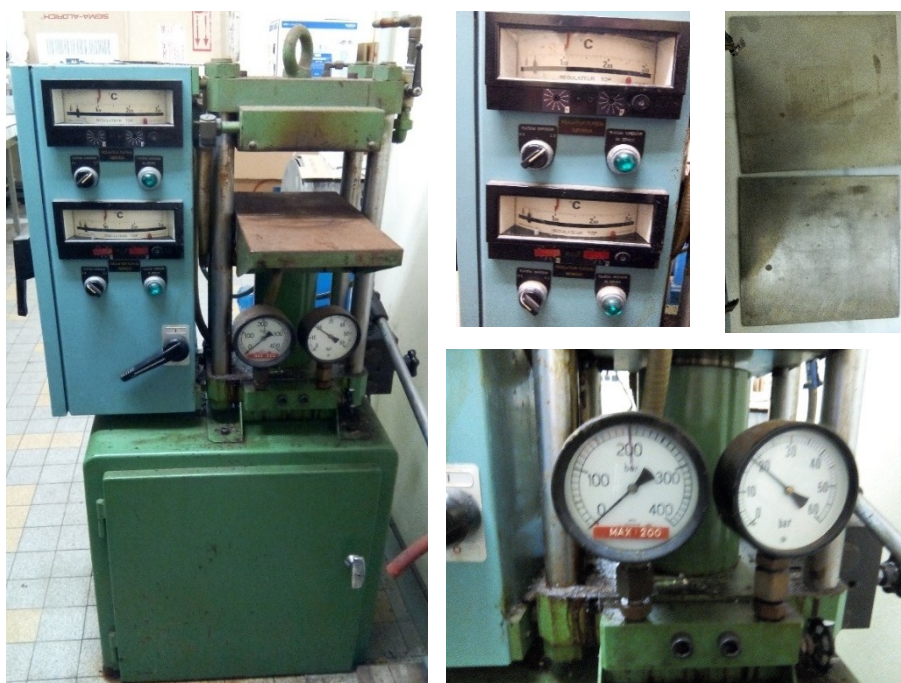
Fig. S6 Press having two independent heating plates ranging from 20 to 300 °C, controlled by a regulator, a hydraulic jack equipped with an oil pressure manometer from 0 to 400 bar and two steel plates.
