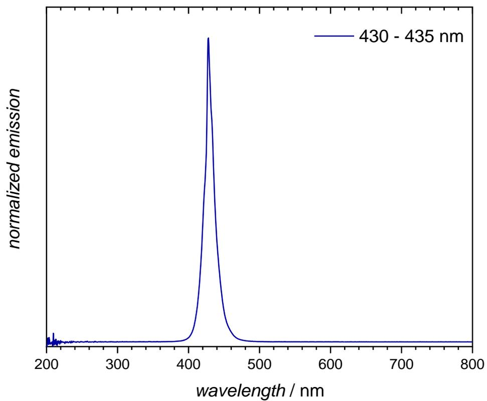
**Figure S6** Emission spectrum of the LED setup employed in the current study.
