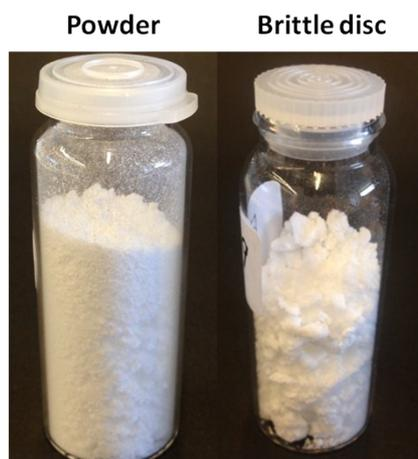
**Figure S2:** Representative products taken straight after depressurisation of the autoclave. The left hand-side is a free flowing powder, the right hand-side is a brittle disc that was chiselled out from the reactor.
