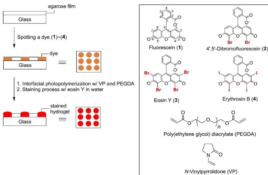
**Fig. S1** Schematic depiction of the procedure for the fabrication of a chip and molecular structure of anionic xanthene dyes, employed in this work.
