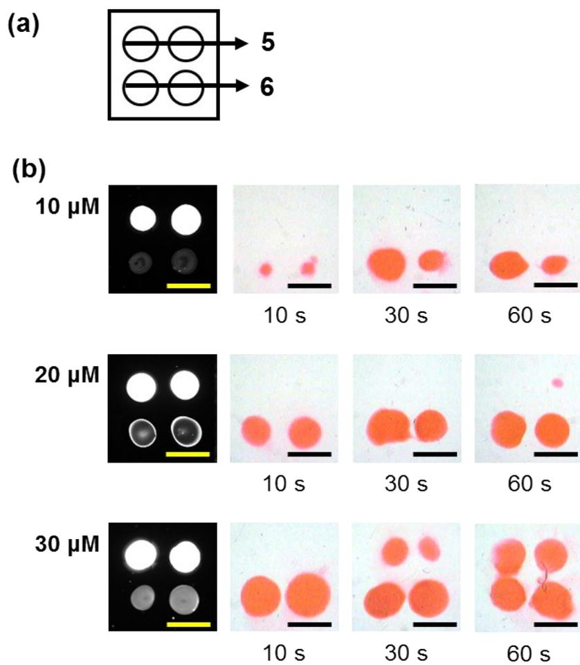
**Fig. S9** (a) Schematic diagram of a chip for (5) and (6). (b) Fluorescence image (left) and colorimetric readout (2<sup>nd</sup> ~4<sup>th</sup> columns) of (5) and (6) under varied concentrations and irradiation times. Scale bars represent 0.2 cm.
