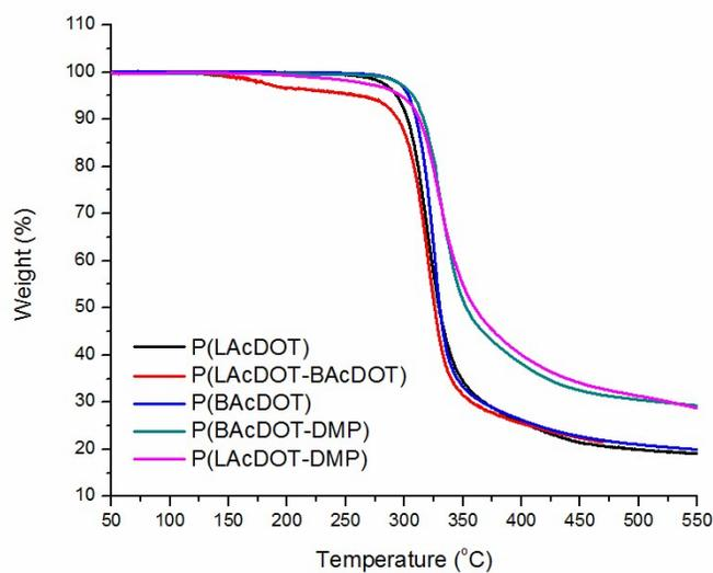
**Figure S9.** TGA studies performed at a rate of 10 °C/minutes.
