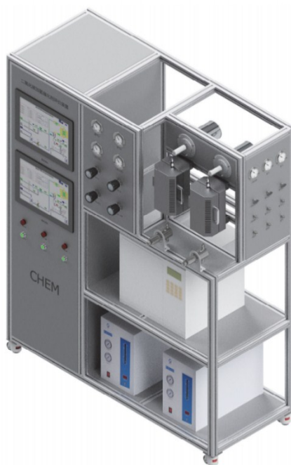
Fig. S16. 3D illustration of the device about CO 2 catalytic evaluation and online detection.
