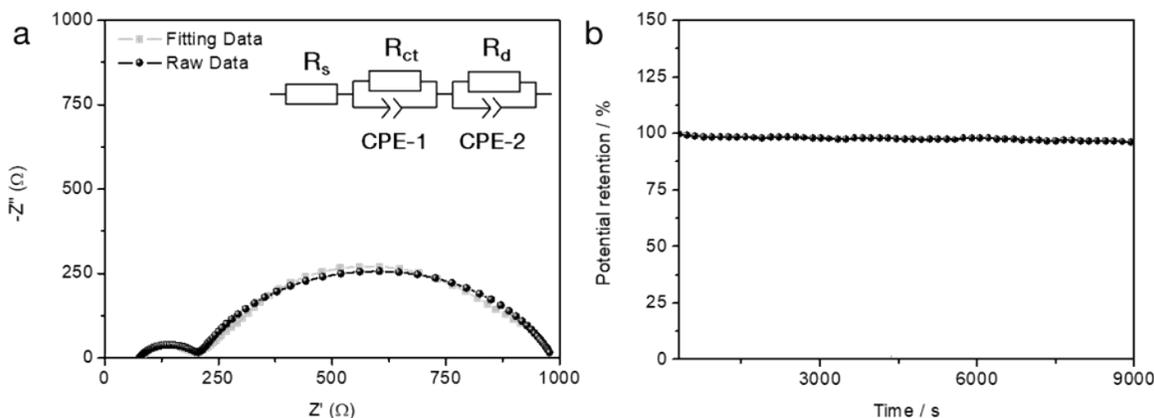
Figure S5. (a) Nyquist plot and (b) chronopotentiometric curve of CoP NCs. Two semicircles are assigned to the charge transfer resistance ( $R_{ct}$ ) and mass-transport resistance ( $R_d$ ) in turn.  $R_s$ ,  $R_{ct}$  and  $R_d$  were estimated to be 84.0, 132.1 and 778.1  $\Omega$ , respectively.
