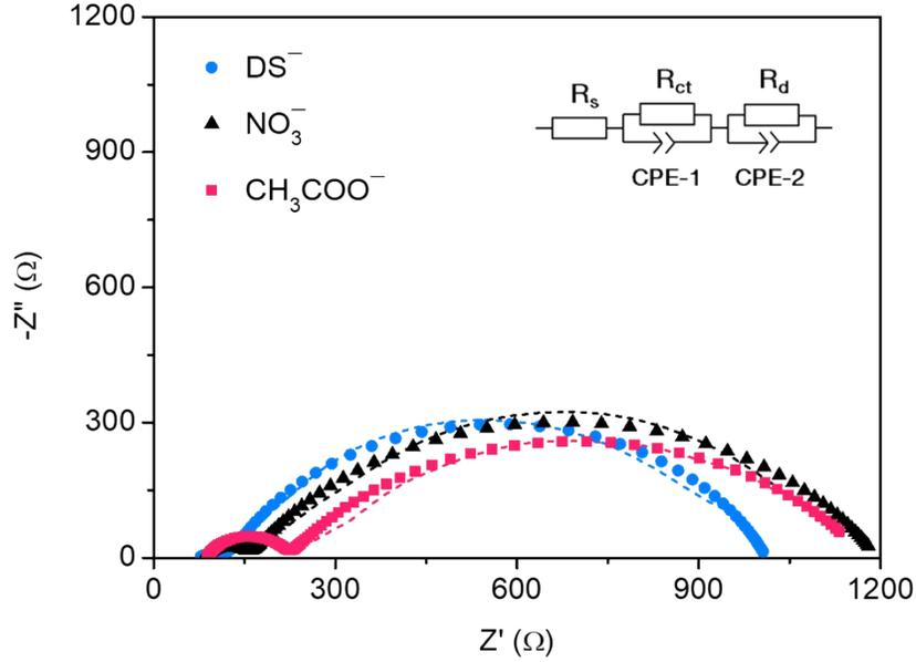
Figure S3. (a) Nyquist plots of  $\text{DS}^-$ ,  $\text{NO}_3^-$ ,  $\text{CH}_3\text{COO}^-$ -intercalated cobalt hydroxide NCs. Two semicircles are assigned to the charge-transfer resistance ( $R_{ct}$ ) and mass-transfer resistance ( $R_d$ ) in turn. The shot dashes represent the raw data and the symbol dots represent the fitting data. The inset is the equivalent circuit model.
