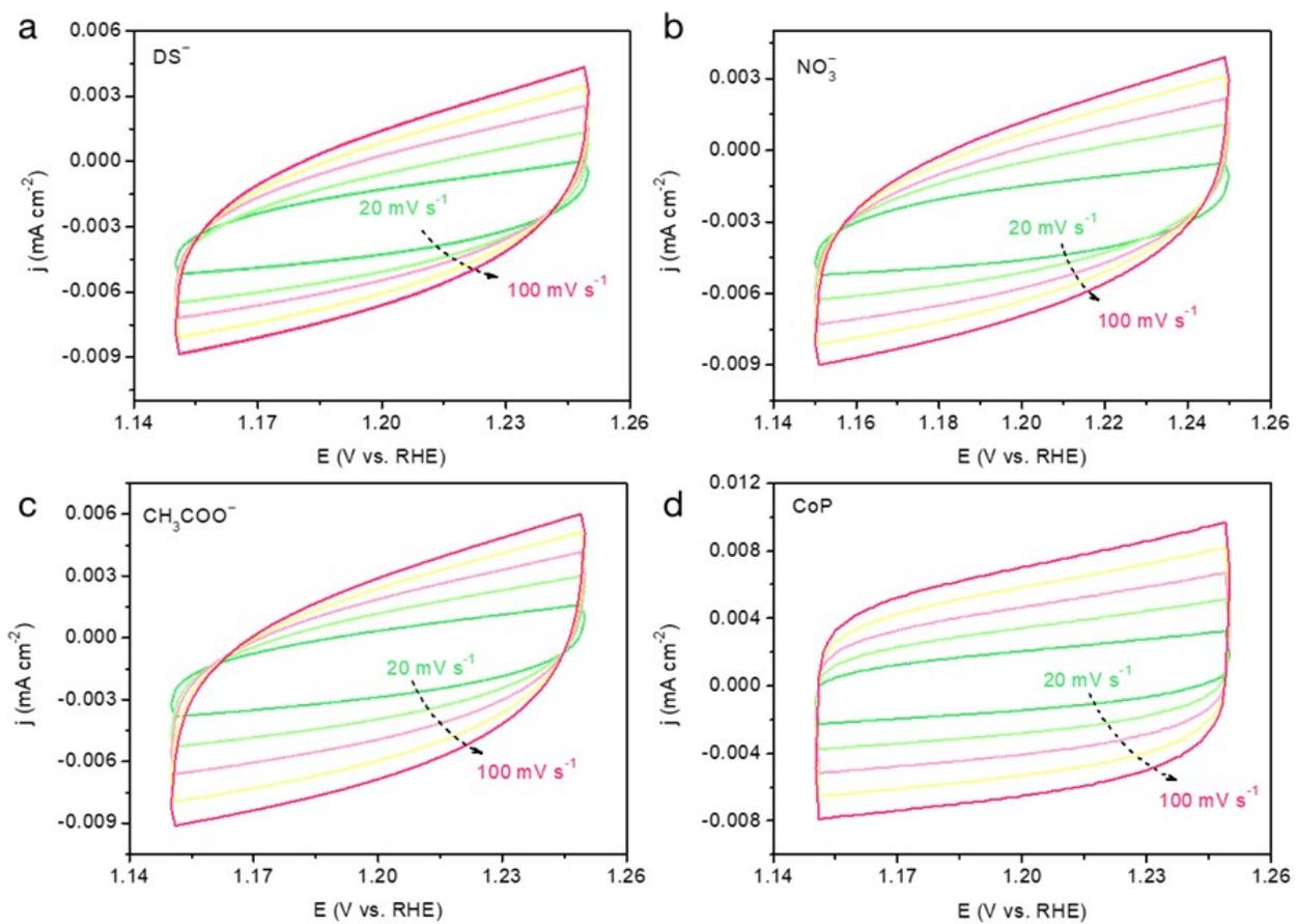
Figure S2. Cyclic voltammetry (CV) curves for (a)  $DS^-$ , (b)  $NO_3^-$ , (c)  $CH_3COO^-$ -intercalated cobalt hydroxide NCs and (d) CoP NCs at incremental scan rates in the potential range of 1.15 - 1.25 V vs RHE.
