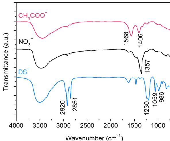
Figure S1. FT-IR spectra of layered cobalt hydroxide NCs intercalated with DS<sup>-</sup>, NO<sub>3</sub><sup>-</sup> and CH<sub>3</sub>COO<sup>-</sup> anions, respectively.
