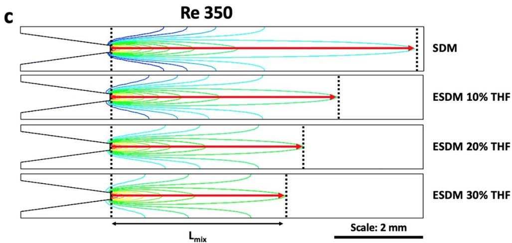
**Figure S3.** Contour lines of mass fraction of THF to study the effect of variation of %THF (x) in ant-solvent on  $L_{mix}$  at (a) Re 46.7, (b) Re 116.7 and (c) Re 350.
