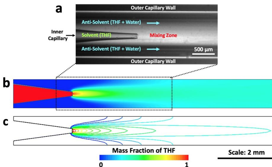
**Figure S2.** (a) Microscopy image of microfluidic glass capillaries with tip of inner capillary (solvent flow) inside outer capillary (anti-solvent flow). Contour of mass fraction of THF with (b) smooth shading and (c) contour lines after mixing between solvent (THF) and anti-solvent (water) in the process of SDM at Re 350.
