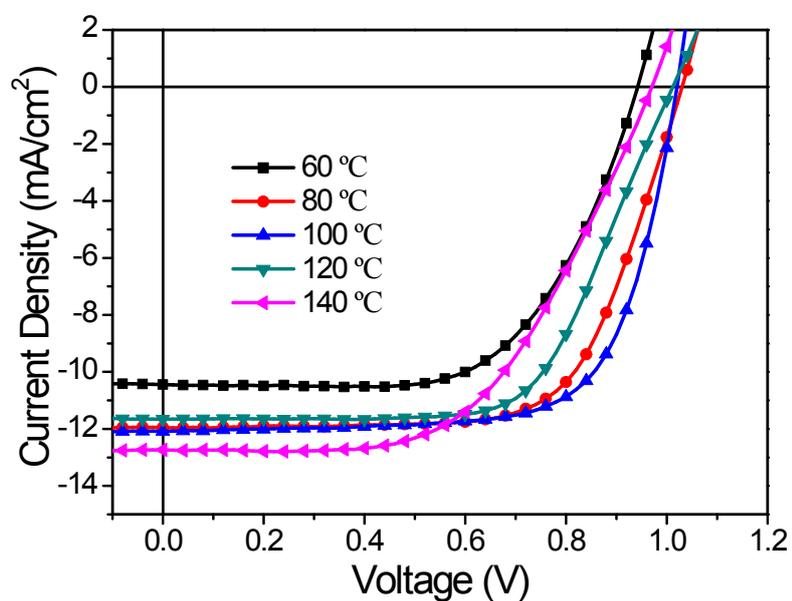
**Figure S4**  $J$ - $V$  curves for PSCs with different annealing temperature (35  $\mu$ L/mL HBr, annealing time 10 min).
