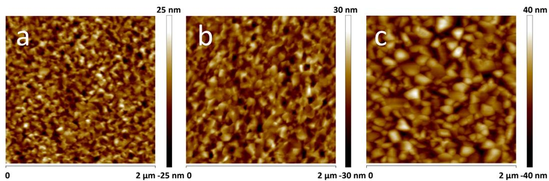
**Figure S13** AFM height images for CsPbI<sub>3</sub> films with HBr additive annealed at 100 °C for 20 s (a), 15 min (b) and 60 min (c).
