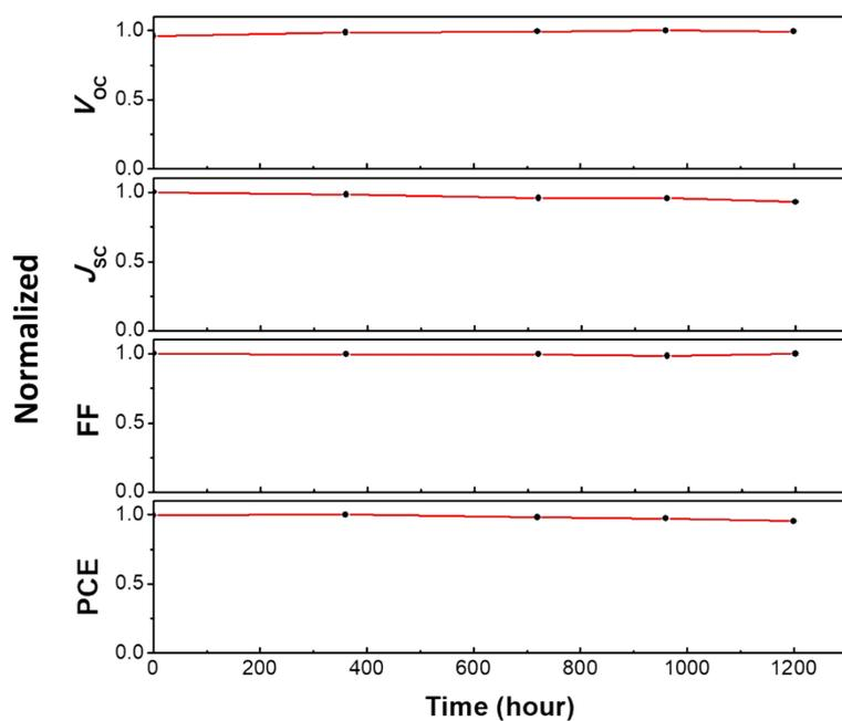
**Figure S12** Tracking the device performance in a N<sub>2</sub> glovebox for 1200 hours.
