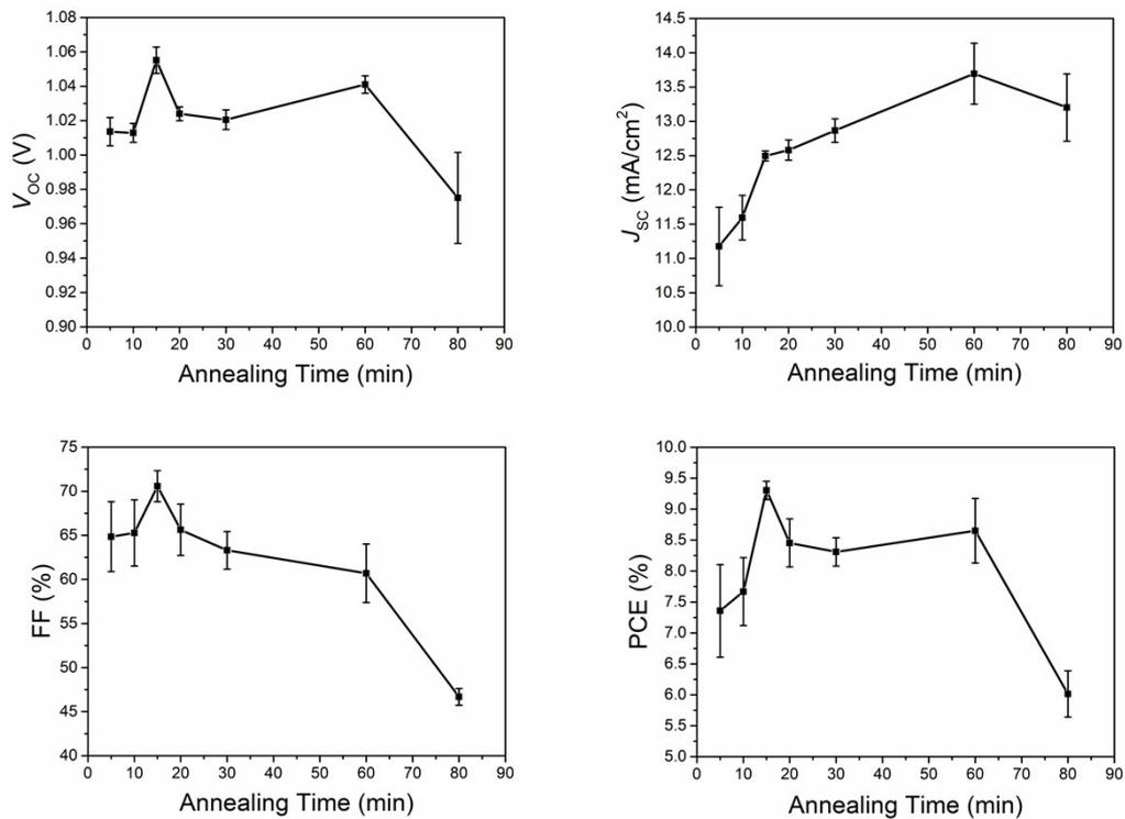
**Figure S5** The performance parameters ( $V_{OC}$ ,  $J_{SC}$ , FF, PCE) of CsPbI<sub>2.69</sub>Br<sub>0.31</sub> solar cells plotted against the annealing time.
