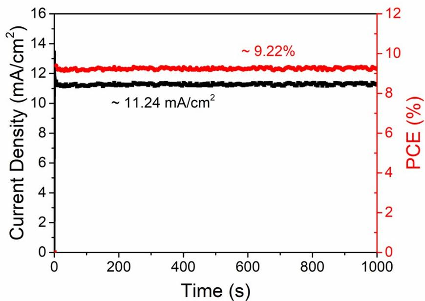
**Figure S11** Photocurrent measured under 0.82 V bias near the maximum power point and PCE (active area 4 mm<sup>2</sup>).
