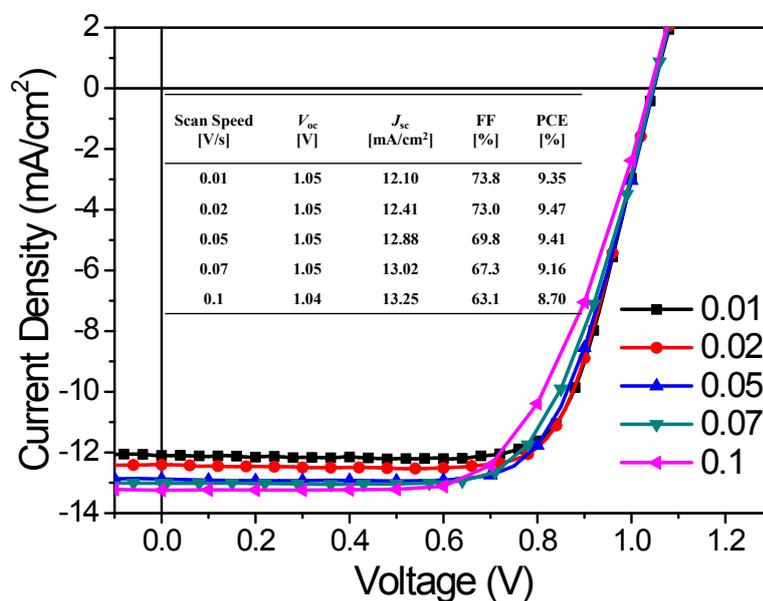
**Figure S10**  $J$ - $V$  curves and performance data (inset) under different scan speeds (0.01 V/s; 0.02 V/s; 0.05 V/s; 0.07 V/s; 0.1 V/s) for the  $\text{CsPbI}_{2.69}\text{Br}_{0.31}$  solar cell.
