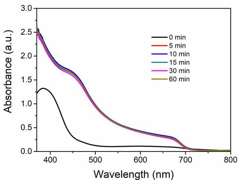
**Figure S7** The absorption spectra for CsPbI<sub>2.69</sub>Br<sub>0.31</sub> films with different annealing time.
