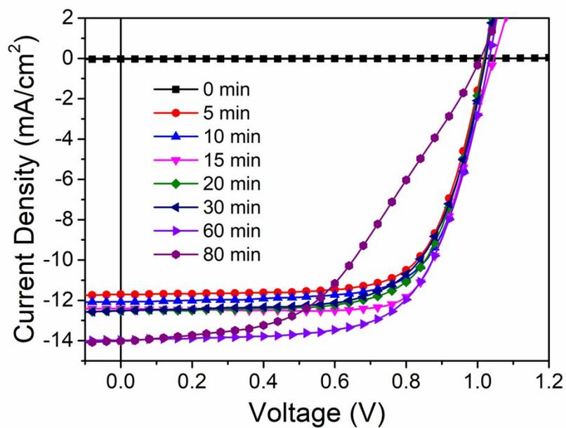
**Figure S6** The  $J-V$  curves for devices with different annealing time (35  $\mu$ L/mL HBr, annealing temperature 100  $^{\circ}$ C).
