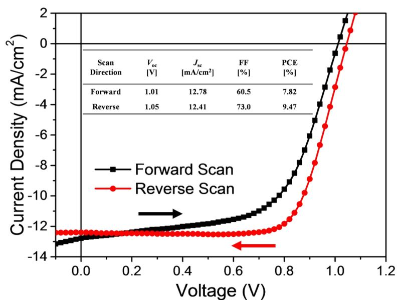
**Figure S9**  $J$ - $V$  curves (forward and reverse) and performance data (inset) for the  $\text{CsPbI}_{2.69}\text{Br}_{0.31}$  solar cell.
