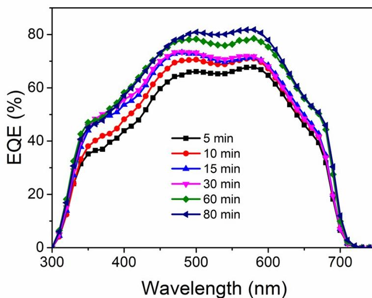
**Figure S8** EQE spectra for CsPbI<sub>2.69</sub>Br<sub>0.31</sub> solar cells with different annealing time.
