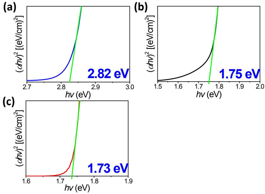
**Figure S1** Tauc plots for perovskite films made without additive (a), with HBR additive (b) and with HI additive (c).
