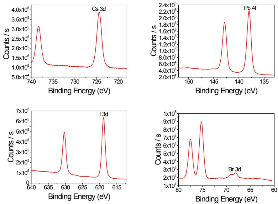
**Figure S2** XPS spectra of  $\text{CsPbI}_{2.69}\text{Br}_{0.31}$  film.
