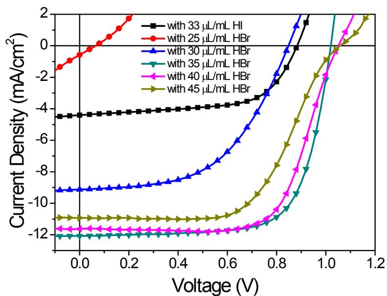
**Figure S3**  $J$ - $V$  curves for PSCs made with different additive concentrations (annealing temperature 100 °C, annealing time 10 min).
