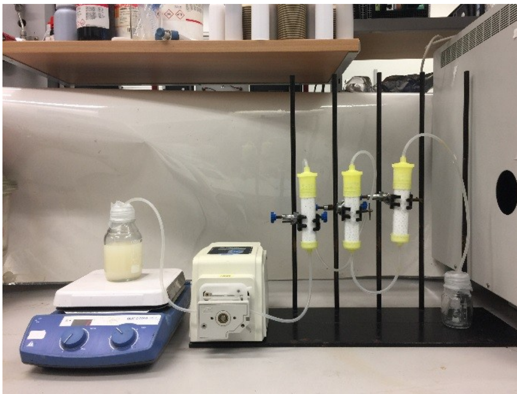
Fig. S6 Photo illustrating continuous process for biodiesel production in an integrated continuous stirred tank reactor with three packed bed reactors (CSTR-PBRs) connected in series.
