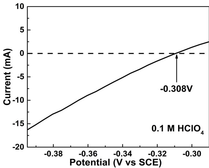
**Figure S1.** LSV curves collected at room temperature in H<sub>2</sub>-saturated 0.1 M HClO<sub>4</sub> aqueous solution with a scan rate of 1 mV·s<sup>-1</sup>. The experiment was performed in a H<sub>2</sub>-saturated electrolyte with platinum wire as working electrode. The thermodynamic equilibrium potential for H<sup>+</sup>/H<sub>2</sub> reaction was determined at zero current.
