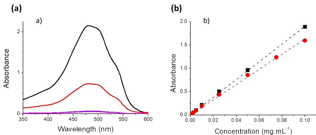
**Figure S1.** a) Absorption spectra for the initial solution (0.12 mg.mL<sup>-1</sup>) of DOX loading (black curve) as well as the filtrate and washing solutions after the nanoparticles removing (red for the first filtrate, blue for the second and pink for the third); b) Calibration curves for the doxorubicin in water (black curve) and in PBS (red curve).
