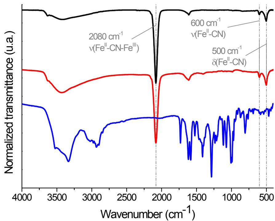
**Figure S2.** FTIR spectra for **1** (black) and **1@DOX** (red) and doxorubicin (blue).
