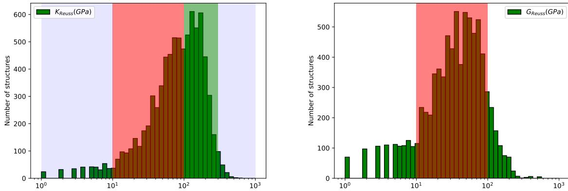
Figure 8: Histogram of log Reuss bulk modulus and log reuss shear modulus for 8,050 synthesized inorganic compounds. The corresponding values are extracted from the Material Project database. The different areas colors is related to the distribution of materials relative to their respective values.
