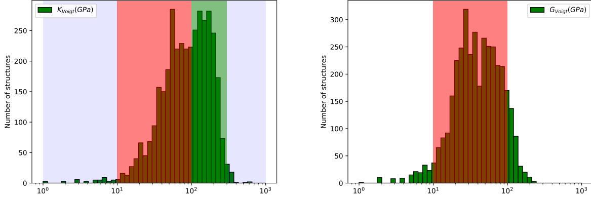
Figure 9: Histogram of log Voigt bulk modulus and log Voigt shear modulus for 3,714 hypothetical inorganic compounds. The corresponding values are extracted from the Material Project database. The different areas colors is related to the distribution of materials relative to their respective values.
