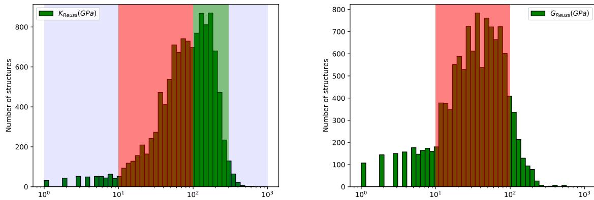
Figure 6: Histogram of log Reuss bulk modulus and log Reuss shear modulus for 11,764 inorganic compounds. The corresponding values are extracted from the Material Project database. The different areas colors is related to the distribution of materials relative to their respective values.
