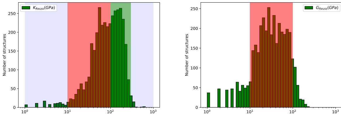
Figure 10: Histogram of log Reuss bulk modulus and log Reuss shear modulus for 3,714 hypothetical inorganic compounds. The corresponding values are extracted from the Material Project database. The different areas colors is related to the distribution of materials relative to their respective values.
