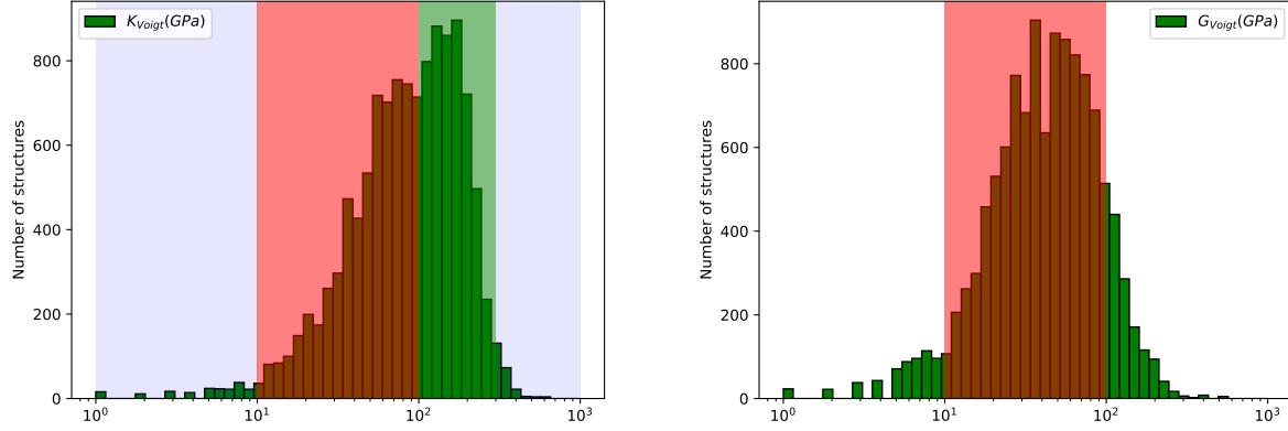
Figure 5: Histogram of log Voigt bulk modulus and log Voigt shear modulus for 11,764 inorganic compounds. The corresponding values are extracted from the Material Project database. The different areas colors is related to the distribution of materials relative to their respective values.
