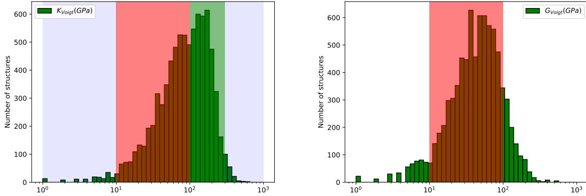
Figure 7: Histogram of log Voigt bulk modulus and log Voigt shear modulus for 8,050 synthesized inorganic compounds. The corresponding values are extracted from the Material Project database. The different areas colors is related to the distribution of materials relative to their respective values.
