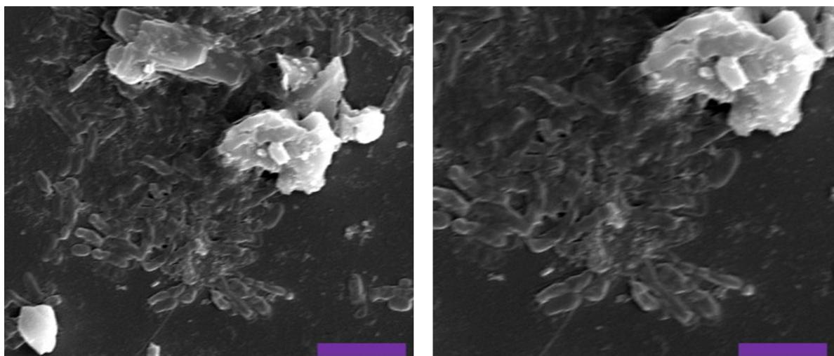
**Figure S17-** SEM images of non-templated CLEA formed from free PLE in solution. Please note the broad size distribution as a result of uncontrolled cross-linking. Scale bars correspond to 5  $\mu\text{m}$ .
