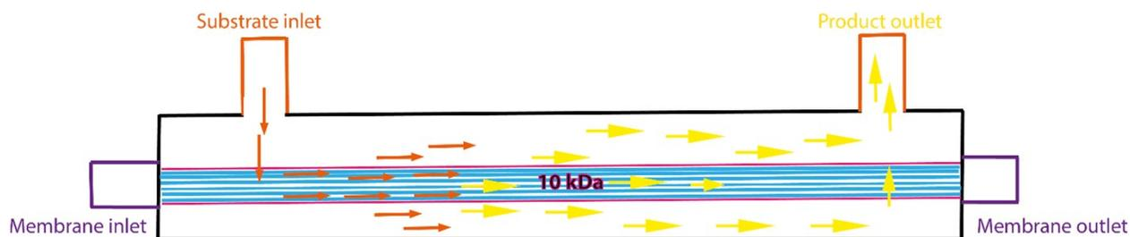
**Figure S13-** Schematic representation of the flow reactor system. The orange arrows indicate the diffusion of the substrate throughout the permeable membrane, and its conversion into the product *p*- nitrophenol (yellow arrows) that can be collected at the product outlet.
