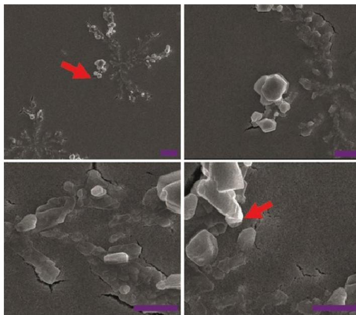
**Figure S6-** SEM images of non-templated CLEA formed from free CalB in solution. Please note the broad size distribution (red arrows indicate macro-cluster formation in the range of 5 to 20  $\mu$ m) as a result of uncontrolled cross-linking. Scale bars correspond to 10  $\mu$ m.
