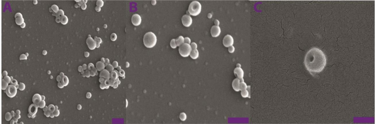
**Figure S2-** SEM images of A) open neck stomatocytes B) Stomatocytes after neck closure C), and subsequent cross-linking reaction using 100 mM of glutaraldehyde. Scale bars correspond to 500 nm
