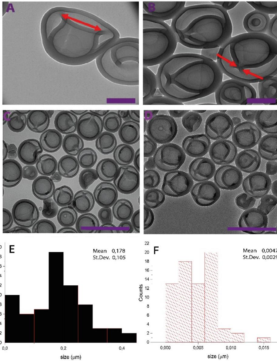
**Figure S1-** TEM images of A) Open neck stomatocytes B) CalB loaded stomatocytes after neck closure. C) PLE- loaded stomatocytes after neck closure. D) GOx/HRP- loaded stomatocytes after neck closure. Scale bar corresponds to 100nm in A) B) and 1 μm in C) D). Histogram analysis of stomatocytes' neck size: E) open neck F) closed-neck
