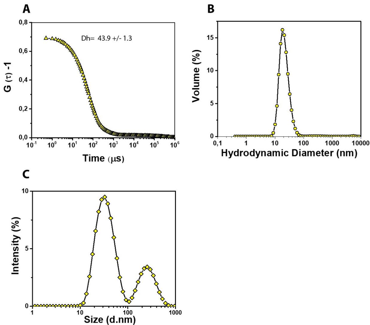
**Figure S4-** A) correlation function of the released CalB CLEnA; B) volume profile derived from A, showing a size distribution of ~43 nm and a PDI of 0.5, C) DLS Intensity distribution of the released CalB CLEnA. Please note the two peaks; one is corresponding to the released CLEnA (~43 nm) and the other is corresponding to the stomatocytes left in solution (~300nm).
