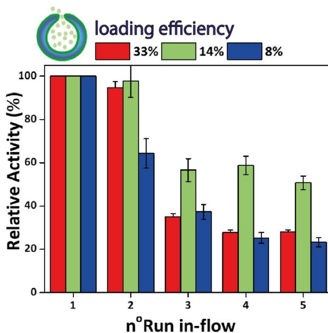
**Figure S14-** Relative activity of stomatocyte nanoreactors with different CalB loading during five runs in-flow (each run 13 min, 0.3 mL min<sup>-1</sup>).
