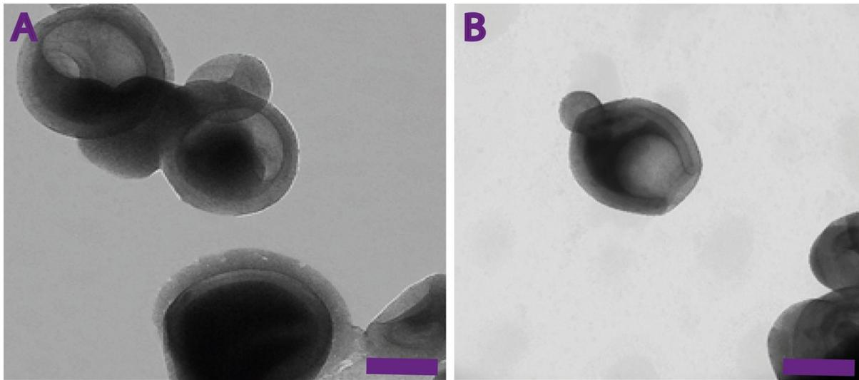
**Figure S10-** TEM images of A) PLE *c-CLEnA* formed with genipin B) GOX/HRP *c-CLEnA* formed with genipin. Scale bar corresponds to 100nm
