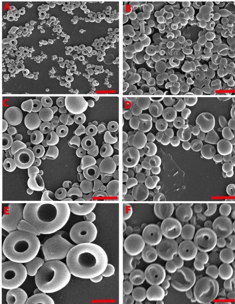
**Figure S18-** SEM images of A) B) C) open neck stomatocytes (used for PLE encapsulation); D) E) F) PLE *c-CLEnA* prepared with 50mM of genipin. Scale bar corresponds to 3  $\mu\text{m}$  in A and B, 1  $\mu\text{m}$  in C and D and 400nm in E and F.
