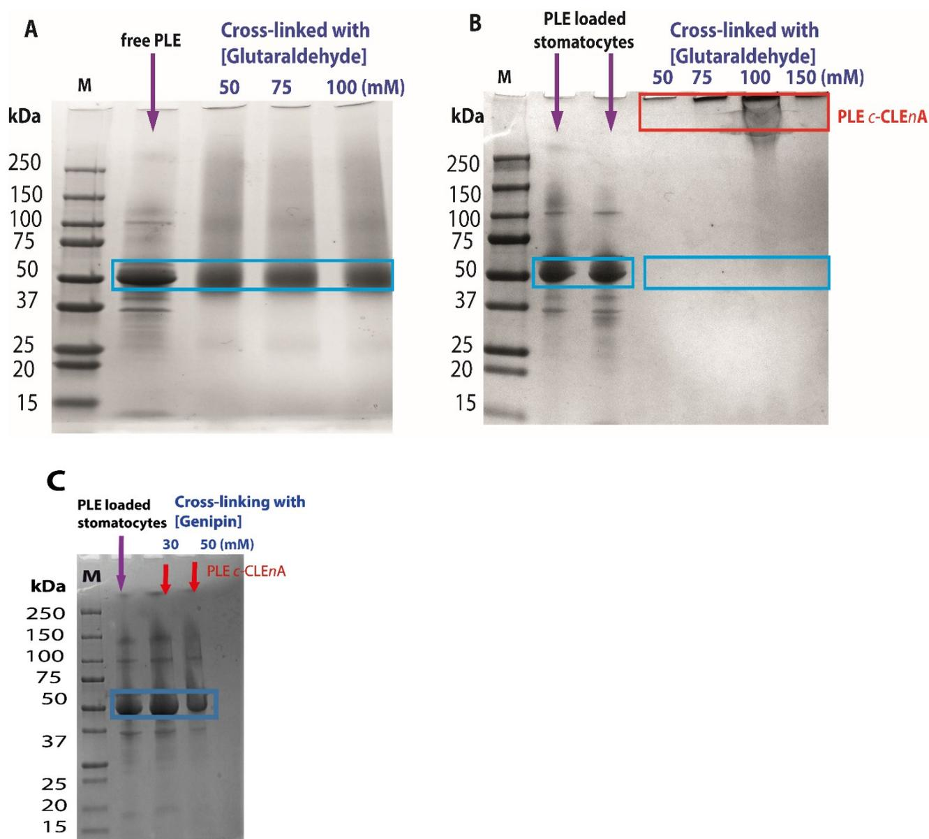
**Figure S9-** A) SDS-PAGE gel of PLE cross-linked with different glutaraldehyde concentrations in solution. From left to right: molecular weight ladder (M), the second lane (indicated with an arrow)
