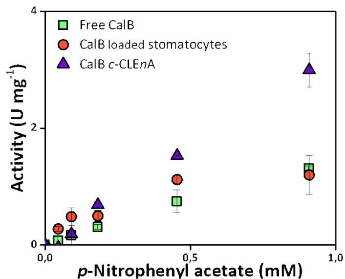
**Figure S7-** Comparison between specific activity (U mg<sup>-1</sup>) of free CalB, CalB loaded stomatocytes (with non-cross-linked CalB), and CalB c-CLEnA. The absorbance of the product is measured at 405 nm at different concentration of substrate.
