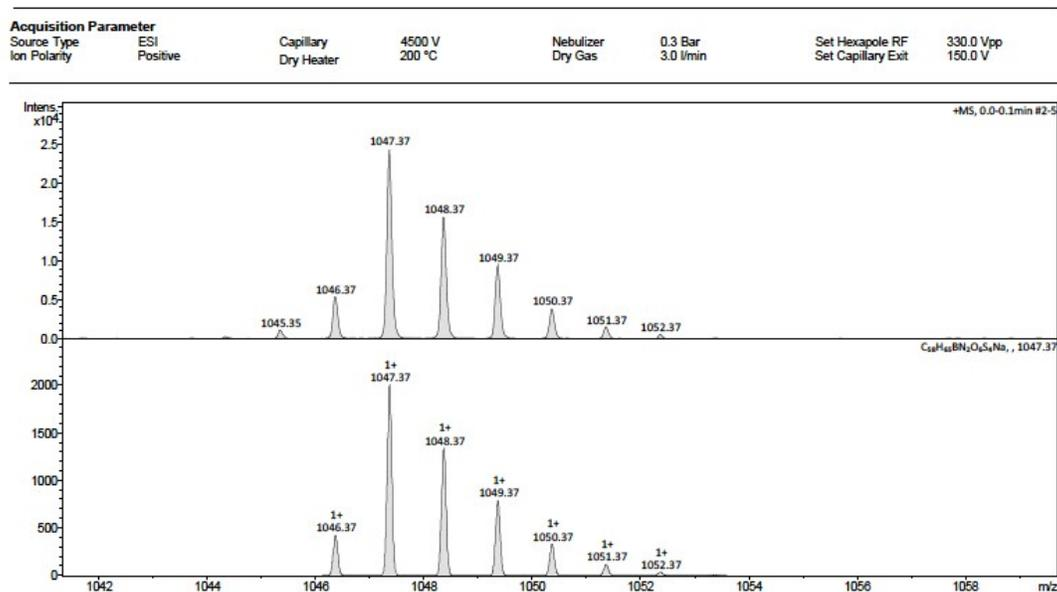
Figure S1. zoom (top) + simulation (bottom) analysis of T''<sub>2</sub>P<sub>2</sub>A
