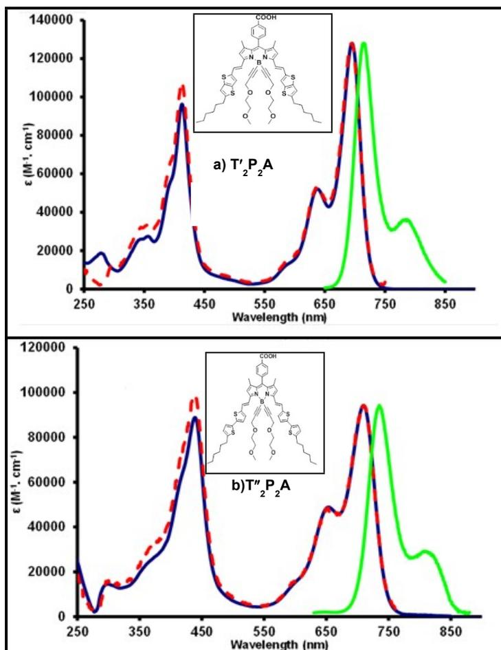
Figure S3. Absorption spectra (orange), emission spectra (green) and the excitation spectra (dashed l) in THF of a) T'<sub>2</sub>P<sub>2</sub>A and b) T''<sub>2</sub>P<sub>2</sub>A photosensitizers
