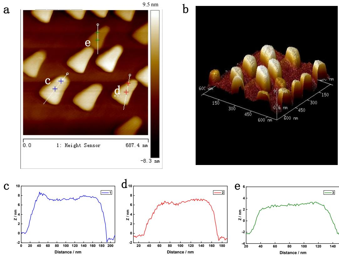
**Figure S4.** Typical AFM and 3D AFM images of the electrolyzed sample under 2.8 V at 950 °C for 8 h (a,b). The thinness at different locations (c-e).
