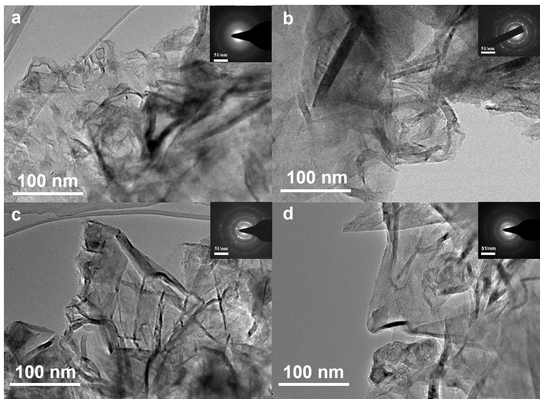
**Figure S3.** TEM images of Cellulose material after cathodic electrolysis cathodic under different constant cell voltages : (a) 2.0V, (b) 2.2 V, (c)2.4V,(d)2.6V at 950 °C for 8 h.
