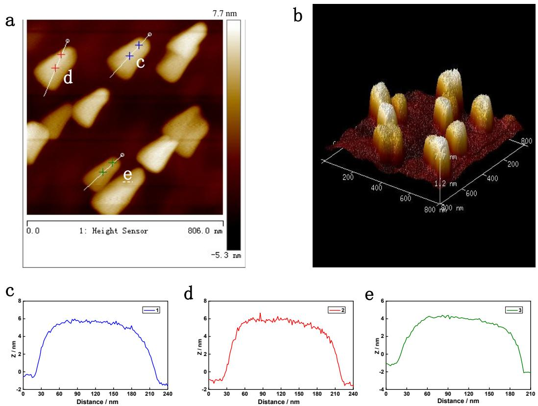
**Figure S5.** Typical AFM and 3D AFM images of the electrolyzed sample under 2.8 V at 900 °C for 8h (a,b). The thinness at different locations (c-e).
