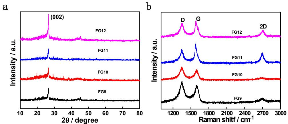
**Figure S1.** (a) XRD patterns of cellulose resources after cathodic electrolysis under 2.0 V, 2.2 V, 2.4 V and 2.6 V, which obtained FG9, FG10, FG11 and FG12 at 950 °C for 8 h. (b) Raman spectra of cellulose resources after cathodic electrolysis under 2.0 V, 2.2 V, 2.4 V and 2.6 V, which obtained FG9, FG10, FG11 and FG12 at 950 °C for 8 h.
