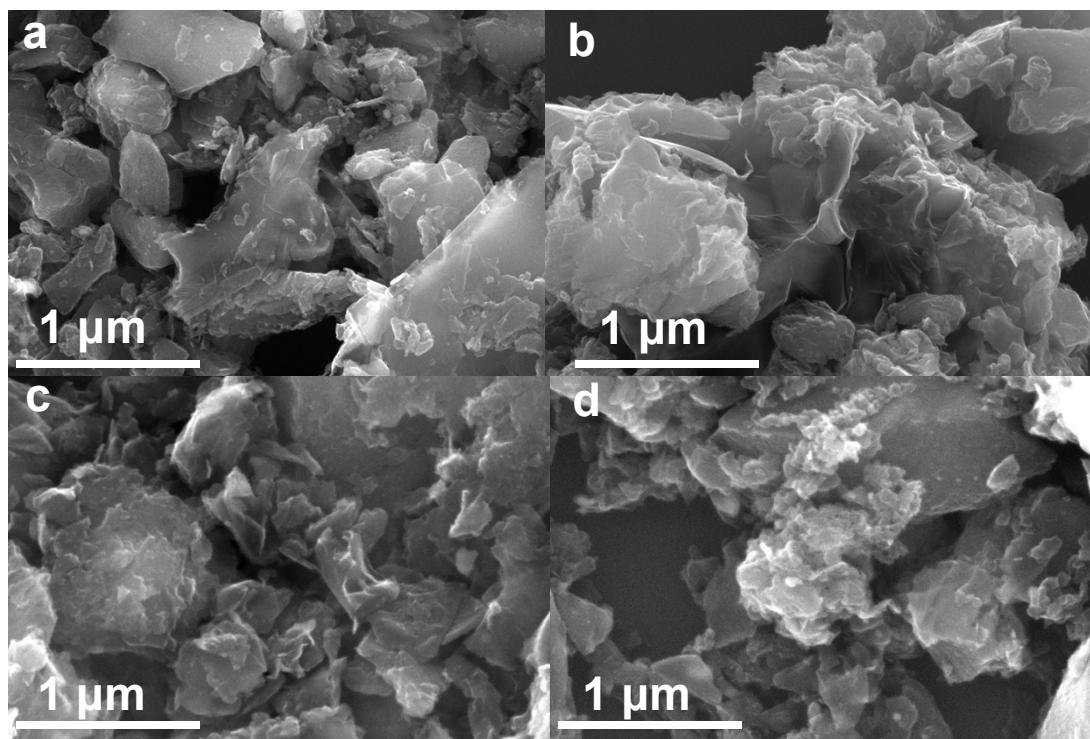
**Figure S2.** SEM images of Cellulose material after cathodic electrolysis cathodic under different constant cell voltages : (a) 2.0 V, (b) 2.2 V, (c) 2.4 V, (d) 2.6 V at 950 °C for 8 h.
