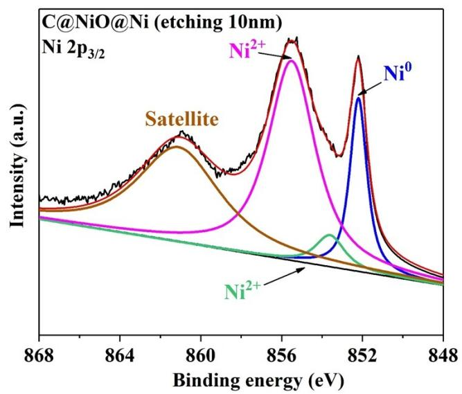
**Fig. S2.** The Ni 2p<sub>3/2</sub> XPS pattern using Ar particles to etch C@NiO@Ni for 10 nm.
