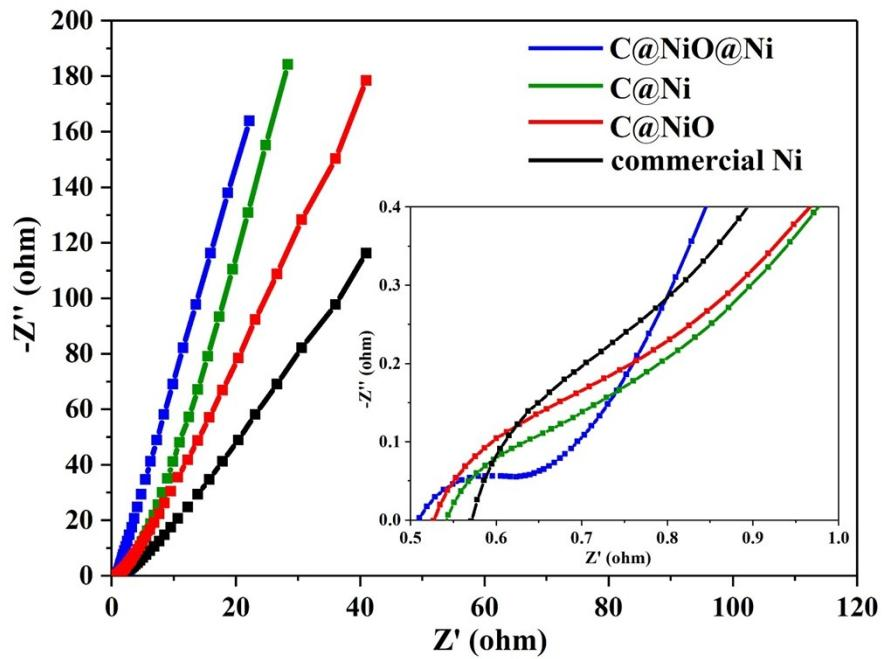
**Fig. S21.** EIS plots of C@Ni, C@NiO@Ni, C@Ni and commercial Ni in 0.1 M KOH.
