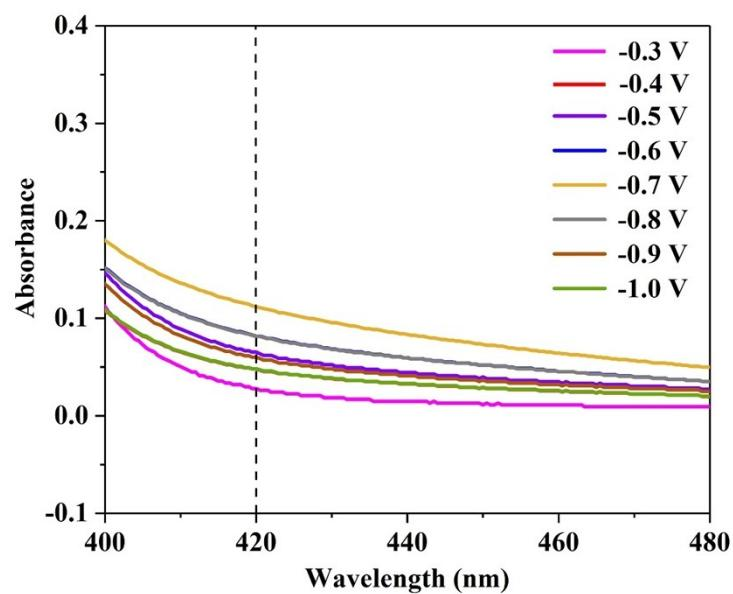
**Fig. S10.** UV-Vis absorption curves of the electrolyte after tests of C@NiO@Ni at different potentials.
