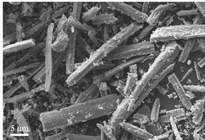
**Fig. S5.** SEM image of Ni-MOF (Ni-BTC) precursor.
