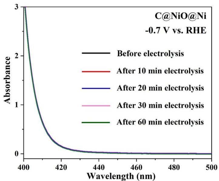
**Fig. S17.** UV-Vis absorption spectra of the electrolytes stained with p-C<sub>9</sub>H<sub>11</sub>NO indicator after NRR electrolysis at different time.
