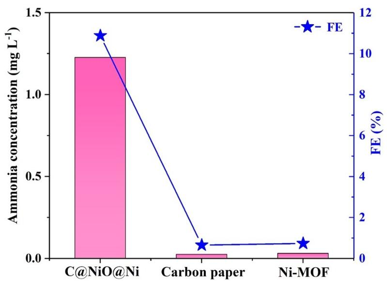
**Fig. S18.** Ammonia concentration and FE of C@NiO@Ni/CP, Ni-MOF/CP and CP after 1 h electrolysis at a potential of  $-0.7$  V under ambient conditions.
