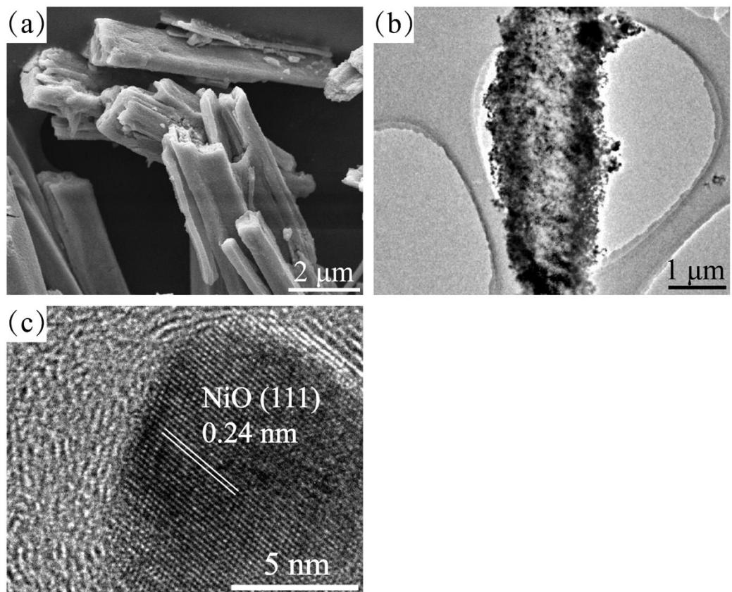
**Fig. S7.** (a) SEM image, (b) TEM image and (c) HRTEM image of C@NiO microtubes.
