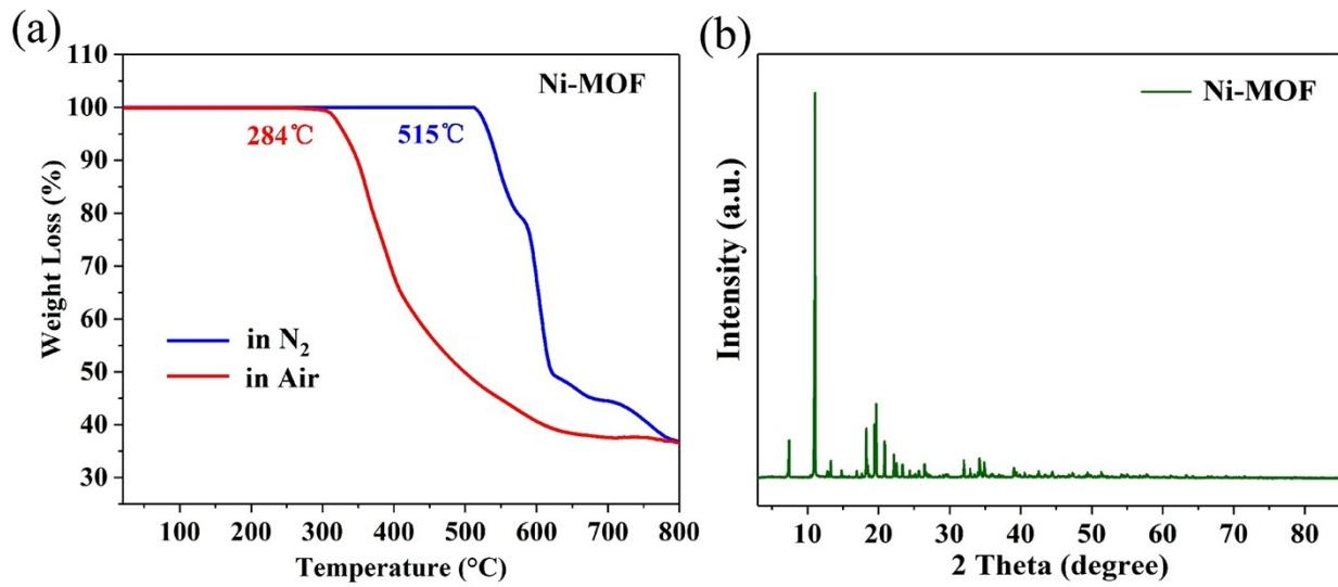
**Fig. S1.** (a) Thermogravimetric curve of Ni-MOF (Ni-BTC) in Air and N<sub>2</sub>. (b) XRD pattern of Ni-MOF (Ni-BTC).
