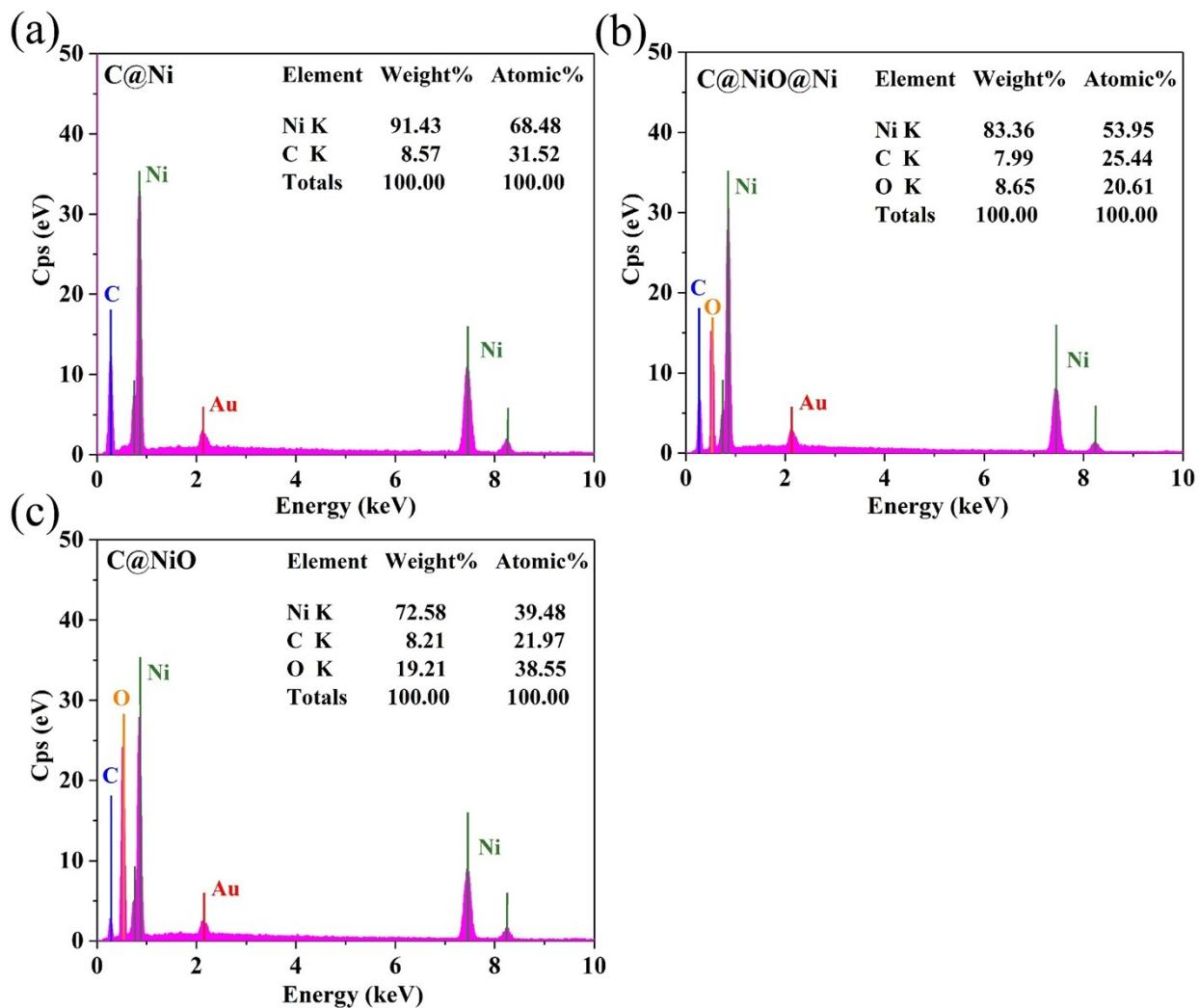
**Fig. S8.** (a) EDX of C@Ni. (b) EDX of C@NiO@Ni. (c) EDX of C@NiO.
