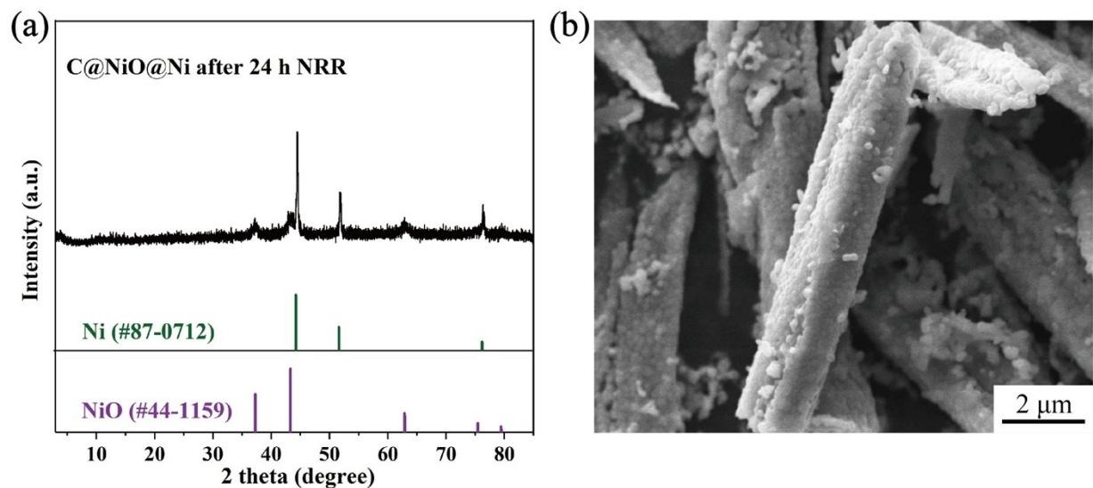
**Fig. S19.** (a) XRD pattern, (b) SEM image of C@NiO@Ni after 24 h NRR.
