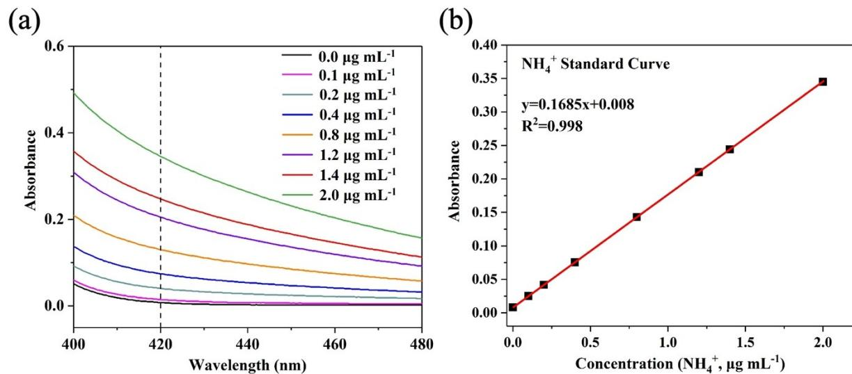
**Fig. S9.** (a) UV-Vis absorption curves of Nessler's reagent assays kept with different concentrations of  $\text{NH}_4^+$  ions. (b) A calibration curve used to estimate the concentrations of  $\text{NH}_4^+$  ions.
