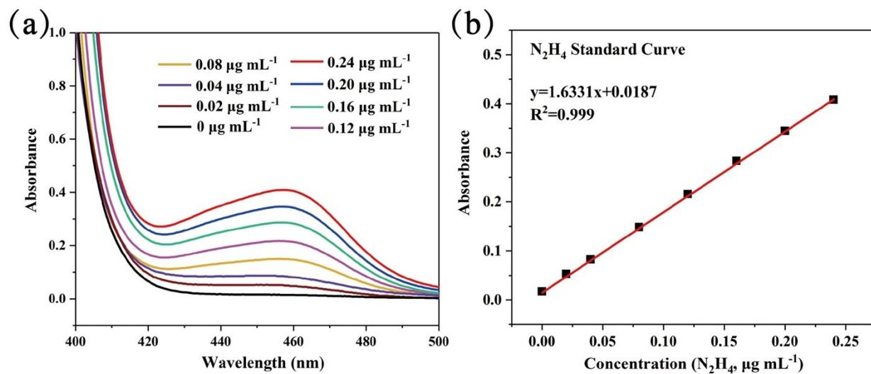
**Fig. S16.** (a) UV-Vis curves of various concentrations of  $\text{N}_2\text{H}_4$  stained with  $\text{p-C}_9\text{H}_{11}\text{NO}$  indicator.
