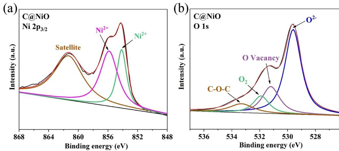
**Fig. S4.** XPS Ni 2p<sub>3/2</sub> (a) and O 1s (b) spectra for the C@NiO.
