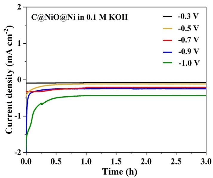
**Fig. S11.** Chronoamperometry results of C@NiO@Ni at the corresponding potentials.
