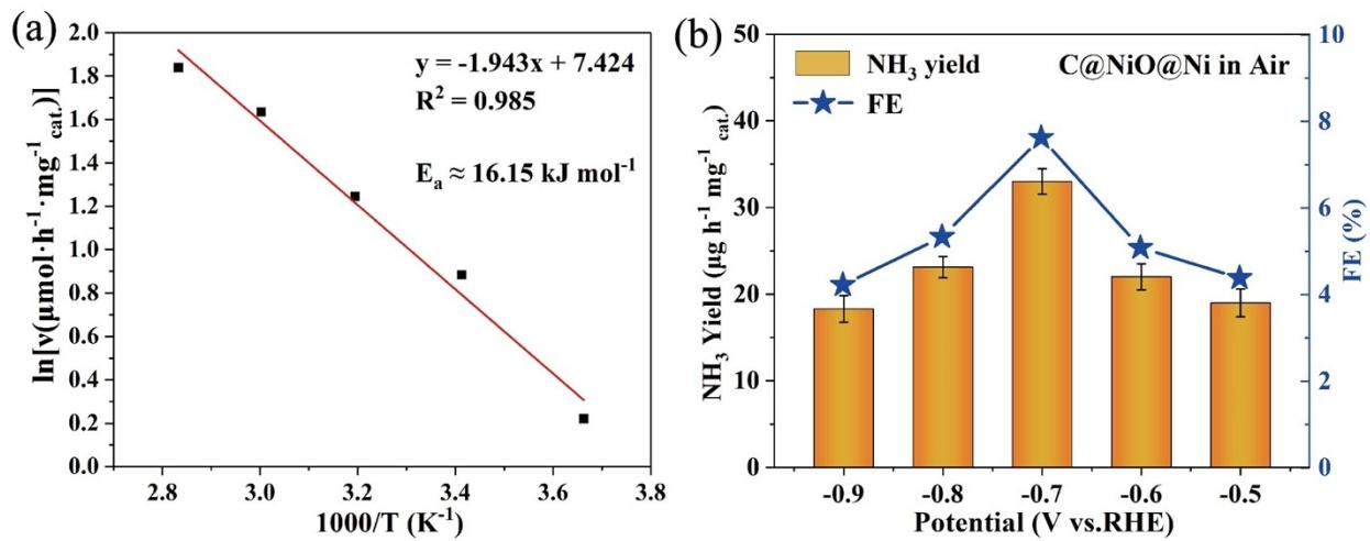
**Fig. S20.** (a) Arrhenius plot of the NRR rate over C@NiO@Ni catalyst at the temperature from 273 to 353 K. (b)  $\text{NH}_3$  yields and FE for C@NiO@Ni at different potentials in Air.
