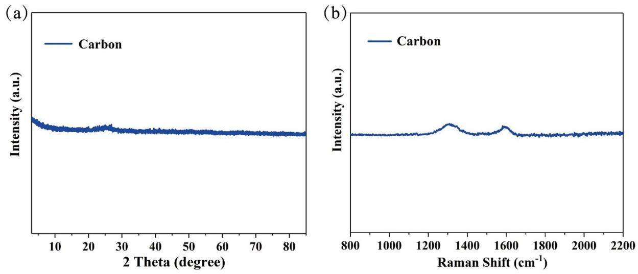
**Fig. S12.** (a) XRD pattern of carbon (etching NiO and Ni of C@NiO@Ni by HNO<sub>3</sub>). (b) Raman pattern of carbon (etching NiO and Ni of C@NiO@Ni by HNO<sub>3</sub>).
