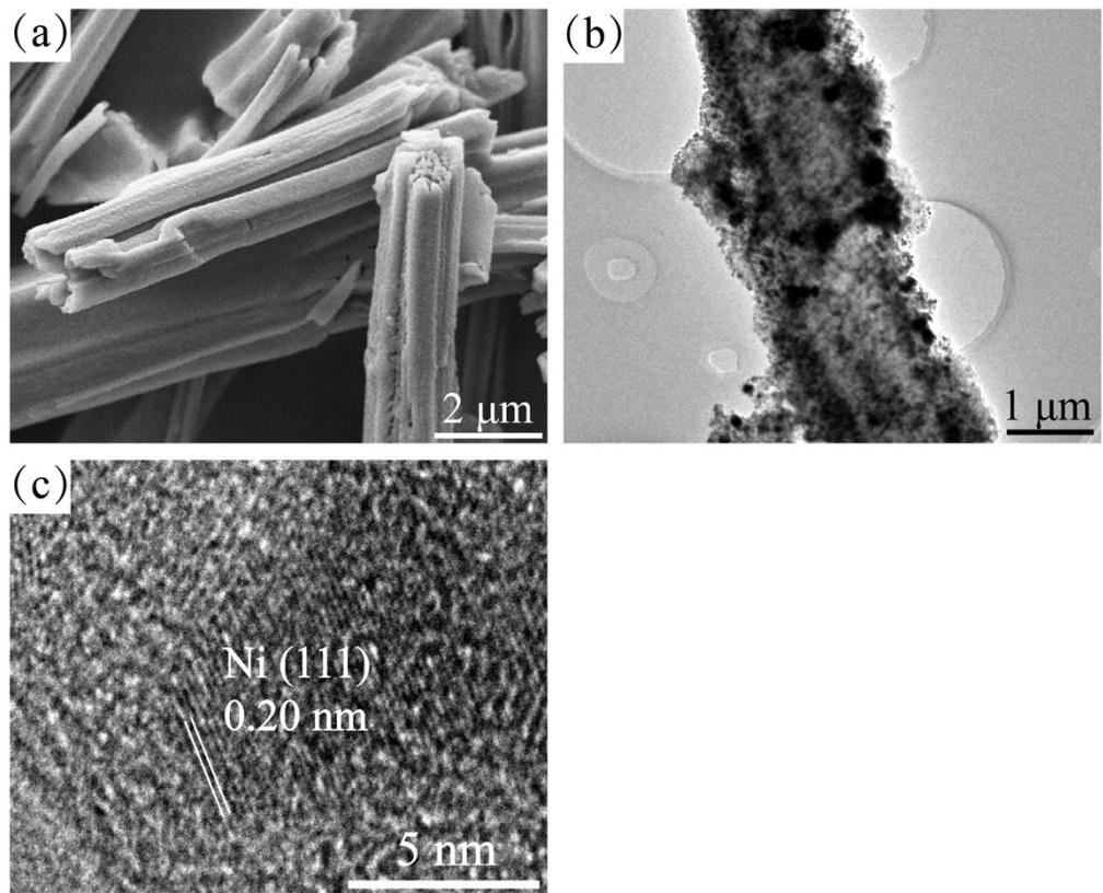
**Fig. S6.** (a) SEM image, (b) TEM image and (c) HRTEM image of C@Ni microtubes.
