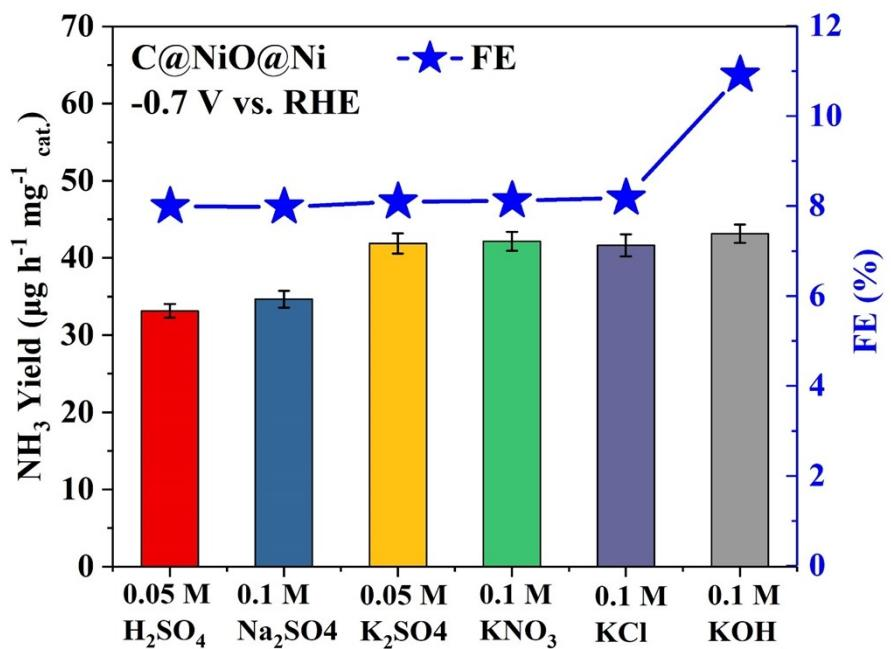
**Fig. S13.** NRR performance of C@NiO@Ni in different electrolytes at -0.7 V.
