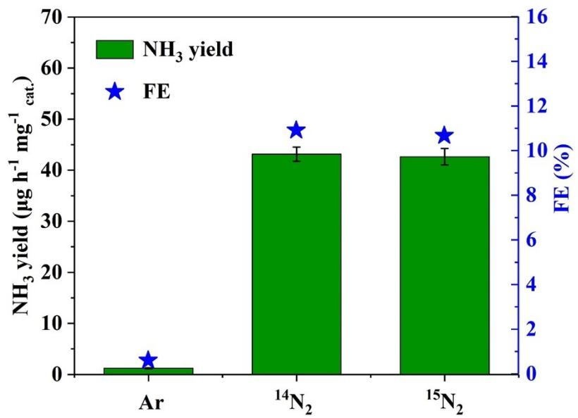
**Fig. S15.** Comparison of the Faradaic efficiency and  $\text{NH}_3$  yield of C@NiO@Ni using different feeding gases for the NRR at -0.7 V.
