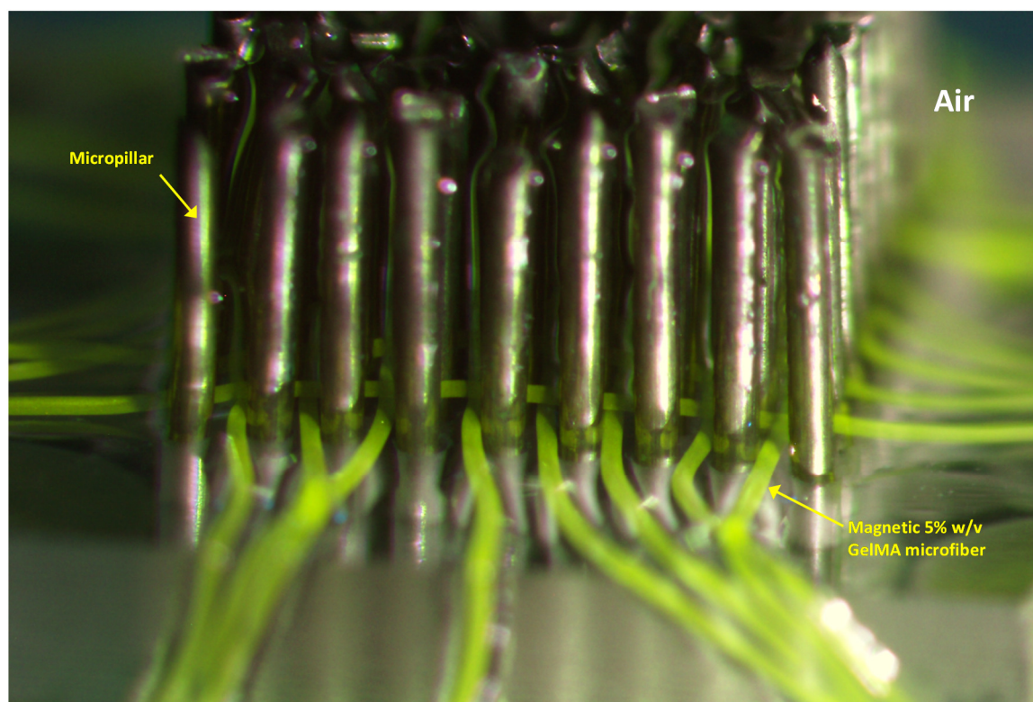
Figure S1. Surface tension enables the upper and lower microfibers to directly contact where they crossed.
