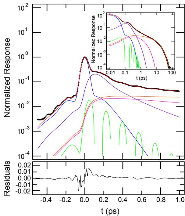
Figure S2: (Top panel) Example of raw data (open black circles) with the full fit (red line) and the constituent electronic (blue line), librational (purple line), intermediate (magenta line), vibrational (green line), and diffusive responses for PC at 310 K. The inset is the same plot on a full scale logarithmic plot. (Bottom panel) Residuals of the fit.
