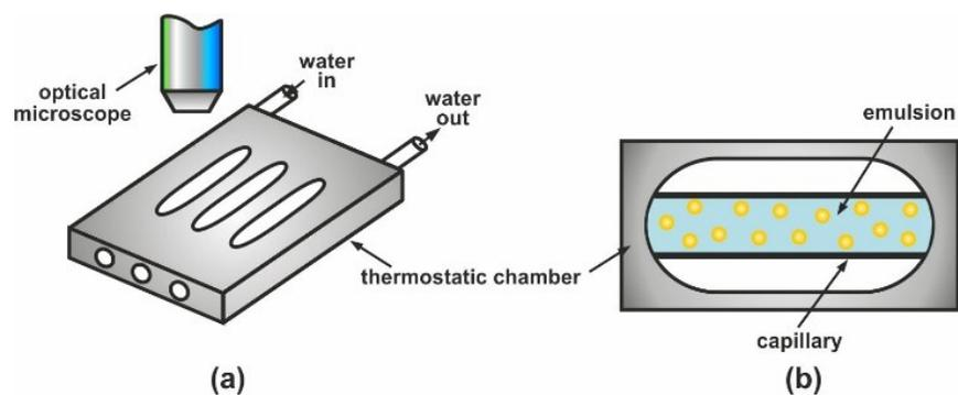
**Figure S1.** Experimental setup for optical observations of emulsion drops in a glass capillary upon cooling.
