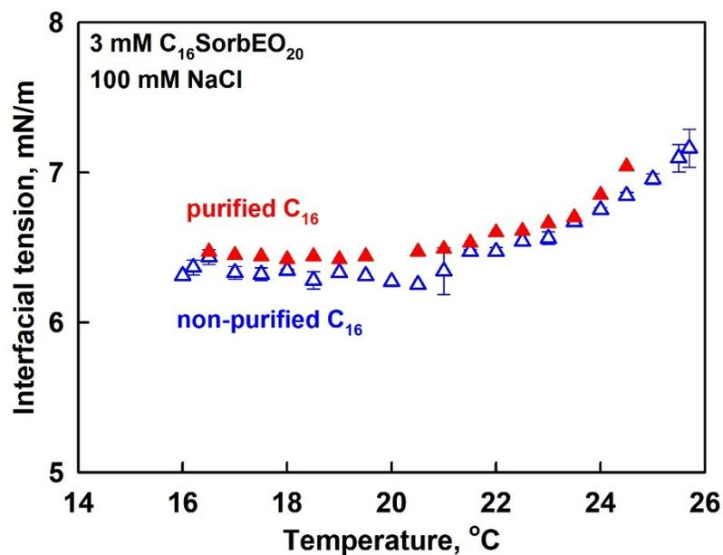
**Figure S3.** Interfacial tension as a function of temperature for purified (full red symbols) and non-purified (empty blue symbols) hexadecane drop immersed in aqueous solution containing 3 mM C<sub>16</sub>SorbEO<sub>20</sub> and 100 mM NaCl. Note that these commercial surfactants are multicomponent mixtures and the changes in the interfacial tension include possible variations in the chemical composition of the surfactant adsorption layer.
