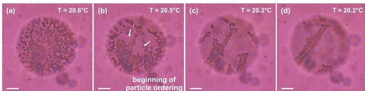
**Figure S5.** Evolution observed upon cooling with  $0.1^{\circ}\text{C}/\text{min}$  of non-purified hexadecane drop, decorated with  $1\ \mu\text{m}$  chloromethyl latex particles and immersed in solution of  $3\ \text{mM}$  surfactant  $\text{C}_{16}\text{SorbEO}_{20}$  and  $100\ \text{mM}$   $\text{NaCl}$ . Scale bars =  $10\ \mu\text{m}$ .
