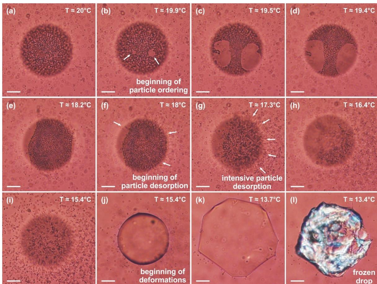
**Figure S4.** Evolution observed upon cooling with  $0.1^{\circ}\text{C}/\text{min}$  of purified hexadecane drop, decorated with  $1\ \mu\text{m}$  chloromethyl latex particles and dispersed in solution of  $3\ \text{mM}$  surfactant  $\text{C}_{16}\text{SorbEO}_{20}$  and  $100\ \text{mM}$   $\text{NaCl}$ . Scale bars =  $20\ \mu\text{m}$ .
